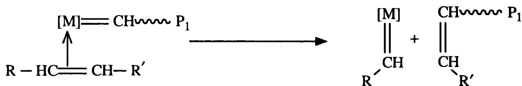
Figure 1.26: Chain transfer between acyclic olefins and the polymer chains.
