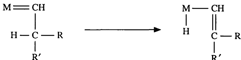
Figure 1.23: Termination of metathesis by \beta -hydrogen abstraction.
