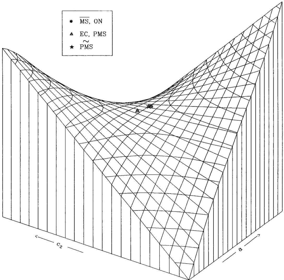
**Figure 7.3**  $a_e^{(3)}$  as a function of the couplant,  $a$ , and the second  $\beta$ -function coefficient,  $c_2$ , with  $2.3 \times 10^{-3} \leq a \leq 2.34 \times 10^{-3}$  and  $-50 \leq c_2 \leq 50$ . The values predicted by PMS, EC,  $\overline{\text{MS}}$ , ON and  $\widetilde{\text{PMS}}$  are indicated. The minimum value of  $a_e^{(3)}$  is  $1.159\ 645\ 97 \times 10^{-3}$  and the maximum value is  $1.159\ 657\ 96 \times 10^{-3}$ .
