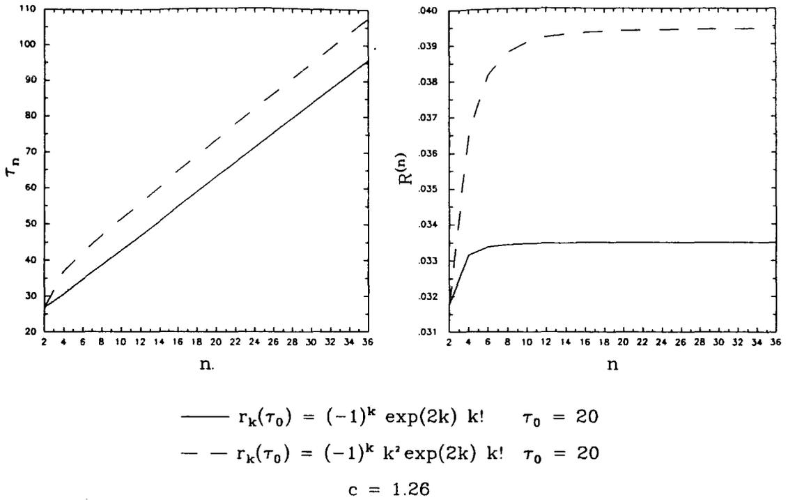
**Figure 4.10** The  $\widetilde{\text{PMS}}$  renormalization point,  $\bar{\tau}_n$ , and  $R^{(n)}(\widetilde{\text{PMS}})$  are shown for  $n = 2, \dots, 36$ , for two different functions,  $f(n)$ , in  $r_n(\tau_0)$  for  $c = 1.26$ . Again  $R^{(n)}$  converges rapidly to a value equal to the truncated Borel sum.  $\bar{\tau}_n$  appears to grow linearly with  $n$ , with slope converging to  $e^2\chi_0$ .
