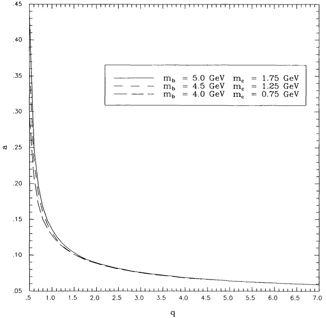
**Figure 6.4** The couplant,  $a$ , as a function of momentum,  $q$ , for three combinations of the mass of the charm and bottom quarks, with  $\tilde{\Lambda}_{\overline{\text{MS}}}^{(5)} = 0.2 \text{ GeV}$ , as this  $\tilde{\Lambda}_{\overline{\text{MS}}}$  yields the central value of the Marshall fit for  $\tilde{R}_{e^+e^-}^{(3)}$  at  $s = 1000 \text{ GeV}^2$ .
