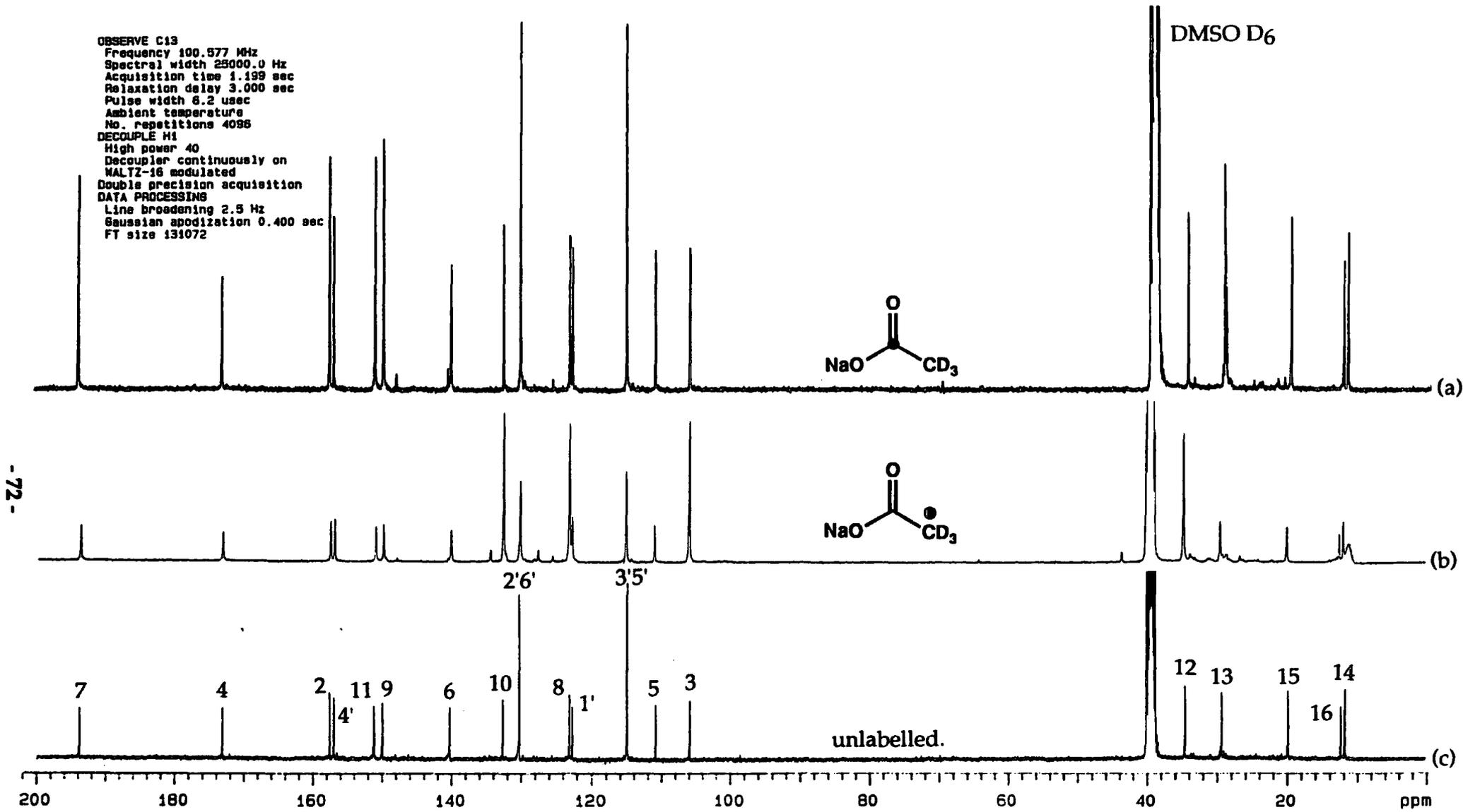
Fig. 2.514.  $^{13}\text{C}$  nmr spectra of tenellin (1) obtained from *B. bassiana* cultures (a) supplemented with sodium  $[1\text{-}^{13}\text{C}, 2\text{-}^2\text{H}_3]$ -acetate, (b) supplemented with sodium  $[2\text{-}^{13}\text{C}, 2\text{-}^2\text{H}_3]$ -acetate, (c) unfermed.
