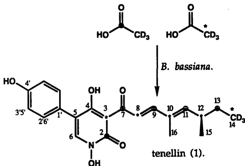
Fig. 2.512. Pattern of incorporated labels from tenellin (1) supplemented with [1-<sup>13</sup>C, 2-<sup>2</sup>H<sub>3</sub>] and [2-<sup>13</sup>C, 2-<sup>2</sup>H<sub>3</sub>] acetates.
