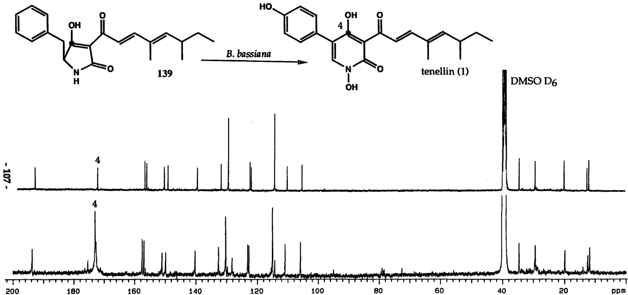
Fig. 3.221.  $^{13}\text{C}$  nmr spectra of tenellin (a) unlabelled, (b) obtained from a culture of *B. bassiana* supplemented with the acyl tetramic acid (**139**).
