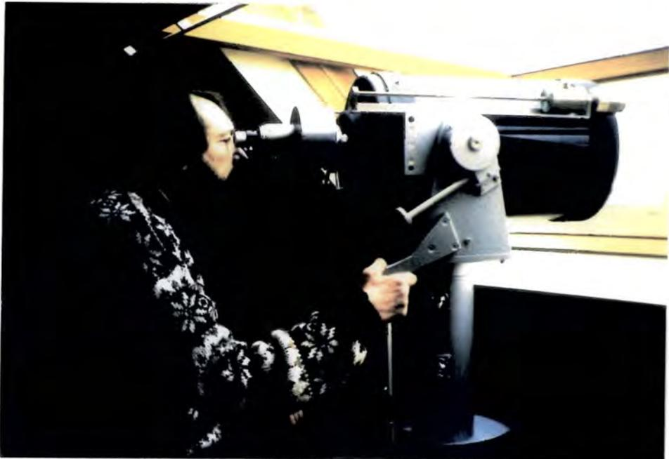
**Figure 5.** Celestron 11 astronomical telescope on special terrestrial mounting.
