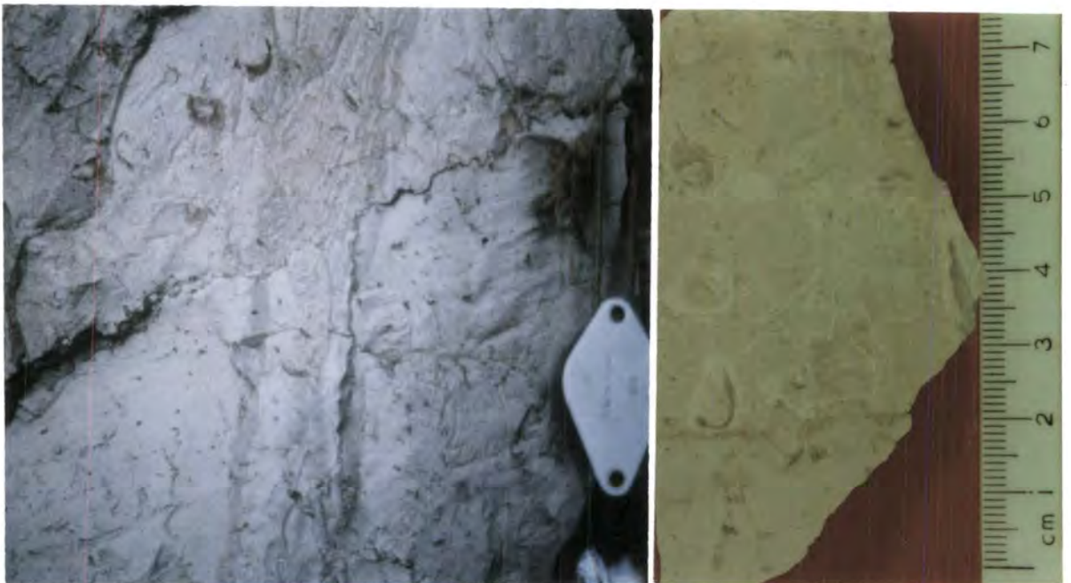
Figure 4.33B. Polished block and outcrop photo of low-energy restricted-shelf type facies overlying intertidal fenestral mudstones with Pseudotriloculina (F11 facies) within BsAi, Balcon des Ecouges, northern Vercors. The restricted lagoonal facies are characterized by small rudists up to 20mm in size and 10-20mm irregular, asymmetric oncolites nucleated on to bioclasts. The stylotized boundary between the F11 and F10 facies is the base of a 2m shallowing-up cycle (see also Figs 6.15 & 6.16).
