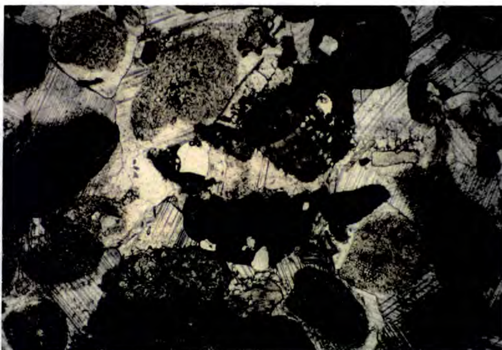
Figure 6.42. Photomicrograph of the 'Lumachelle' limestone. This grainstone contains a low diversity fauna of bryozoans and crinoids with glauconitic grains. These sands were deposited within a sand-wave complex on top of the Urgonian limestones. Field of view approximately 4mm.
