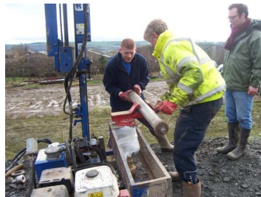
Figure 7.16 – Recovering the core of the borehole.
