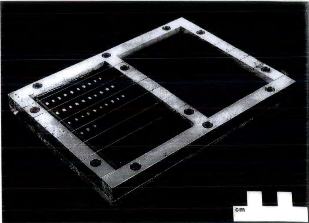
Figure 6. Mould constructed after Bedford (1983) showing otoliths aligned on black-pigmented polyester resin.
