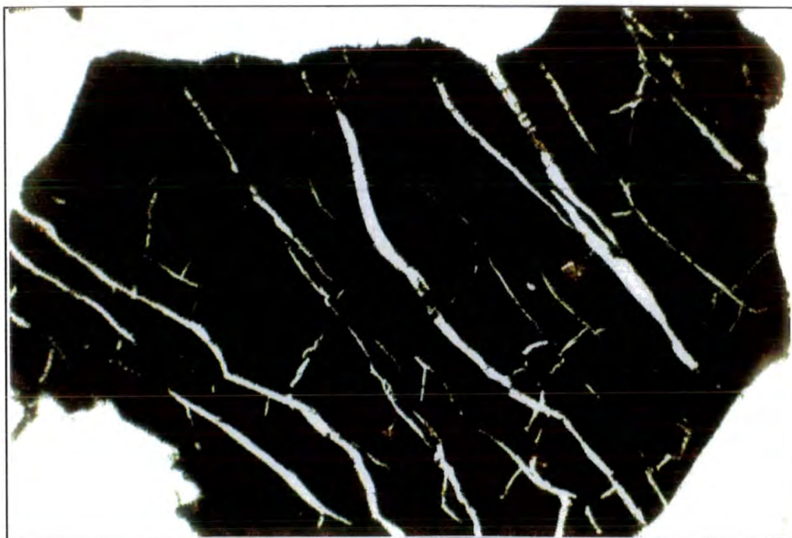
Plate (2.6) Magnetite rim in spinel. Note expansion cracks in spinel filled with serpentine. Plain polarized light, field of view 1.3 mm.
