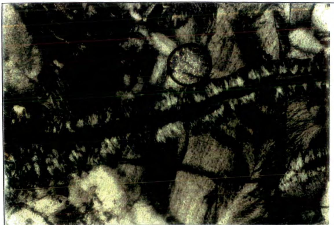
Plate (2.8) Fracture filling vein with walls of cross-fibre serpentine and centre of featureless serpentine. Crossed nicols, field of view 0.6 mm.
