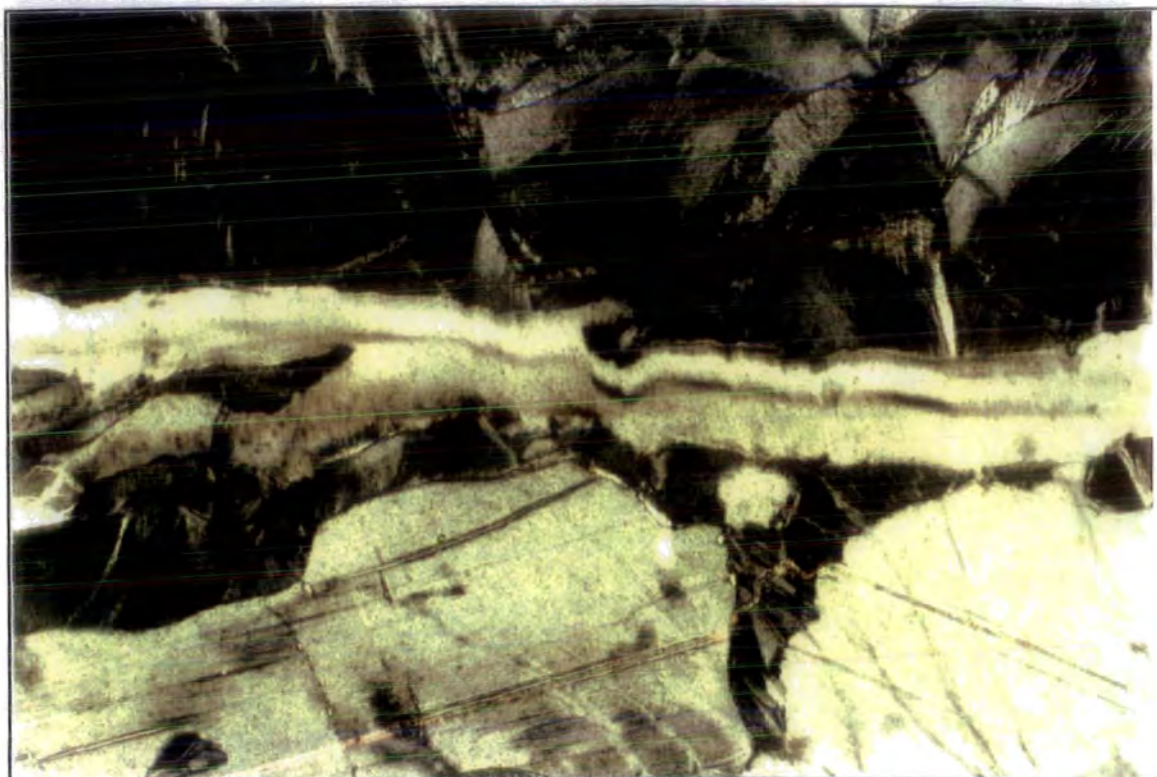
Plate (2.7) Fracture filling vein of featureless serpentine. Crossed nicols, field of view 0.6 mm.
