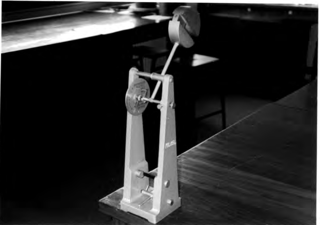
Figure 4.8 HOUNSFIELD IMPACT TESTING MACHINE
