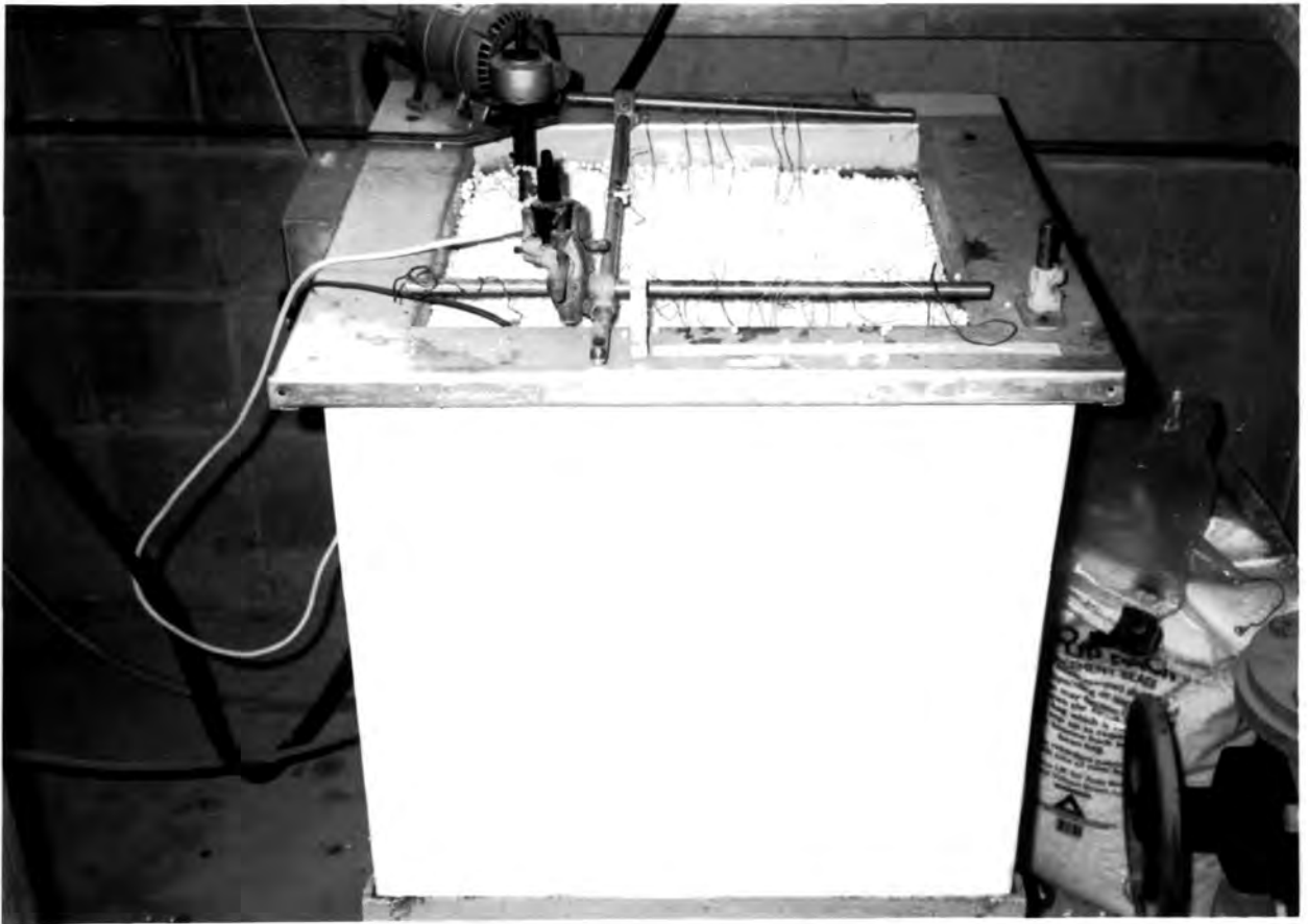
Figure 4.3 CONSTANT TEMPERATURE WATER BATH
