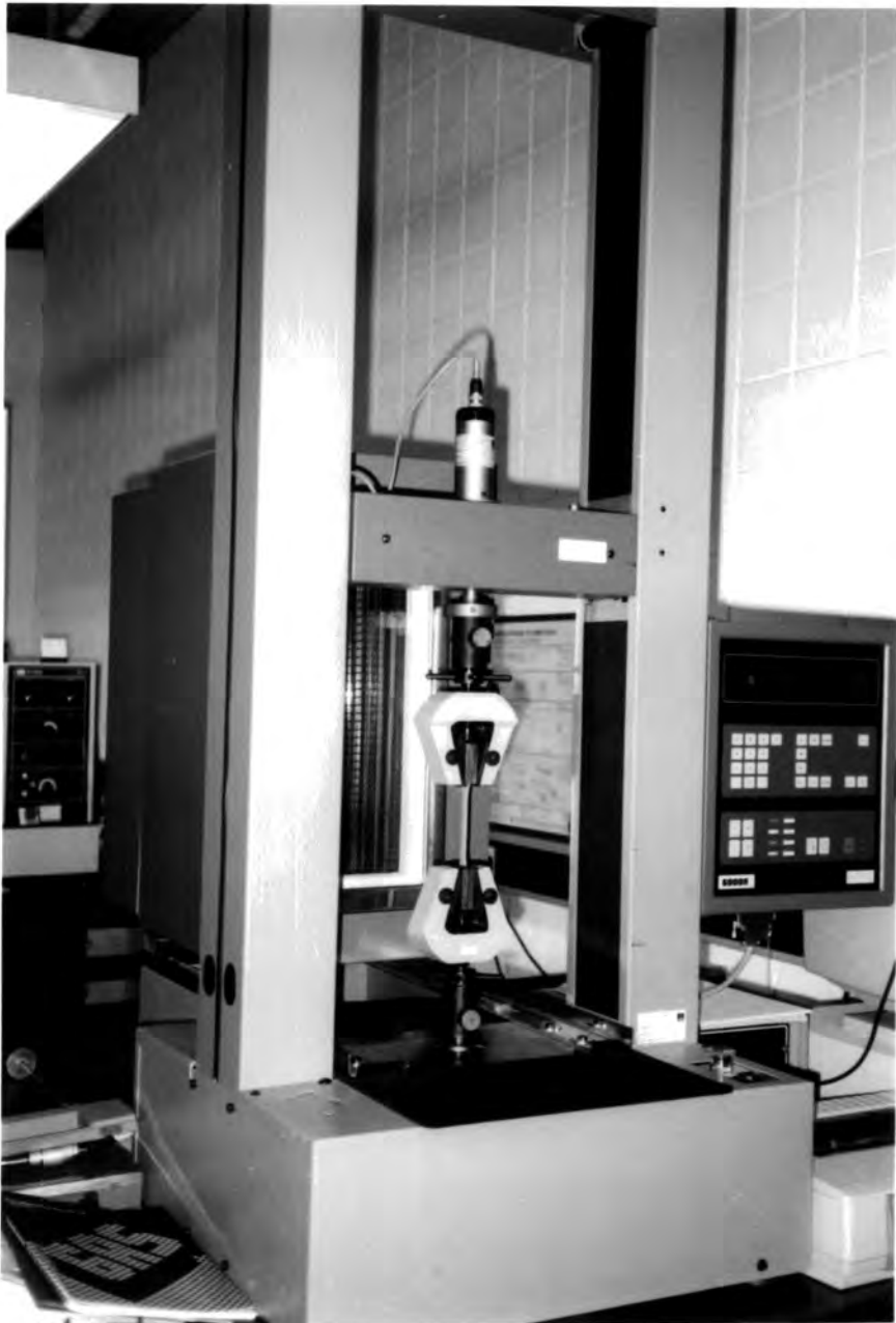
Figure 4.4 LLOYD INSTRUMENTS 30 kN BENCH MACHINE (set up for Tensile Tests)
