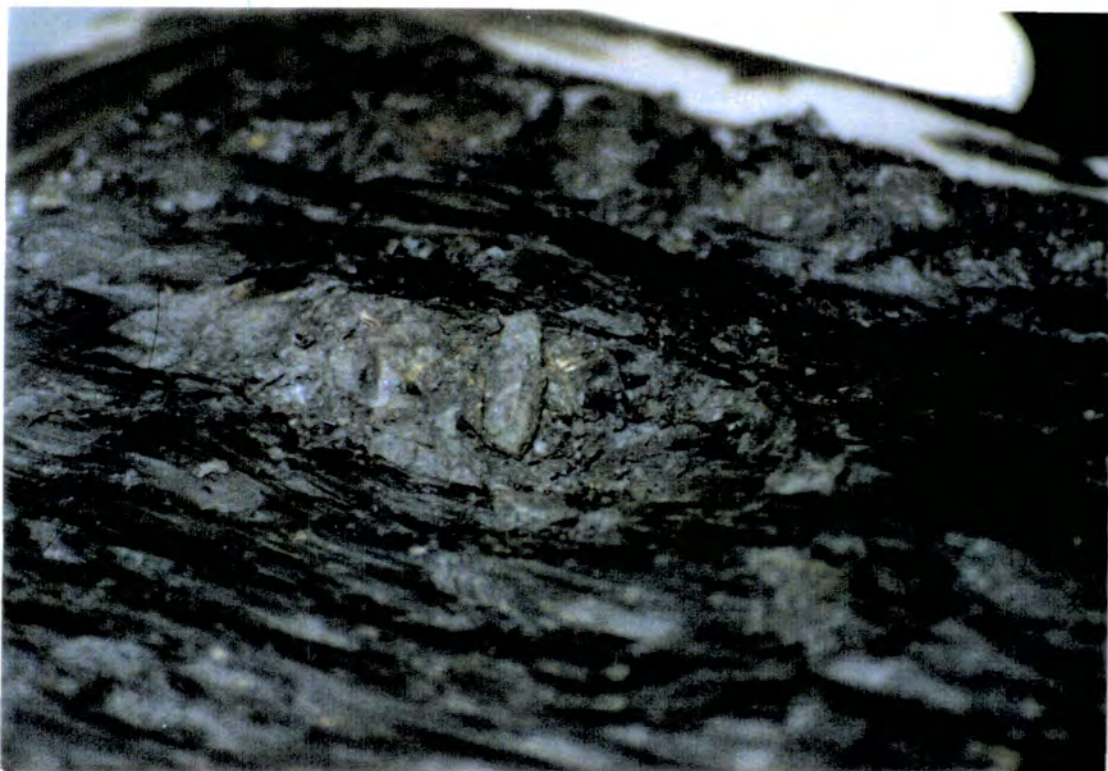
Plate 6.3: Interruption of shear plane by large clast in shear box test (undisturbed sample, Gale Common 5 year weathered shale)
