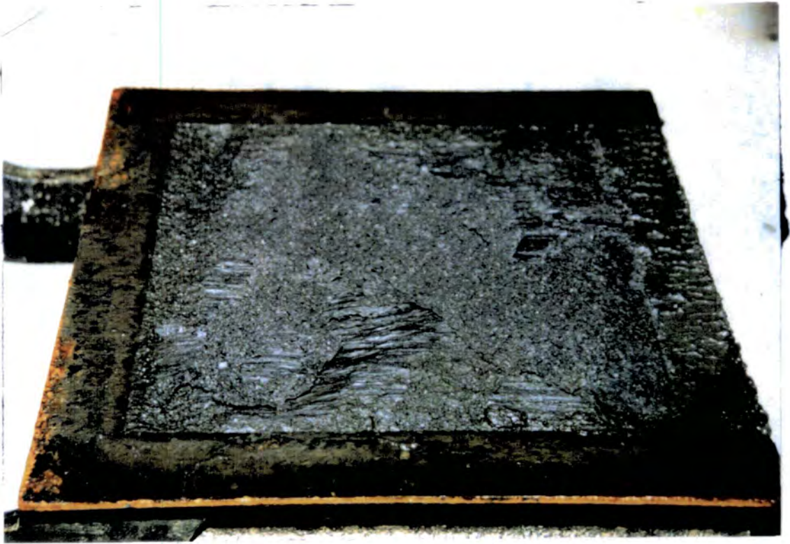
Plate 6.5: Shear plane from large shear box test (fresh Coal Measures shale passing 2mm sieve).
