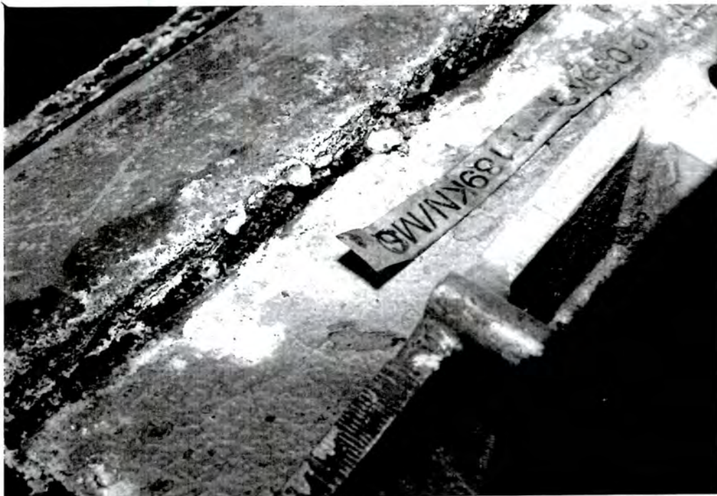
Plate 6.11: Close up of crystalline growth shown in Plate 6.10.
