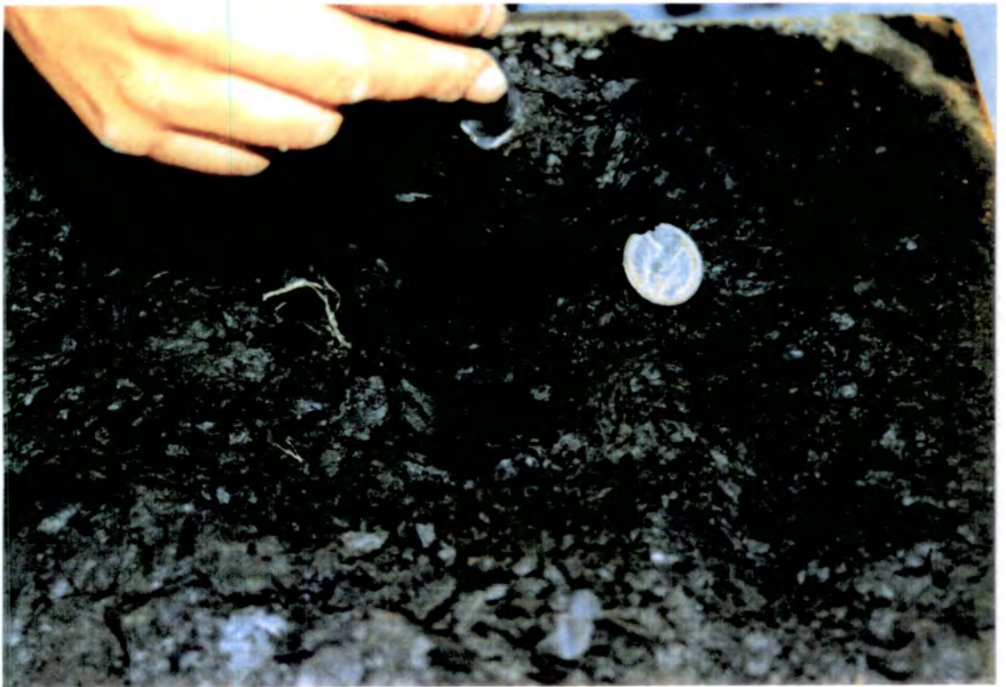
Plate 6.8: Close up of shear plane from Plate 6.7.
