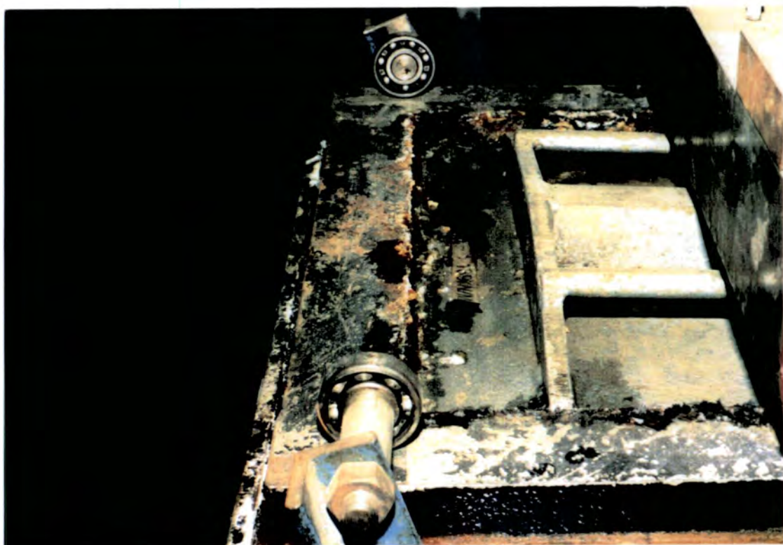
Plate 6.10: Crystalline growths around box lid observed during large shear box test (Gale Common 5 year weathered shale).
