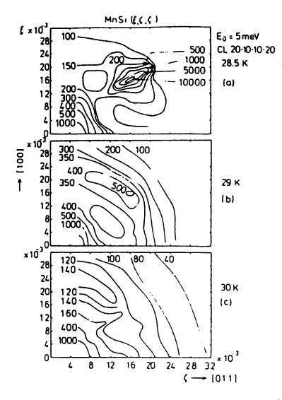
Figure 8.1 Contour maps of equal intensity of critical scattering of MnSi around a satellite point measured with  $E_i=5$ meV with  $\hbar\omega=0$  at three different temperatures. (After Ishikawa *et al.* (1982)).
