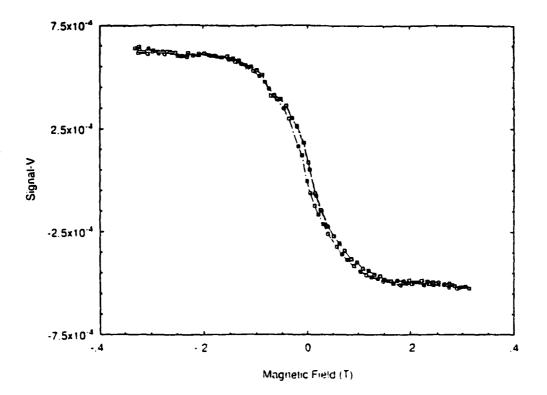
Figure A4.4 BeCu cell residual recorded at room temperature. The lockin amplifier was 'phased' when the cell contained a nickel sample.
