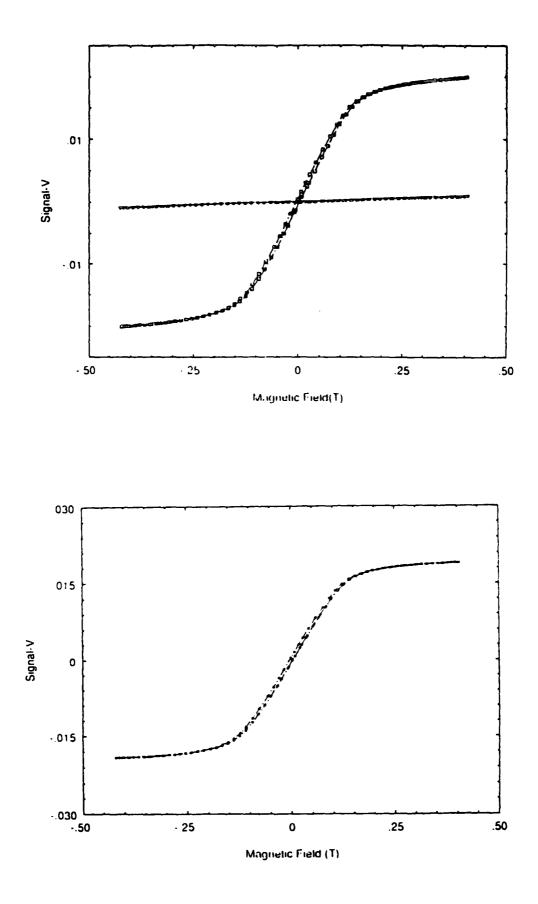
Figure A4.7 (a) The signal obtained from 0.0737g of nickel in the BeCu pressure cell (unpressurised) at 80K together with the cell residual at that temperature. (b) The corrected signal from 0.0737g of nickel with the cell residual subtracted.
