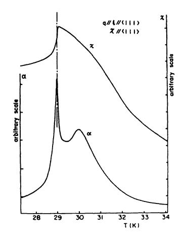
Figure 8.5 Simultaneous measurements of ultrasonic attenuation and static susceptibility of MnSi. Note the temperature where the sharp peak of attenuation agrees with the divergence of the temperature derivative of the static susceptibility. (After Kusaka *et al.* (1976)).
