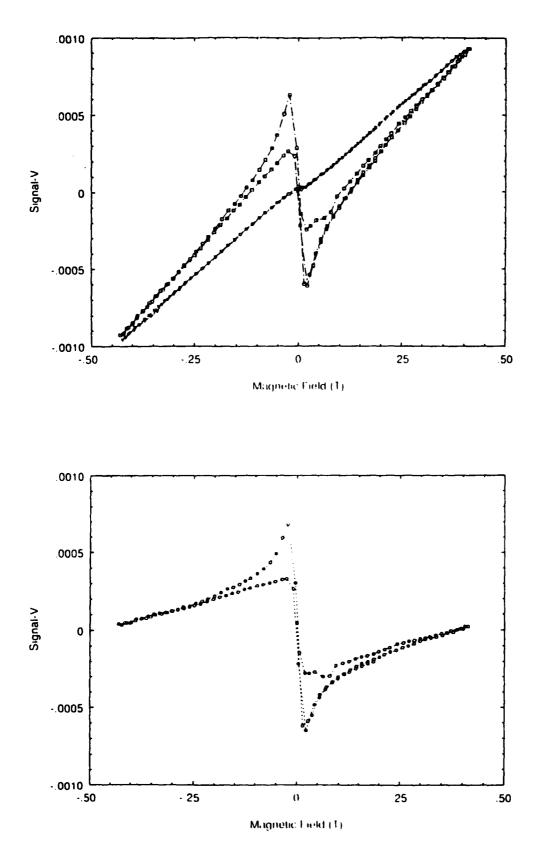
Figure A4.9 (a) The signal obtained from 0.121g of 'YBCO' in the BeCu cell at 80K (squares), where the cell had been pressurised to 1kbar at room temperature before cooling, together with the unpressurised BeCu cell residual (triangles), at that temperature. (b) The corrected signal from the 'YBCO' at 80K with the unpressurised BeCu cell residual subtracted.
