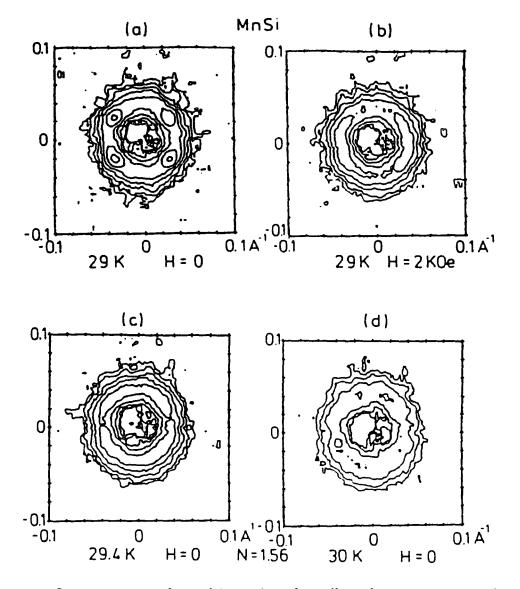
Figure 8.3 Contour maps of equal intensity of small angle neutron scattering on MnSi in the (110) reciprocal lattice plane of MnSi. Lines are plotted at intervals of 1/N of intensity with N=1.56. (a) 29K, <u>H</u>=0; (b) 29K, <u>H</u>=2kOe; (c) 29.4K, <u>H</u>=0; (d) 30K, <u>H</u>=0. (After Ishikawa *et al.* (1984)).
