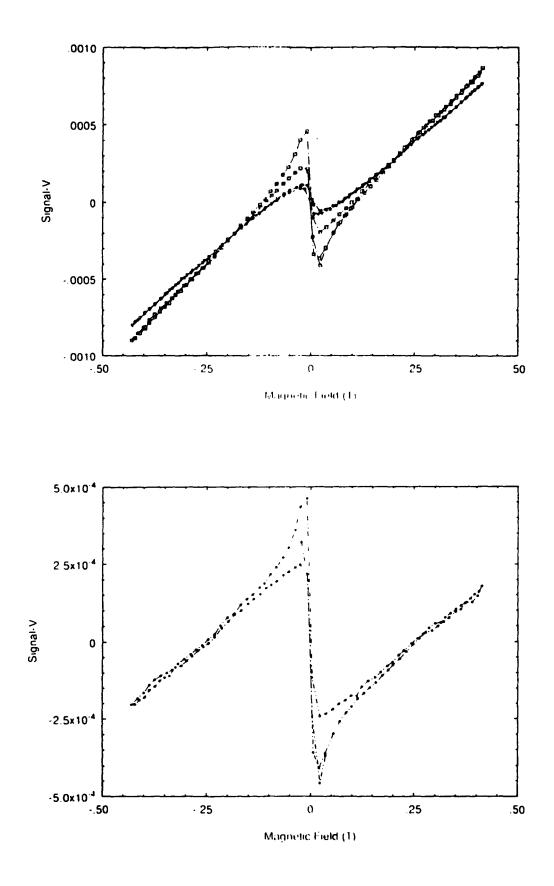
Figure A4.14 (a) The signal obtained from 0.121g of 'YBCO' in the BeCu cell at 85K (squares), where the cell had been pressurised to 1kbar at room temperature before cooling, together with the signal obtained from 0.121g of 'YBCO' under identical conditions apart from at 95K (triangles). (b) The corrected signal from the 'YBCO' at 85K with signal obtained at 95K subtracted.
