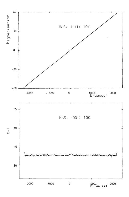
Figure 5.14 (a) The magnetisation of MnSi with a magnetic field applied parallel to the < 111 > direction at a temperature of 10K; (b) the inverse magnetic susceptibility of MnSi at 10K derived from the magnetisation data. The solid line is an average through the data points for a given field value and direction and is a measure of the experimental incertainty.
