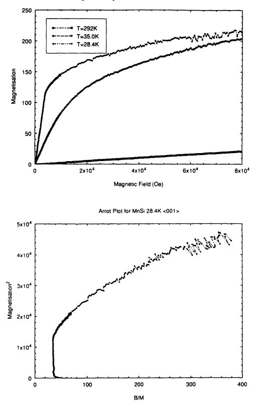
Figure 5.17 (a) High field magnetisation measurements on MnSi with magnetic field applied parallel to the < 001 > direction for temperatures 292K (squares), 35.0K (triangles) and 28.4K (circles); (b) the 'Arrot Plot' for MnSi at 28.4K derived from the high field magnetisation data with magnetic field applied parallel to the < 001 > direction.
