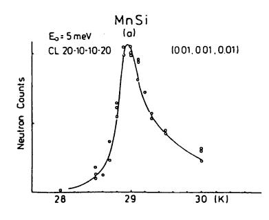
Figure 8.2 Temperature variation of peak intensities of MnSi at  $\underline{q} = (0.01, 0.01, 0.01)^{2\pi}$  measured with  $E_i = 5$  meV. (After Ishikawa (1982)).
