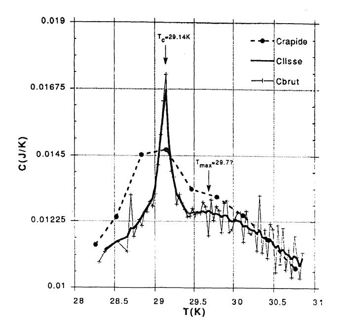
Figure 8.7 (b) Variation of the heat capacity of MnSi for increasing temperature close to  $T_N$ . (After Bernhoeft *et al.* (1992)).
