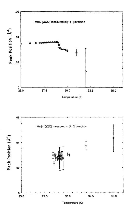
Figure 8.16 Peak position of the Gaussian fit to the residual corrected critical scattering of MnSi close to  $T_N$ . (a)  $\underline{q}$  scan in the [111] direction; (b)  $\underline{q}$  scan in the [110] direction.
