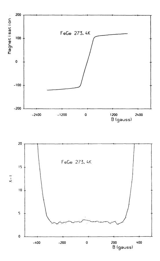
Figure 6.5 (a) The magnetisation of FeGe with magnetic field applied parallel to the < 001 > direction at a temperature of 273.4K; (b) the inverse magnetic susceptibility of FeGe with field applied parallel to the < 100 > at a temperature of 273.4K derived from the magnetisation data. In both cases, the solid line is an average through the data points for a given field value and is a measure of the experimental uncertainty.
