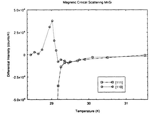
Figure 8.20 Differential intensity of the peak height of the Gaussian fit to the residual corrected critical scattering of MnSi close to  $T_N$ . (a)  $\underline{q}$  scan along [111] direction; (b)  $\underline{q}$  scan along [110] direction; (c) and (d) combined on the same figure.
