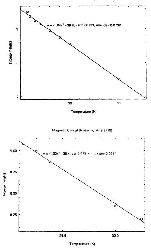
Figure 8.19 Natural log of the peak height of the Gaussian fit to the residual corrected critical scattering of MnSi against temperature together with least squares linear fit. (a)  $\underline{q}$  scan along [111] direction; (b)  $\underline{q}$  scan along [110] direction.
