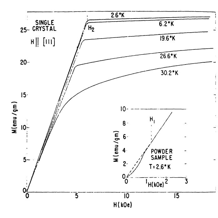
Figure 2.1 Magnetisation of MnSi as a function of applied magnetic field. (After Levinson *et al.* (1972)).
