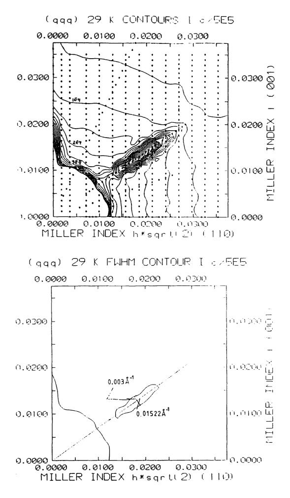
Figure 8.11 (a) equal intensity contours of a compilation of scans of the (111) magnetic Bragg reflection of MnSi at 29K with scans taken along the marked lines. This was used to calculate (b) the half width contour of the (111) magnetic Bragg reflection at 29K.
