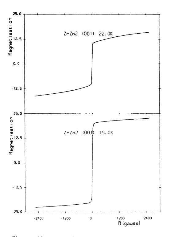
Figure 4.2 Magnetisation of  $ZrZn_2$  as a function of applied magnetic field. Measurements were taken for decreasing temperature with field steps of 50Oe. The solid line is an average through the data points for a particular field. (a) 30.0K; (b) 27.0K; (c) 26.0K; (d) 25.0K; (e) 24.5K; (f) 24.2K; (g) 23.9K; (h) 23.6K; (i) 23.3K; (j) 22.0K; (k) 15.0K.
