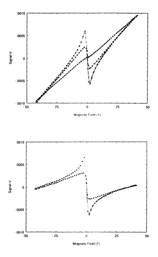
Figure A4.10 (a) The signal obtained from 0.121g of 'YBCO' in the BeCu cell at 80K (squares), where the cell had been pressurised to 2kbar at room temperature before cooling, together with the unpressurised BeCu cell residual (triangles), at that temperature. (b) The corrected signal from the 'YBCO' at 80K with the unpressurised BeCu cell residual subtracted.
