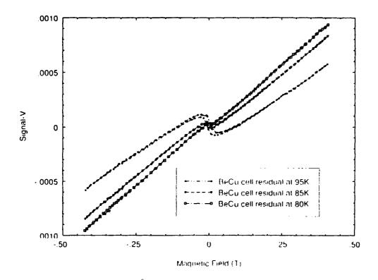
Figure A4.6 The signal obtained from the BeCu cell at 95K (circles), 85K (triangles) and 80K (squares).
