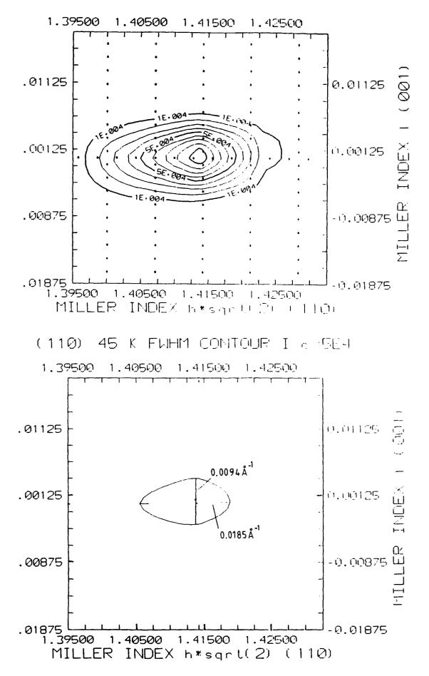
Figure 8.10 (a) Equal intensity contours of a compilation of scans of the (110) crystal Bragg reflection of MnSi at 45K with scans taken along the marked lines. This was used to calculate (b) the half width contour of the (110) crystal Bragg reflection at 45K.
