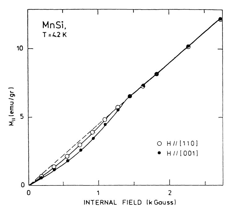
Figure 2.3 Magnetisation of MnSi as a function of applied magnetic field with magnetic field applied along particular crystallographic directions. (After Hansen (1977)).
