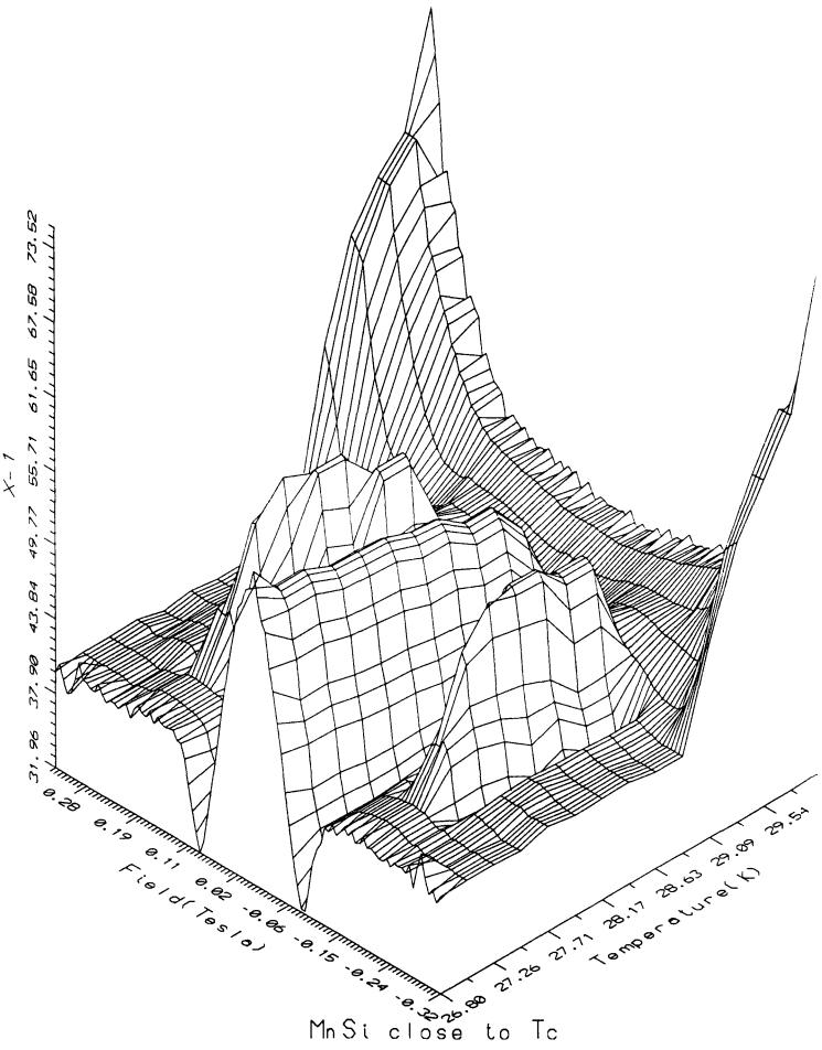
Figure 5.21 The inverse magnetic susceptibility of MnSi as a function of both magnetic field and temperature close to the transition temperature, derived from the magnetisation data with field applied parallel to the < 111 >.
