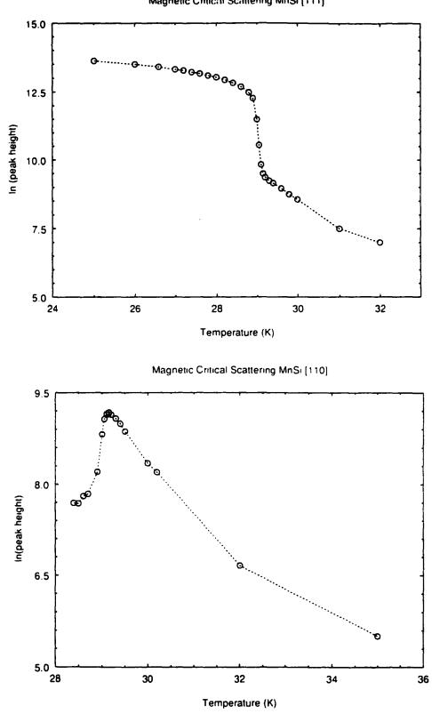
Figure 8.17 Natural log of the peak height of the Gaussian fit to the residual corrected critical scattering of MnSi close to  $T_N$ . (a) q scan in the [111] direction; (b) q scan in the [110] direction.
