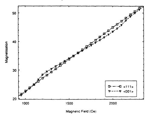
Figure 5.5 The magnetisation of MnSi with magnetic field applied parallel to the < 001 > (triangles) and < 111 > (squares) direction at a temperature of 28.6K i.e. in the temperature and field regime where 'Phase A' is observed in the < 001 > direction.
