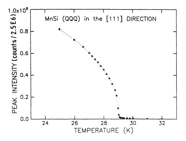
Figure 8.14 Peak height or intensity of the Gaussian fits to the residual corrected critical scattering of MnSi close to  $T_N$ . (a)  $\underline{q}$  scan in the [111] direction; (b)  $\underline{q}$  scan in the [110] direction; (c)  $\underline{q}$  scan in the [111] direction (expanded scale).
