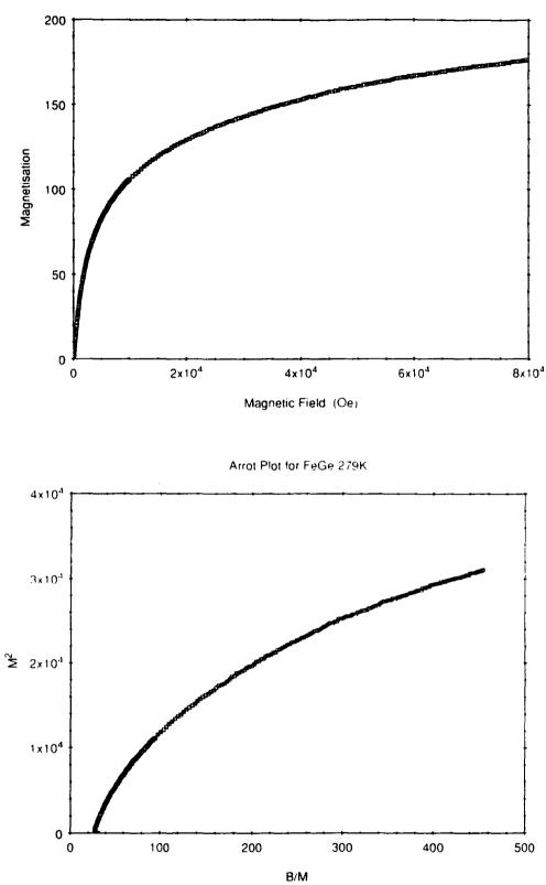
Figure 6.16 (a) high field magnetisation measurements on FeGe with magnetic field applied parallel to the < 100 > direction at 279K; (b) 'Arrot Plot' for FeGe at 279K derived from the high field magnetisation data.
