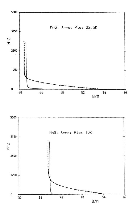
Figure 5.18 'Arrot Plots' for MnSi derived from the magnetisation data with magnetic field applied parallel to the < 111 > (points)/< 001 > (triangles). (a) 30.0K; (b) 29.1K; (c) 28.2K; (d) 22.5K; (e) 10.0K.
