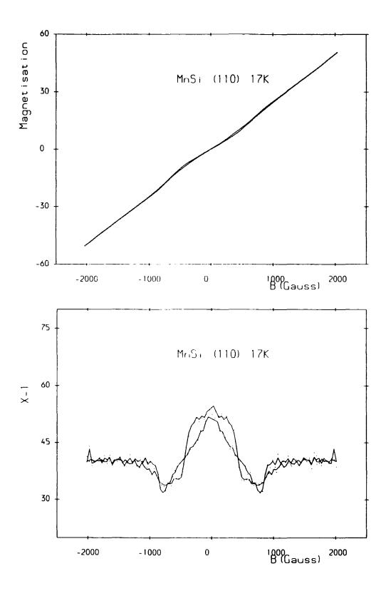
Figure 5.13 (a) The magnetisation of MnSi with a magnetic field applied parallel to the < 110 > direction at a temperature of 17K; (b) the inverse magnetic susceptibility of MnSi at 17K derived from the magnetisation data. The solid line is an average through the data points for a given field value and direction and is a measure of the experimental uncertainty.
