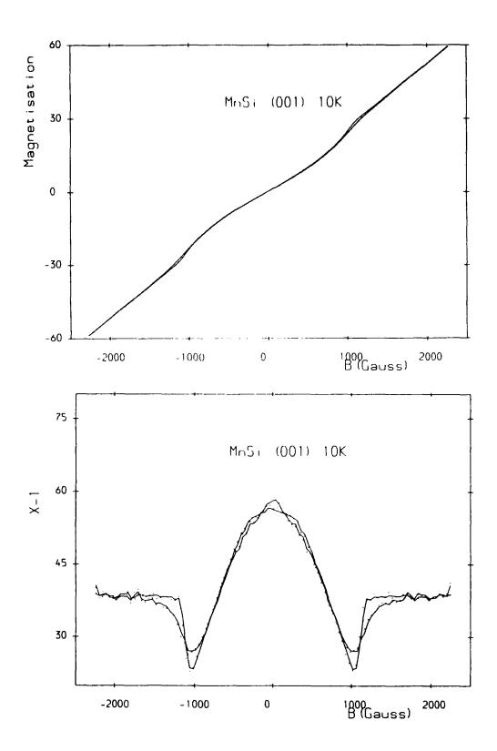
Figure 5.15 (a) The magnetisation of MnSi with a magnetic field applied parallel to the < 001 > direction at a temperature of 10K; (b) the inverse magnetic susceptibility of MnSi at 10K derived from the magnetisation data. The solid line is an average through the data points for a given field value and direction and is a measure of the experimental uncertainty.
