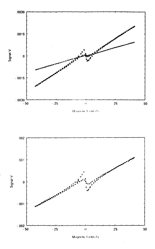
Figure A4.11 (a) The signal obtained from 0.121g of 'YBCO' in the BeCu cell at 80K (squares), where the cell had been pressurised to 4kbar at room temperature before cooling, together with the unpressurised BeCu cell residual (triangles), at that temperature. (b) The corrected signal from the 'YBCO' at 80K with the unpressurised BeCu cell residual subtracted.
