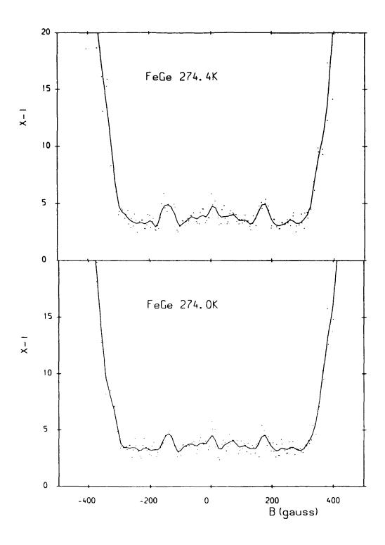
Figure 6.4 The inverse magnetic susceptibility of FeGe with field applied parallel to the < 100 >, derived from the magnetisation data. The solid line is the data (points) after being smoothed (see Appendix 2). (a) 276.8K; (b) 276.2K; (c) 275.2K; (d) 274.4K; (e) 274.0K.
