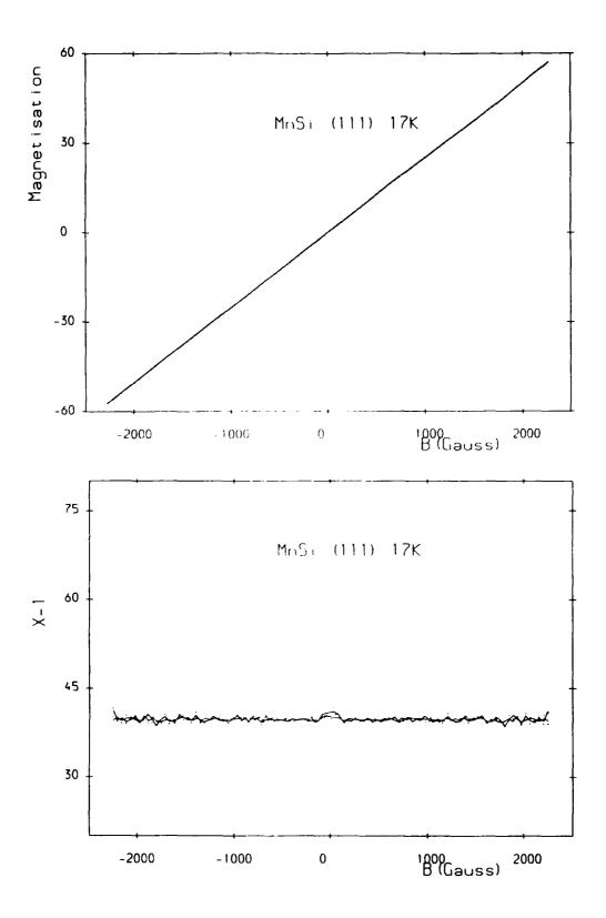
Figure 5.11 (a) The magnetisation of MnSi with magnetic field applied parallel to the < 111 > disrection at a temperature of 17K; (b) the inverse magnetic susceptibility of MnSi at 17K derived from the magnetisation data. The solid line is an average through the data points for a given field value and direction and is a measure of the experimental uncertainty.
