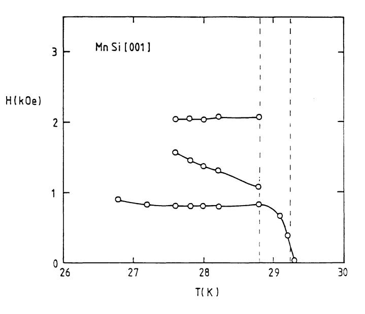
Figure 5.4 The positions of field minima of the inverse susceptibility in the < 001 > direction displayed as a function of internal field and sample temperature.
