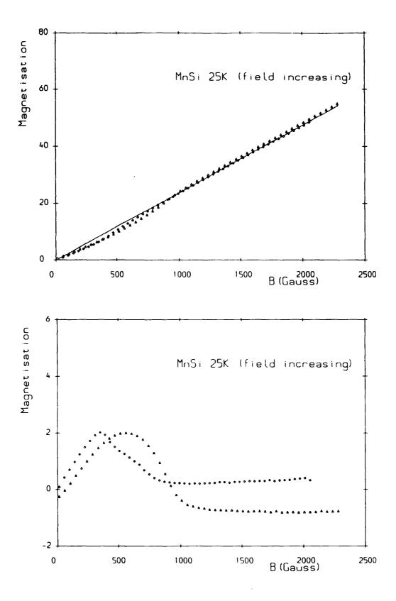
Figure 5.9 (a) The magnetisation of MnSi for an increasing magnetic field applied parallel to the < 111 > (complete line), < 001 > (triangles) and < 110 > (circles) at a temperature of 25K; (b) the subtraction of the magnetisation of MnSi (for an increasing field) with magnetic field applied parallel to the < 001 > (triangles)/< 110 > (circles) from the magnetisation with magnetic field applied parallel to the < 111 > direction.
