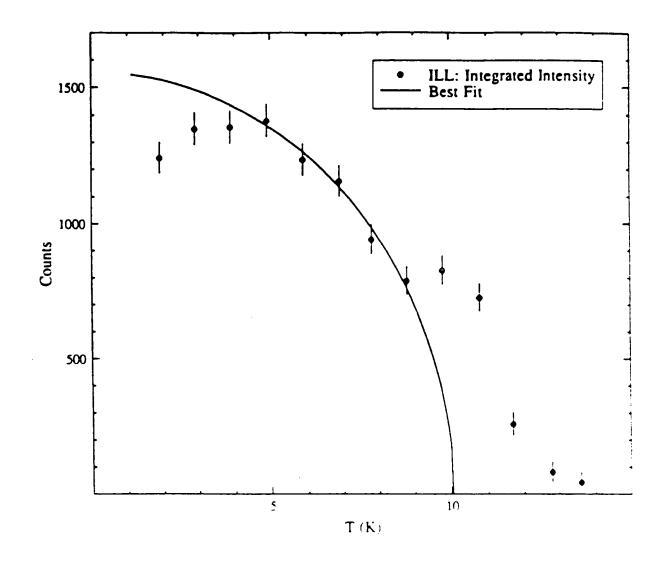
**Figure 8.8** Variation of satellite intensity with temperature for MnSi at 12kbar. The intensity was obtained by integrating the number of counts at each temperature between q=0.071Å<sup>-1</sup> and q=0.024Å<sup>-1</sup> and then subtracting the 20K background. (After Brown (1990)).
