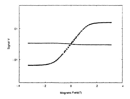
Figure A4.5 The signal obtained from 0.0737g of nickel in the BeCu cell (unpressurised) at room temperature together with the cell residual.
