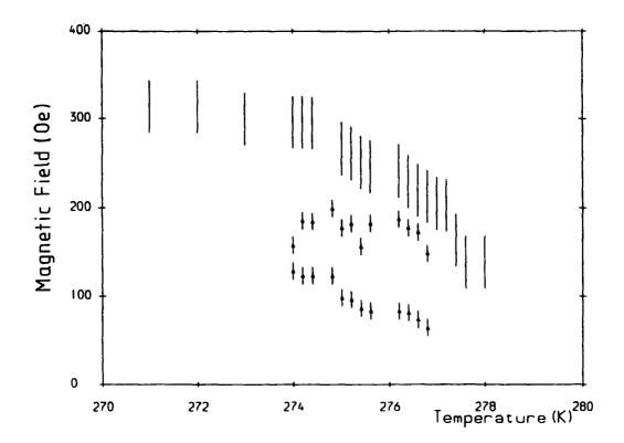
Figure 6.6 Field position of the 'knee' in the magnetisation of FeGe with field applied parallel to the < 100 > direction (points) and the field positions of the onset and conclusion of the region of increased inverse susceptibility (triangles) in an applied magnetic field close to the transition temperature.
