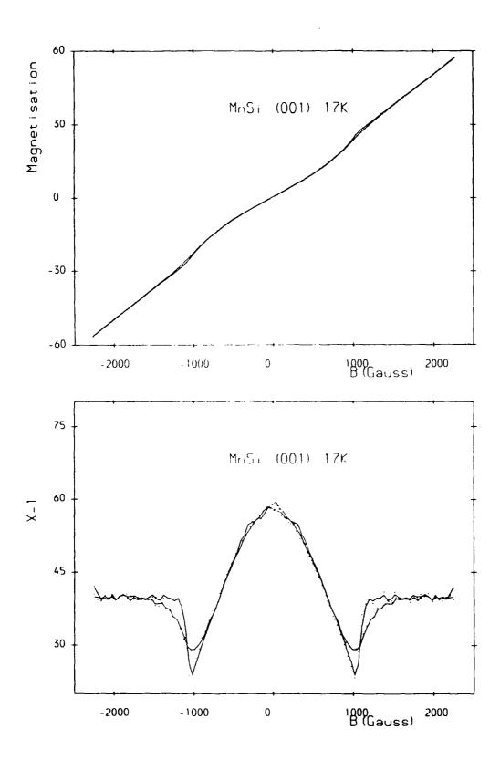
Figure 5.12 (a) The magnetisation of MnSi with a magnetic field applied parallel to the < 001 > direction at a temperature of 17K; (b) the inverse magnetic susceptibility of MnSi at 17K derived from the magnetisation data. The solid line is an average through the data points for a given field value and direction and is a measure of the experimental uncertainty.
