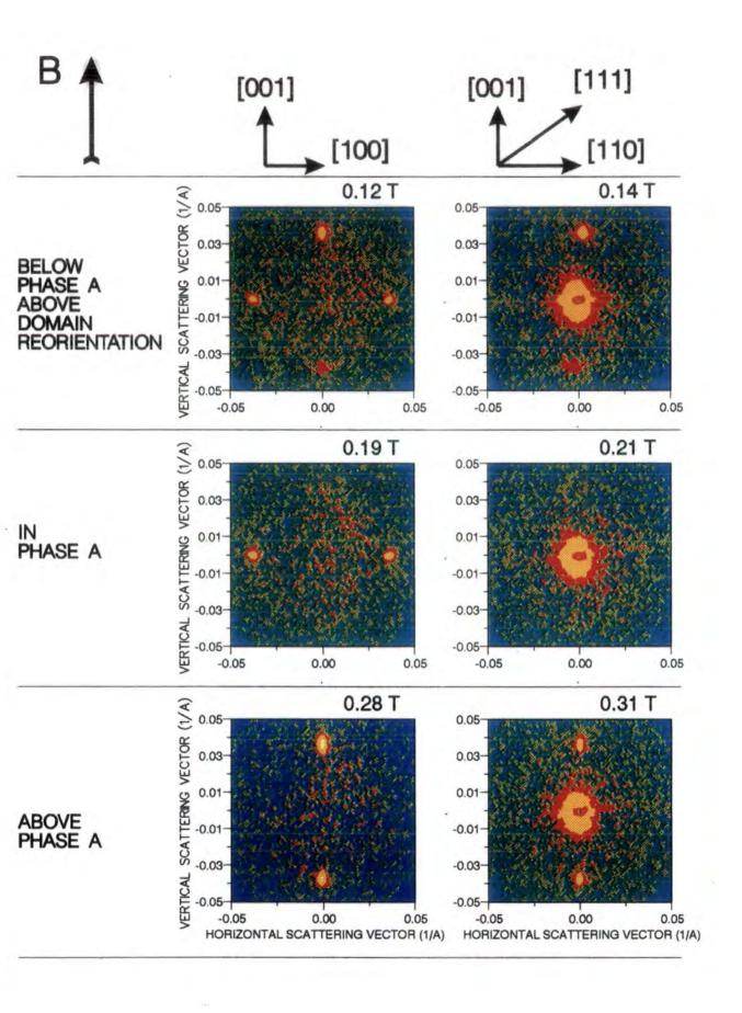
Figure 7.12 Equal intensity contours, SANS data (log scale) observed at the start of 'Phase A' in a magnetic field of 0.12T. The crystal is orientated such that the [001] is vertical and [100] horizontal in the scattering plane.
