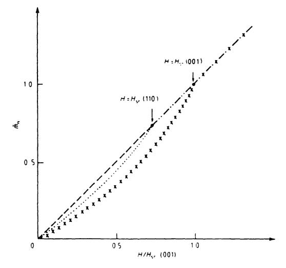
Figure 2.7 The magnetisation in the spin density wave phase versus magnetic field at a temperature well below  $T_N$  for H  $\parallel < 001 >$  (broken curve), H  $\parallel < 110 >$  (dotted curve) and H  $\parallel < 001 >$  (crosses). (After Plumer *et al.* (1981)).
