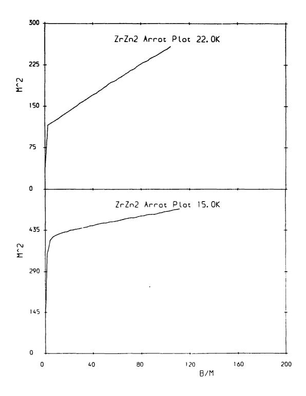
Figure 4.4 Arrot Plots for  $ZrZn_2$  derived from the data of fig. 4.2. A solid line connects the raw data points. (a) 25.0K; (b) 24.5K; (c) 24.2K; (d) 23.9K; (e) 23.6K; (f) 23.3K; (g) 22.0K; (h) 15.0K.
