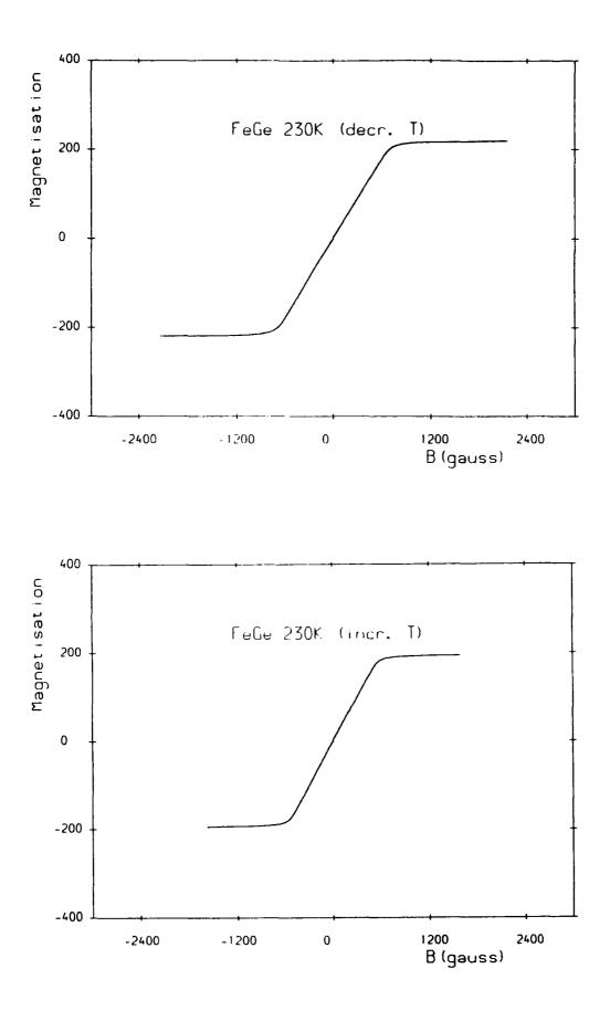
Figure 6.9 (a) The magnetisation of FeGe with magnetic field applied parallel to the < 100 > direction at 230K when lowering the temperature; (b) The magnetisation of FeGe with magnetic field applied parallel to the < 100 > direction at 230K but for increasing the temperature (from 180K).
