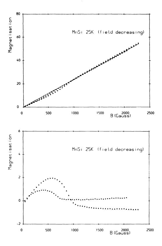
Figure 5.10 (a) The magnetisation of MnSi for a decreasing magnetic field applied parallel to the < 111 > (complete line), < 001 > (triangles) and < 110 > (circles) at a temperature of 25K; (b) the subtraction of the magnetisation of MnSi (for an decreasing field) with amgnetic field applied parallel to the < 001 >(triangles)/< 110 >(circles) from the magnetisation with magnetic field applied parallel to the < 111 > direction.
