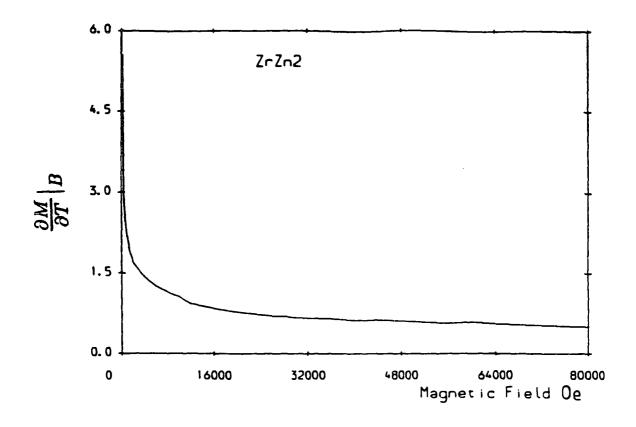
**Figure 4.8**  $\frac{\partial M}{\partial T}|_B$  vs magnetic field from the data of figure 4.7 and other similar measurements close to the transition temperature. A solid line connects the data points.
