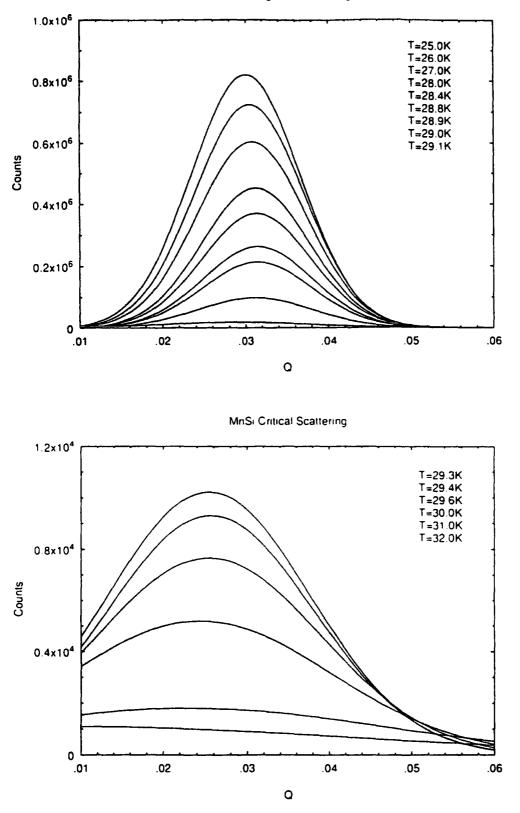
Figure 8.13 A selection of the Gaussian curves fitted to the residual corrected magnetic critical scattering from MnSi with  $\underline{q}$  scanned along the [111] direction. (a) Below the transition temperature determined by SANS (see Chapter 7); (b) above the transition temperature determined by SANS.
