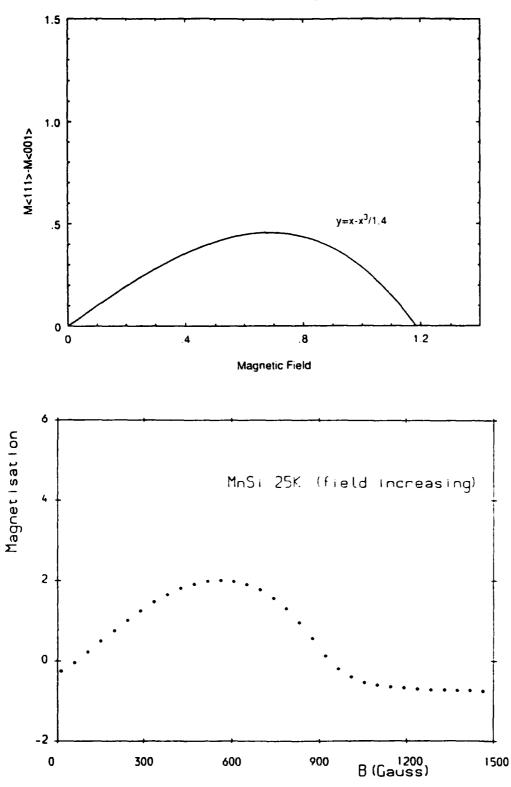
Figure 7.16 (a) Theoretical form of the difference in magnetisation measured with field parallel to the < 111 > and < 001 > directions developed from the work of Plumer *et al.* (1981); (b) experimentally determined difference in magnetisation measured with field applied parallel to the < 111 > and < 001 > directions.
