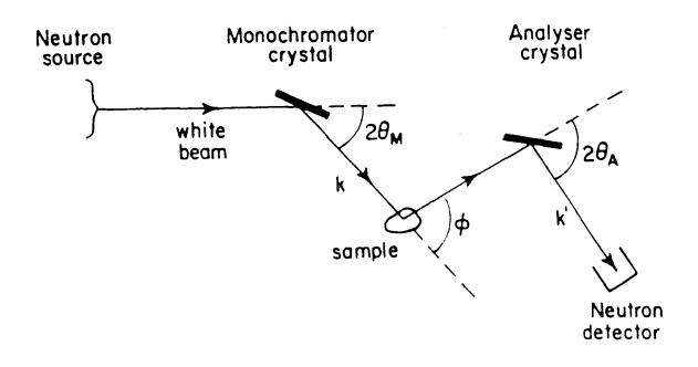
**Figure 8.9** The triple axis spectrometer. A monochromator crystal scatters just those neutrons from a white source with wavevector  $\underline{k}$ . An analyser crystal sends to the detector just those neutrons scattered through an angle  $\phi$  that have wavevector  $\underline{k}'$ .
