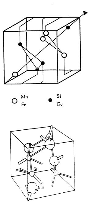
Figure 2.11 The cubic  $B_{20}$  structure of MnSi and FeGe.
