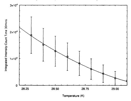
Figure 7.7 (a)Integrated intensity of the detector corresponding to the position of the top left magnetic Bragg satellite; (b) a parabolic fit to the data points below the transition temperature.
