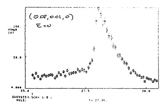
Figure 8.4 Temperature variation of peak intensities of MnSi at q=(0.2,0.2,0)  $\frac{2\pi}{a}$  and  $\hbar\omega = 0$ . (After Hayden *et al.* (1991)).
