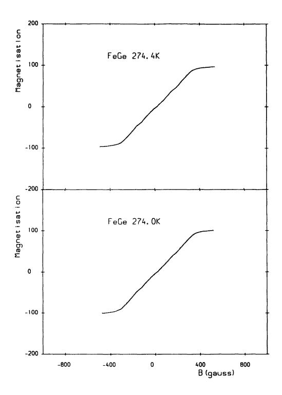
Figure 6.3 The magnetisation of FeGe with applied magnetic field parallel to the < 100 > direction. The solid line is an average through the data points for a given field value and is a measure of the experimental uncertainty. (a) 276.8K; (b) 276.2K; (c) 275.2K; (d) 274.4K; (e) 274.0K.
