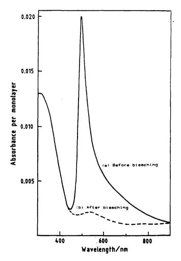
Figure 4.1 : Photochromic switching of CisHas-P3CNQ
