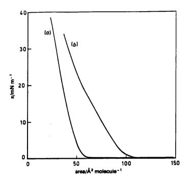
Figure 3.4 : Surface Pressure ( $\Pi$ ) vs. Surface Area Isotherms of (a)C<sub>a</sub>H<sub>17</sub>-Q3CNQ; (b) C<sub>16</sub>H<sub>33</sub>-Q3CNQ (20)
