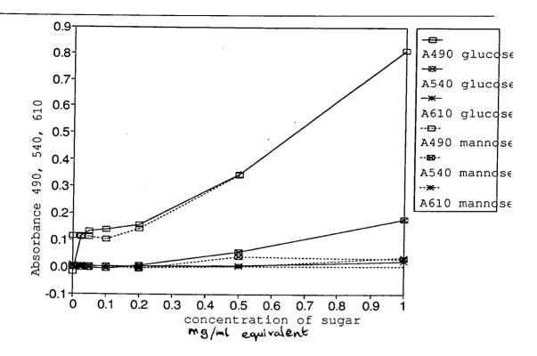
Figure 2-a Absorbance at different wavelengths of standard sugars; calibrating the modified Bernfeld amylase assay
