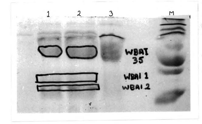
Plate 10 19% SDS-PAGE of WBAI and bands of protein detected on PVDF blot prior to sequencing
