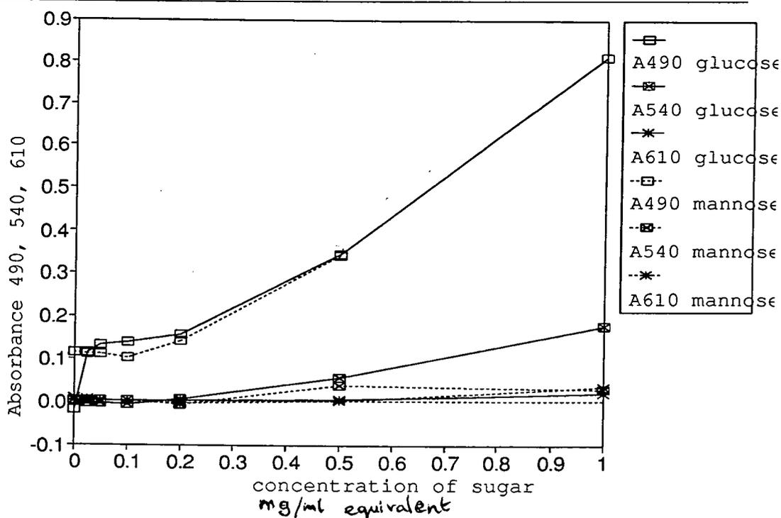
**Figure 2-a** Absorbance at different wavelengths of standard sugars; calibrating the modified Bernfeld amylose assay
