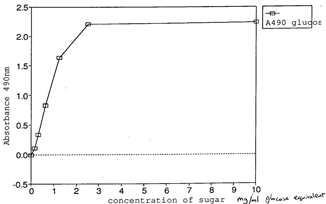
**Figure 2-b** Calibration of glucose up to 10mg/ml equivalent in the substrate solution, for amylase assay
