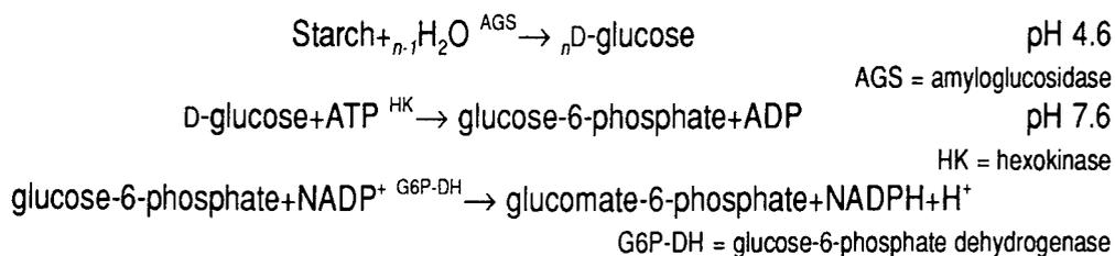
NADPH is produced stoichiometrically with respect to the release of glucose, and is measured quantitatively at 340nm.
