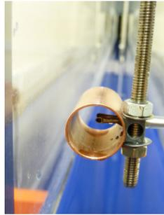
(a) Kiel-reverse probe, detail of the pressure intake and the positioning bar. Due to the pressure taps are protected by the outer cylinder, the positioning bar has little influence in the flow streams.
