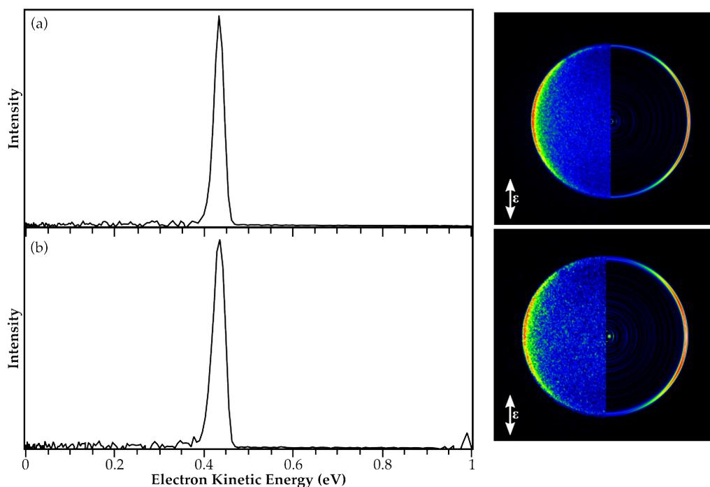
Figure 2.12: Photoelectron spectra for the detachment from iodide collected at 355 nm (3.496 eV). (a) Conventional VMI arrangement (electrodes at  $-75$  V, detector front grounded) (b) inverted imaging voltages with the detector floating at  $+75$  V and the electrodes at  $< 2$  V. Shown on the right are the raw (left half) and reconstructed (right half) photoelectron images with the laser polarisation indicated by the arrow.
