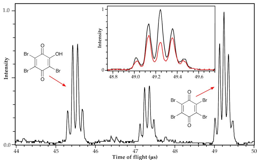
Figure 2.8: Example mass spectrum produced by electrospraying a solution of Bromanyl, whose parent anion peak is observed around  $49.2 \mu\text{s}$ , as indicated. Clear isotope patterns are observed, yielding a mass resolution  $> 200$ . The inset shows the parent anion peak (black) and the effect of irradiation of the most abundant isotope with a nanosecond laser pulse (red), showing strong isotope selective depletion.
