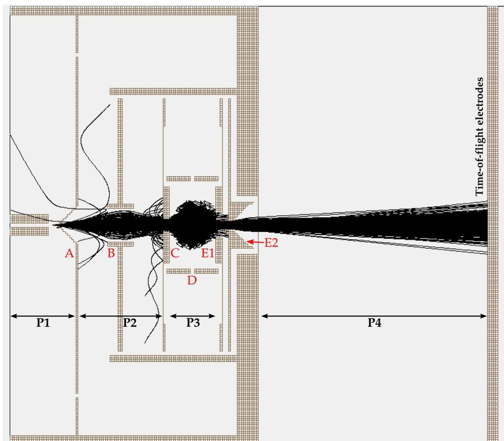
Figure 6.2: SimIon simulation of the new trap design, with parts labelled as in figure 6.1 and P1 - P4 indicating different pressure regions simulated, corresponding to 3 Torr,  $10^{-4}$  Torr,  $10^{-3}$  Torr and  $10^{-5}$  Torr, respectively. Simulated were 1800 ion trajectories ( $m/z = 200$  Da), 46% of ions are successfully trapped and ejected and impact on the time-of-flight electrodes.
