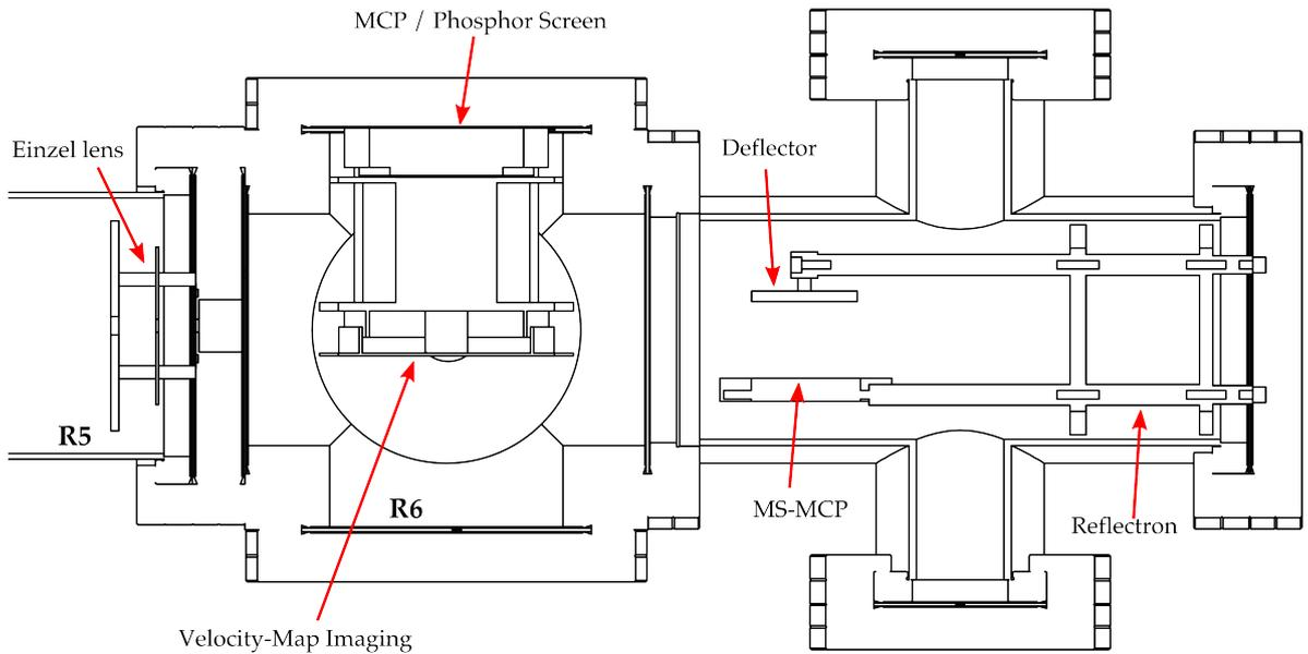
Figure 2.5: Overview of the high vacuum side of the spectrometer, contain regions 5 and 6 with the detector setup. A custom build velocity-map imaging detector is used for photoelectron imaging. The primary ion beam can be monitored by directly measuring ion current as a function of time-of-flight on the microchannel plate (MCP) detector. Alternatively, fragments produced by interaction between the laser and primary ion beam can be separated via a secondary reflectron mass spectrometer.
