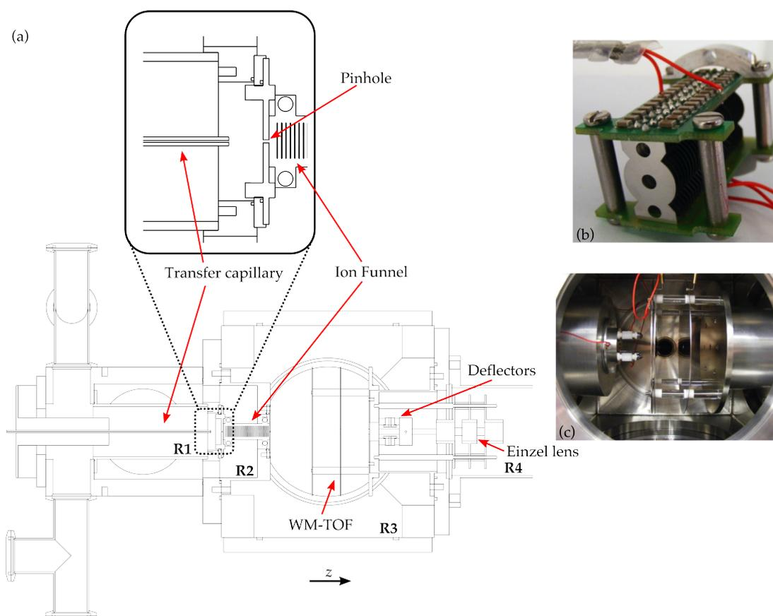
Figure 2.2: Overview of the low vacuum side of the machine, containing regions 1 to 4. (a) Technical drawing, with important parts labelled. Design and operation of these are explained in the text. The inset shows the interface between regions 1 and 2, separated by a pinhole with 1 mm inner diameter. Also shown are photos of the (b) ion funnel and (c) time-of-flight electrodes mounted inside the chamber.
