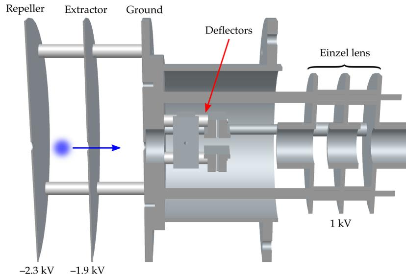
Figure 2.4: 3D rendering of the top hat and flange separating R3 and R4, mounted in this assembly are the time-of-flight (TOF) electrodes, the  $x,y$  deflector plates and Einzel lens. Ions are accelerated in the direction shown and temporally separated by mass-to-charge ratio. The deflector plates allow for small corrections to the beam path ( $x,y$  directions), while the Einzel lens spatially focusses ions onto the centre of the flight ( $z$ ) axis.
