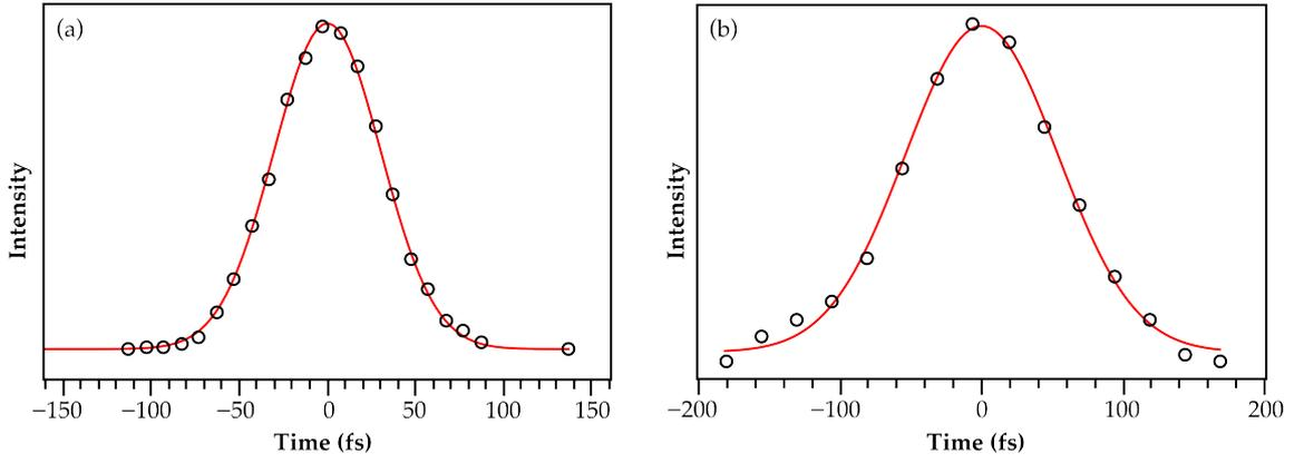
Figure 2.15: Measured intensity cross-correlations between pump and probe pulses at 400 nm + 800 nm (a) and 480 nm + 800 nm (b). The Gaussian fit yields a FWHM for the cross-correlations of 61 fs and 108 fs respectively.
