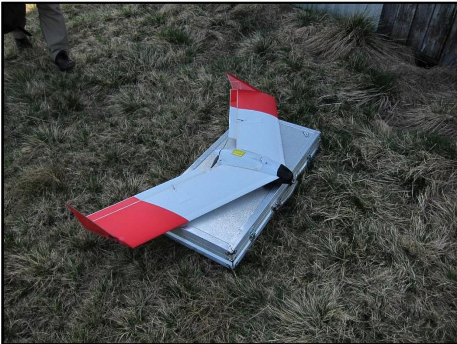
**Figure 7:** The PAMS SmartOne B UAS assembled along with its case
