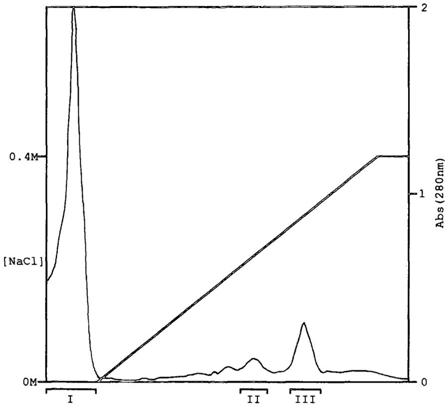
**Figure 35.** Column profile from S-sepharose chromatography of QRG, using 25mM formate buffer pH4.1, 0-0.4M NaCl. Peaks I, II and III were pooled to give SQRG-I, SQRG-II and SQRG-III, respectively.
