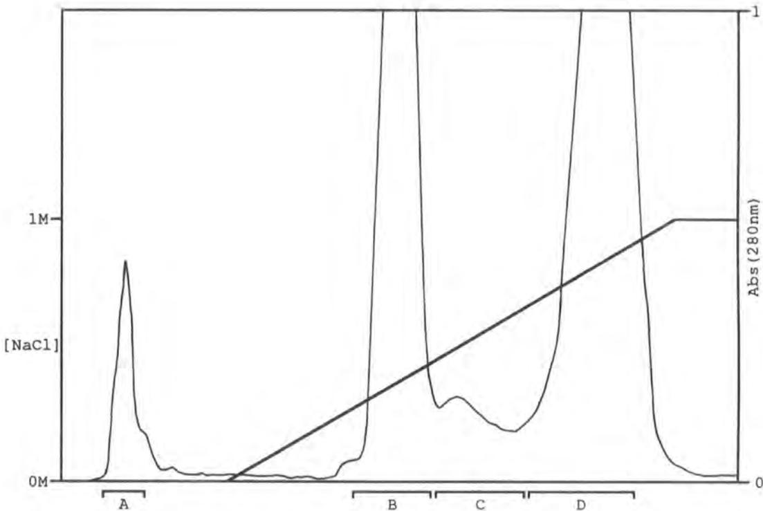
**Figure 62.** Profile of *E. coli* extract separation achieved by Q-sepharose chromatography. Pooled fractions are indicated.
