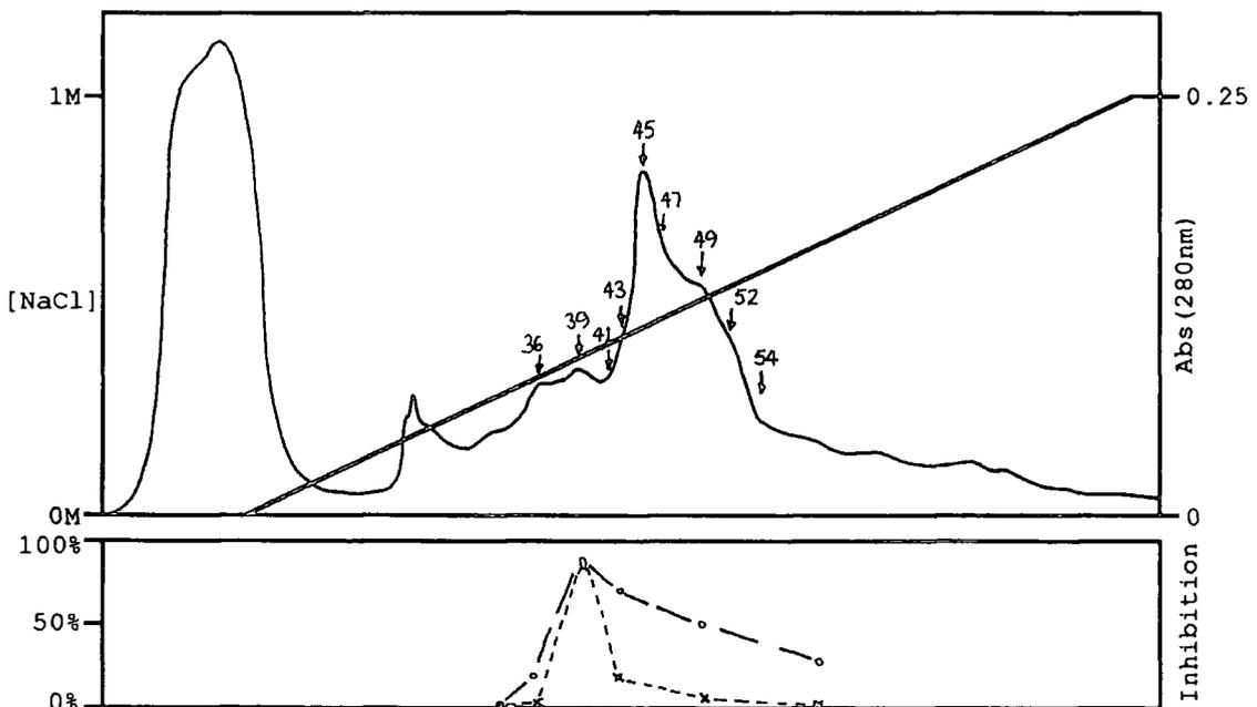
**Figure 43.** Profile obtained from S-sepharose chromatography of BB3-2. Chromatography was conducted using the same conditions as described in Figure 40. Inhibition assays were conducted, using the substrate Z-Phe-Arg-AMC, against LGE ( $\circ$ ) and papain ( $\times$ ).
