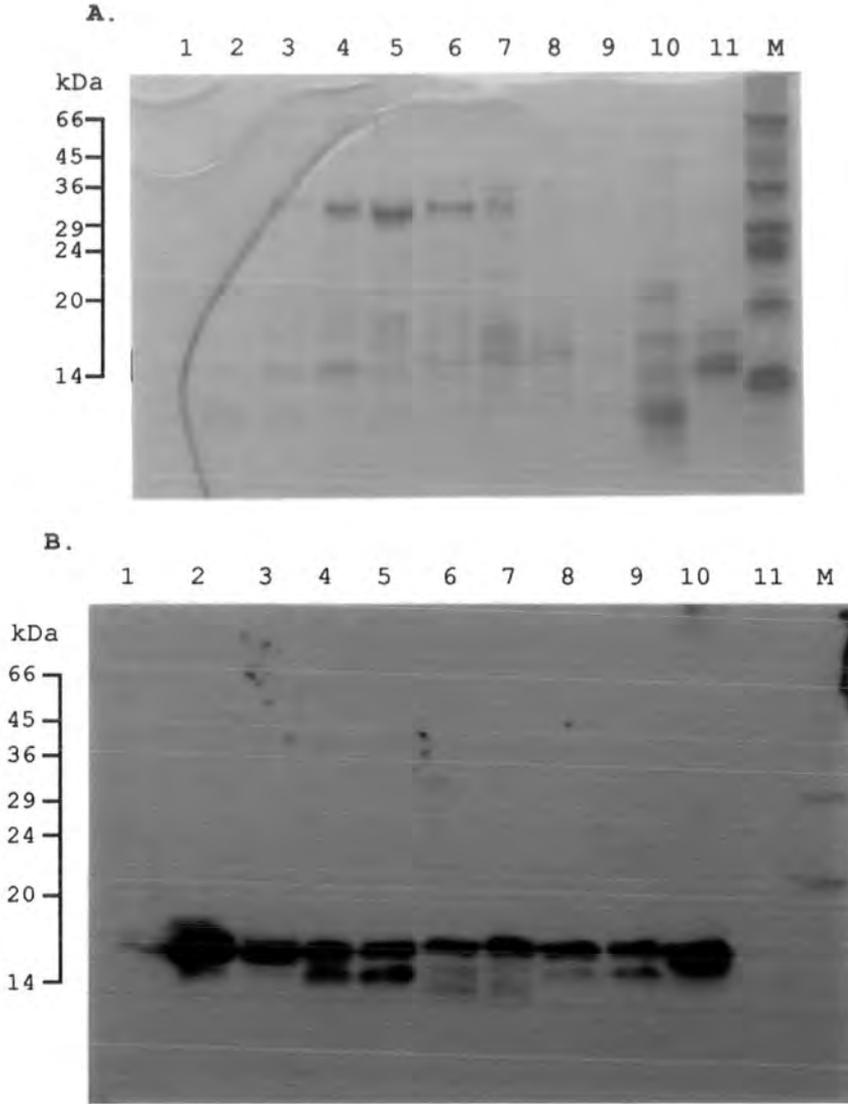
**Figure 44.** SDS-polyacrylamide gel (panel A) and western blot (panel B) of rice fractions following cation-exchange chromatography. Lanes 1-9, fractions 36, 39, 41, 43, 45, 47, 49, 52 and 54, respectively, from the chromatography of BB3-2; lane 10, BB3-11; lane 11, BB3-12; and M, molecular weight markers.
