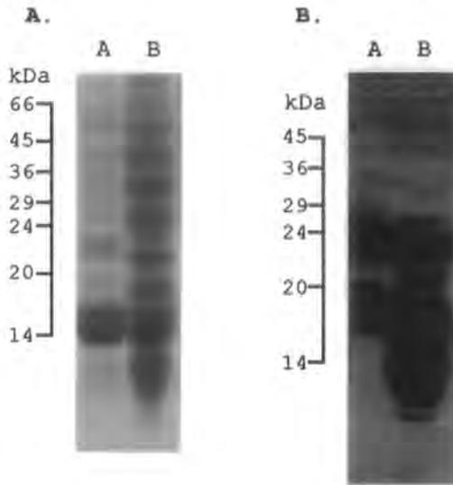
**Figure 40.** SDS-PAGE (panel A) and western blot (panel B) analysis of fractions precipitated between 0-30% (lane A) and 30-65% (lane B) saturation with ammonium sulphate.
