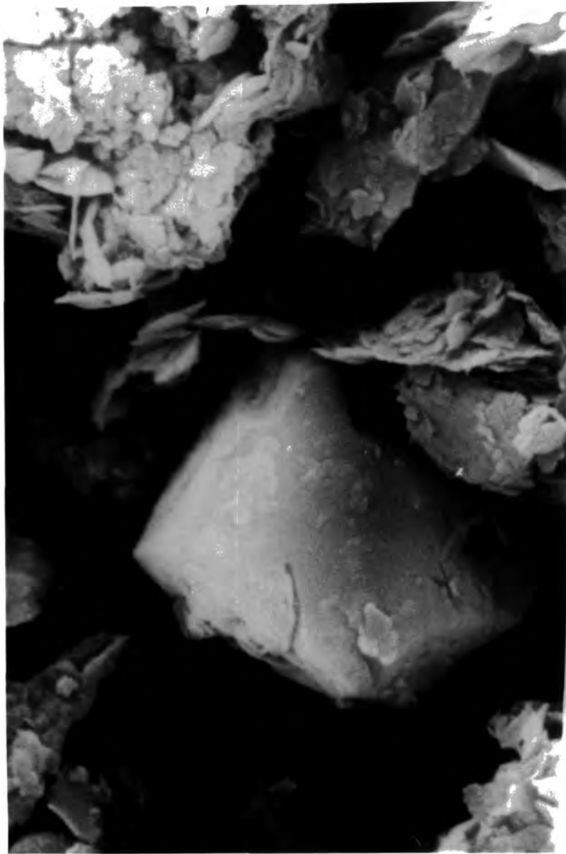
Figure 4.2.3 Sample FF3 showing in the centre a 'clean' quartz grain with negligible clay covering and clearly defined fracture faces. On the top right is a grain consisting of loosely bound clay minerals which form discrete particles in this sample. WD 7 mm; x10 000; 1 cm= 0.8 \mu m.
