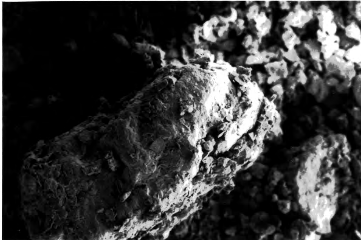
Figure 4.2.23 Sample HAZ1 - occasional larger mineral grains observed in this sample tended to be clay-coated and weathered, as in the case of this feldspar grain. WD 6 mm; x500; 1 cm= 15 \mu m.
