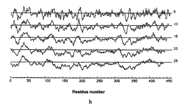
Figure 29: Hydropathy profiles of aerolysin A. hydrophila. Program PLOT.A/HYD5 was used with the hydropathy scales of Eisenberg (a) (Eisenberg *et al.*, 1984) and Argos (b) (Argos *et al.*, 1982). The numbers at the right side represent the moving average windows along the sequences. The regions above the horizontal lines represent the hydrophobic stretches, and below the lines, the hydrophilic ones.
