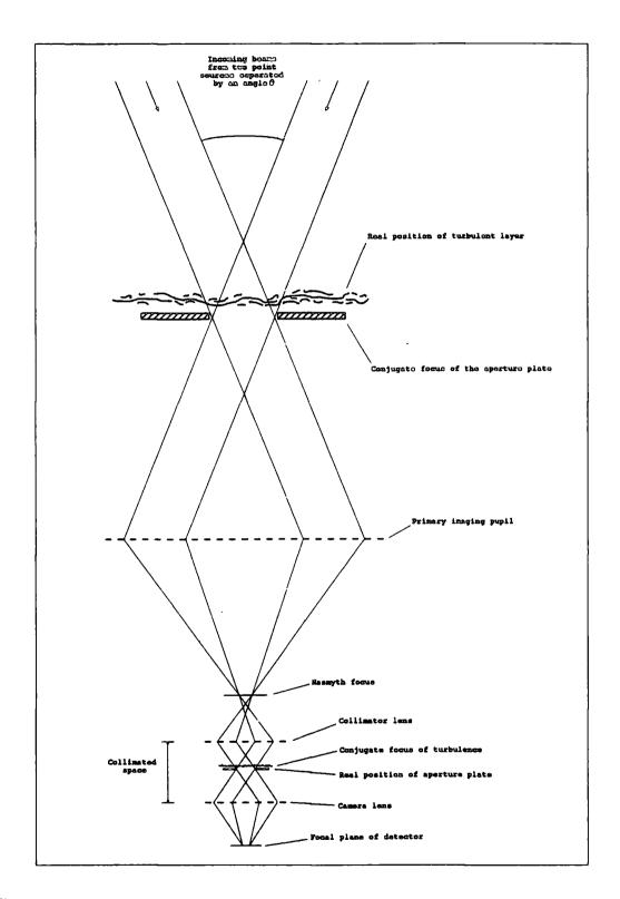
Figure 5.2: Schematic diagram showing the effect of putting the aperture plate at the conjugate focus of the turbulence on the isoplanicity. In this simple model the amount of overlap of the two beams, as they traverse the turbulent layer, will determine the degree to which their tilts are correlated.
