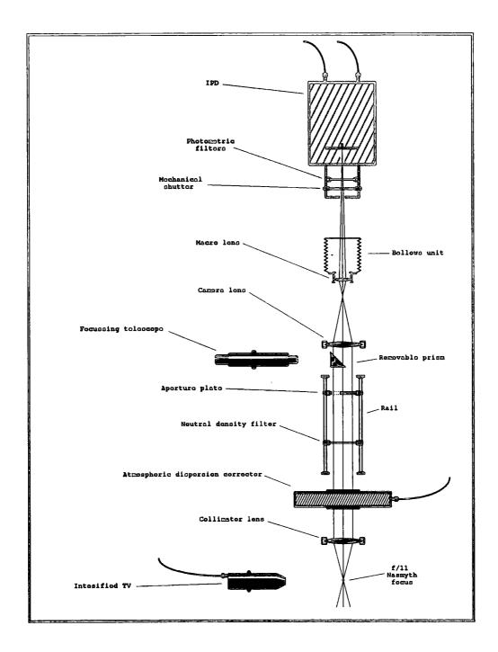
Figure 5.4: Diagram illustrating a typical configuration of the TRIFFID apparatus. The size and conjugate focus position of the aperture can be easily altered, as can the field scale. The focussing telescope and TV camera are used only for set-up purposes
