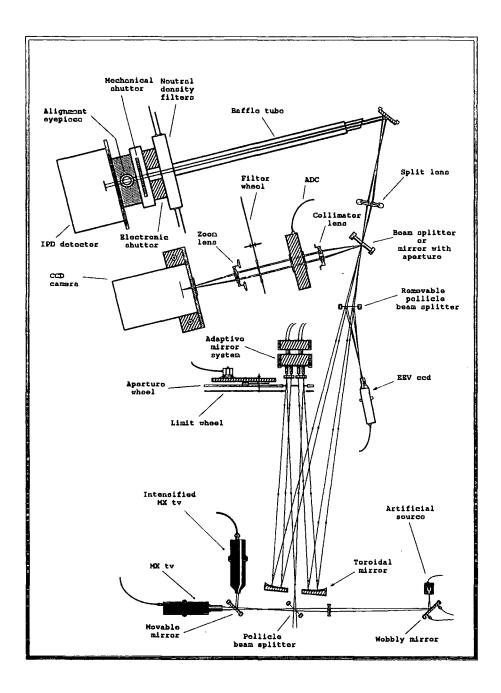
Figure 5.5: Diagram illustrating a typical configuration of the MARTINI apparatus. The light from the telescope enters from the bottom to be focussed in the centre of the toroidal mirror. The precise configuration may be altered to accommodate different beam-splitter arrangements etc.
