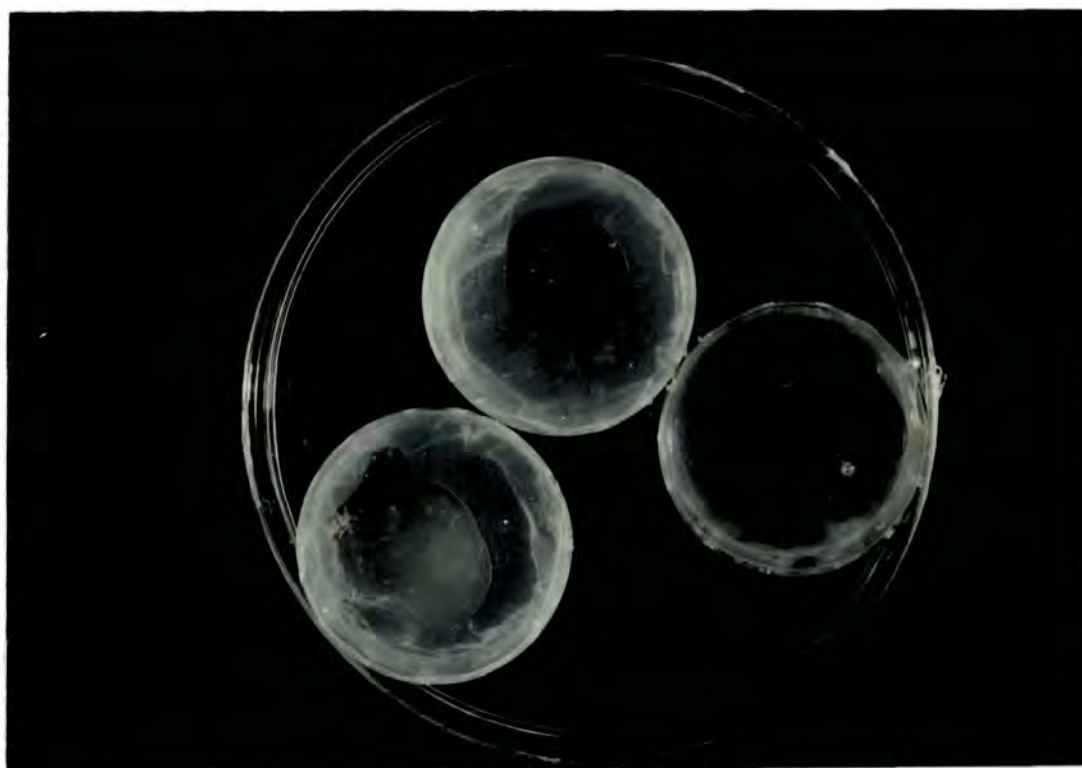
Plate 3: Replicated floating humidity chambers used for qualitative and quantitative determination of BPH honeydew excretion
