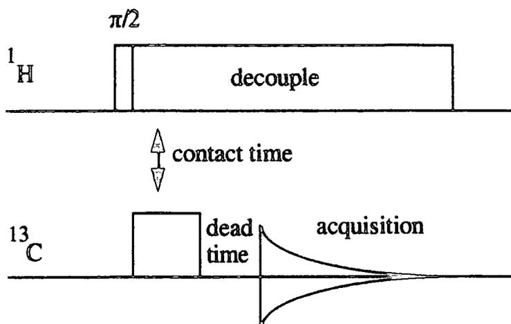
Figure 4.1 continued - The solid-state NMR pulse sequences
