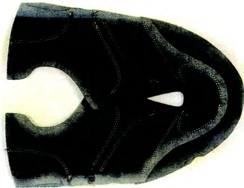
Fig 1.5 The assembly of a shoe upper, comprising a number of skived components ( by permission BUSM Ltd ).
