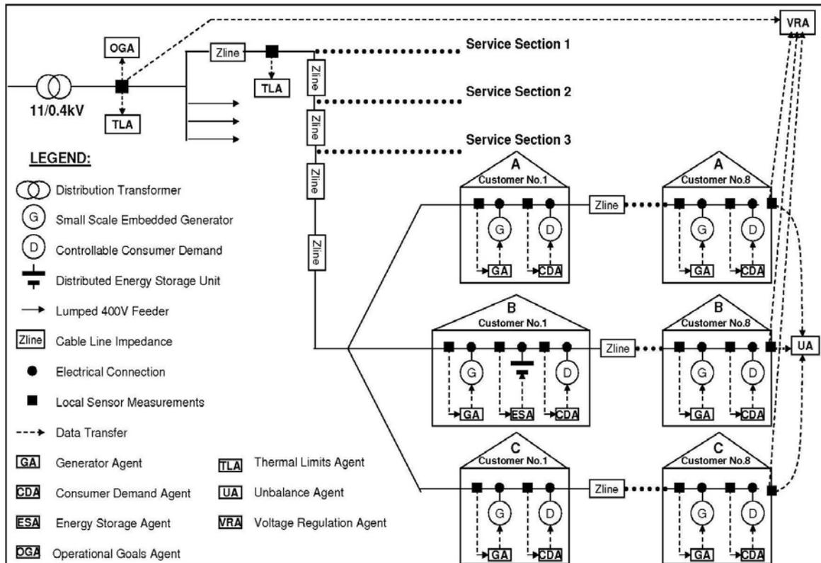
**Figure 6.6:** The MAS-based control approach on the case study SSEZ.
