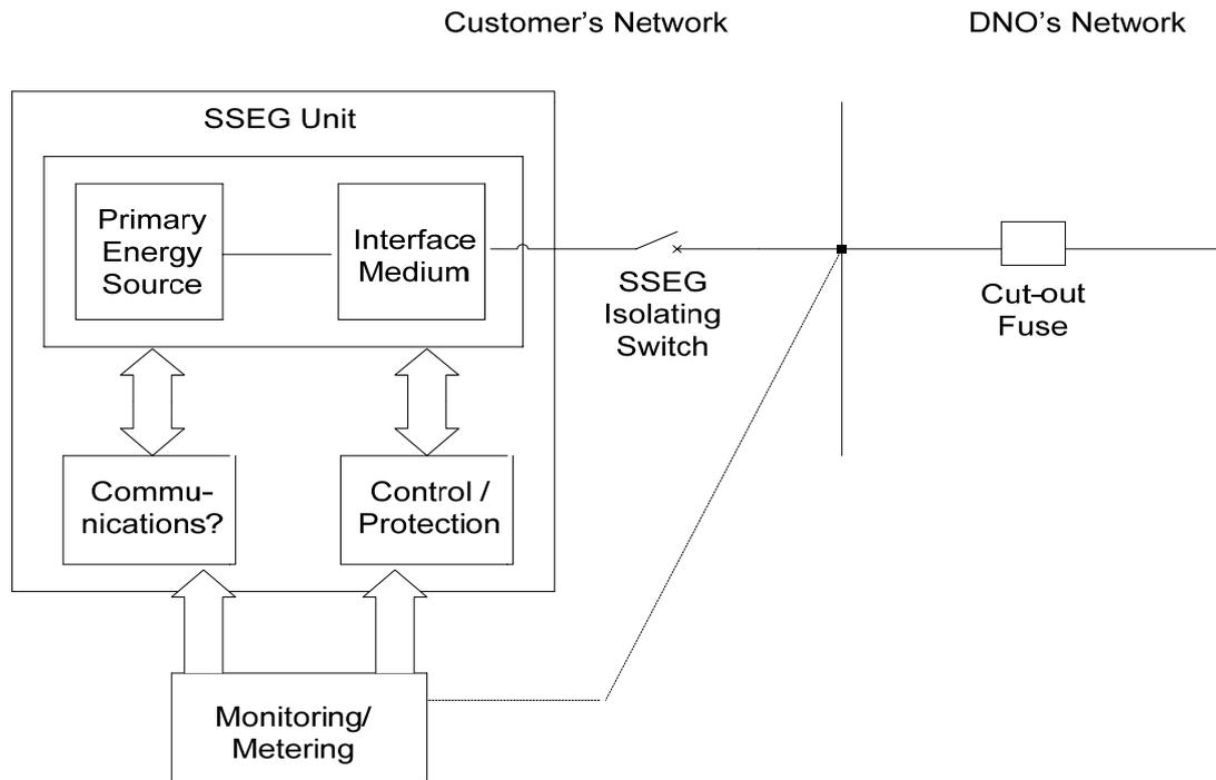
**Figure 2.5:** Block diagram showing a typical SSEG installation.
