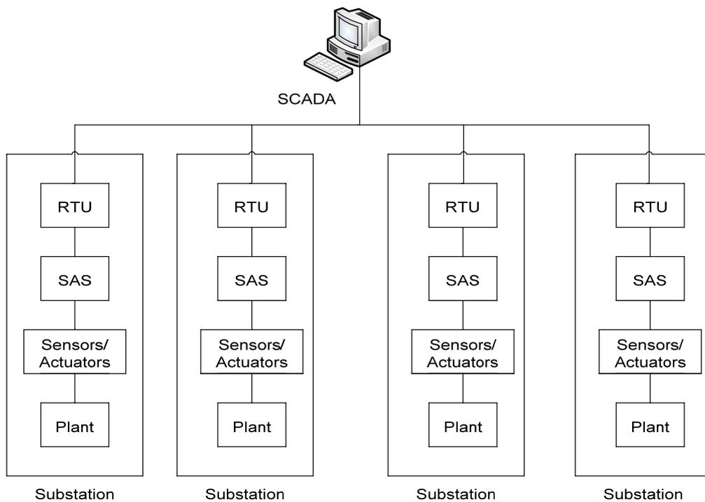
**Figure 2.1:** A Supervisory Control and Data Acquisition system.
