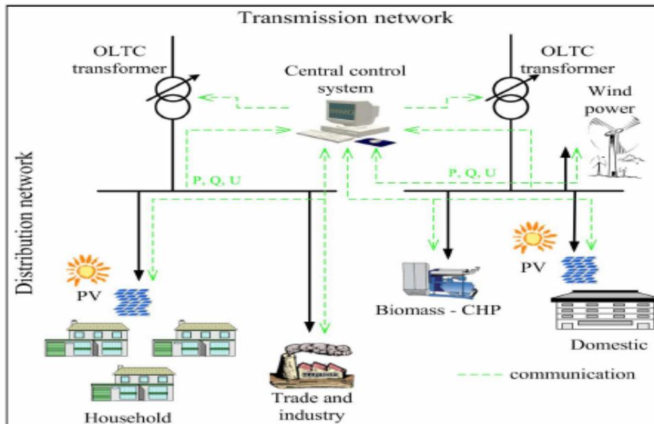
**Figure 2.2:** Example of an active transmission and distribution system [14].
