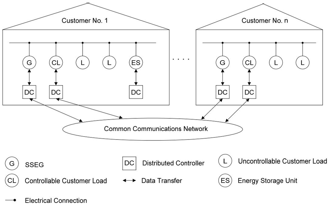
**Figure 5.2:** Distributed control operation for an SSEZ.
