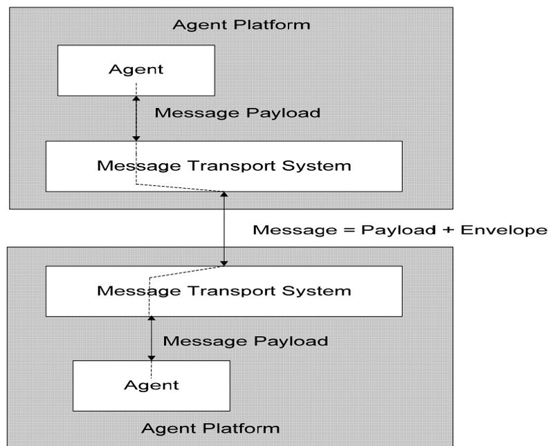
**Figure 3.7:** The FIPA Message Transport Reference Model [120].
