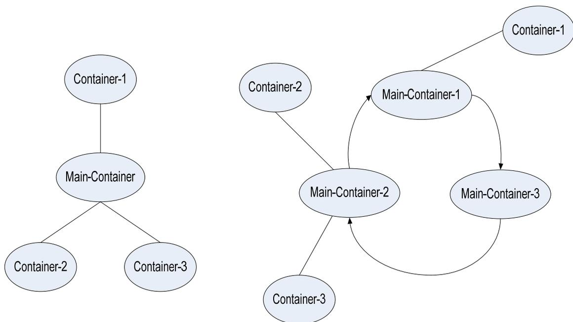
**Figure 8.15:** A JADE platform without (left) and with (right) the main container replication service.
