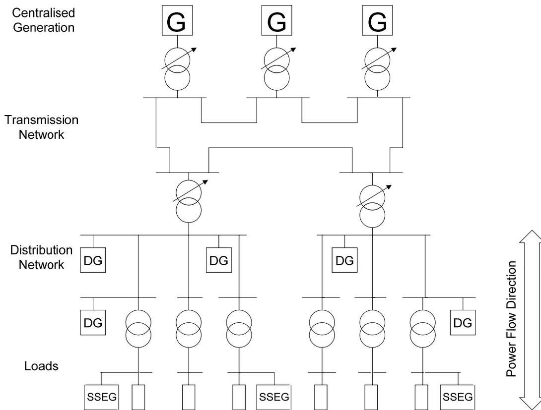
**Figure 1.2:** Structure of electrical power systems with DG and SSEG present.
