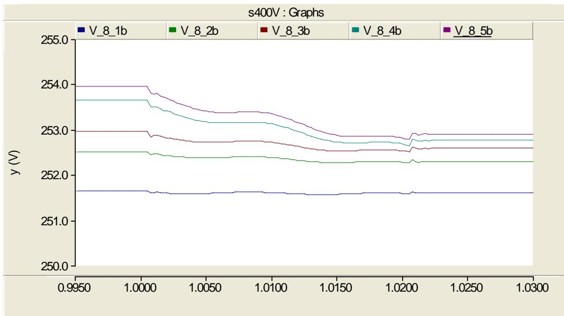
**Figure 8.6:** Instantaneous customer voltages showing the dynamic operation of the MAS-based control system.
