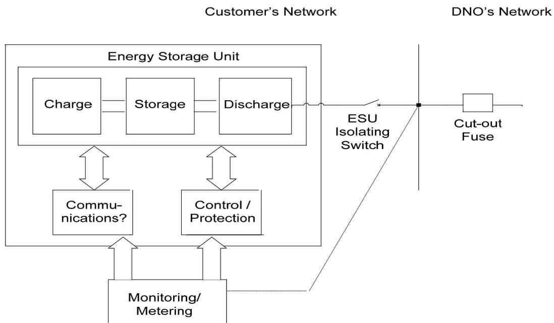
**Figure 2.6:** Block diagram showing a typical ESU installation.
