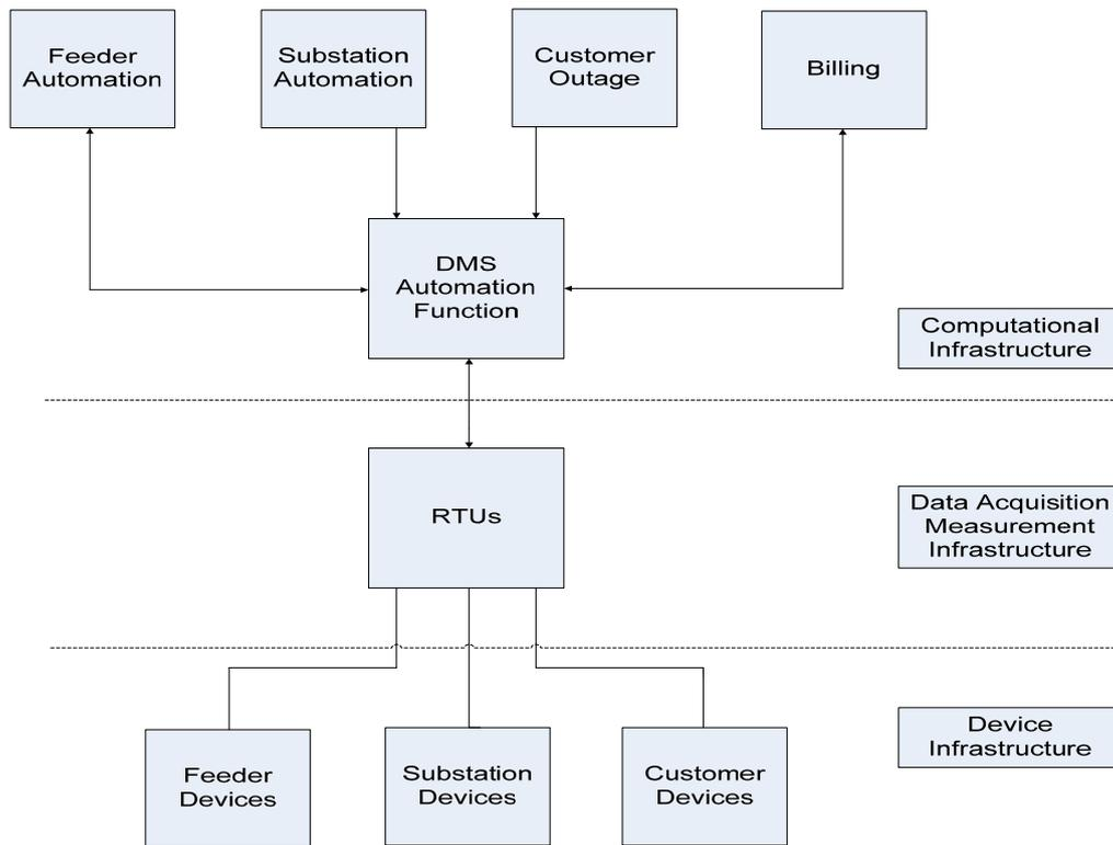
**Figure 2.3:** Typical telecommunication setup in distribution networks.
