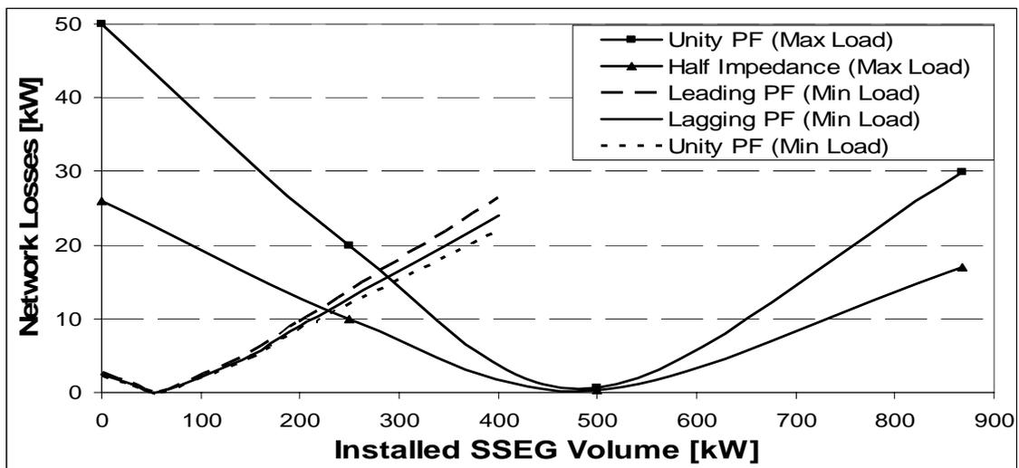
**Figure 4.7:** Results for network losses in the UK generic network.
