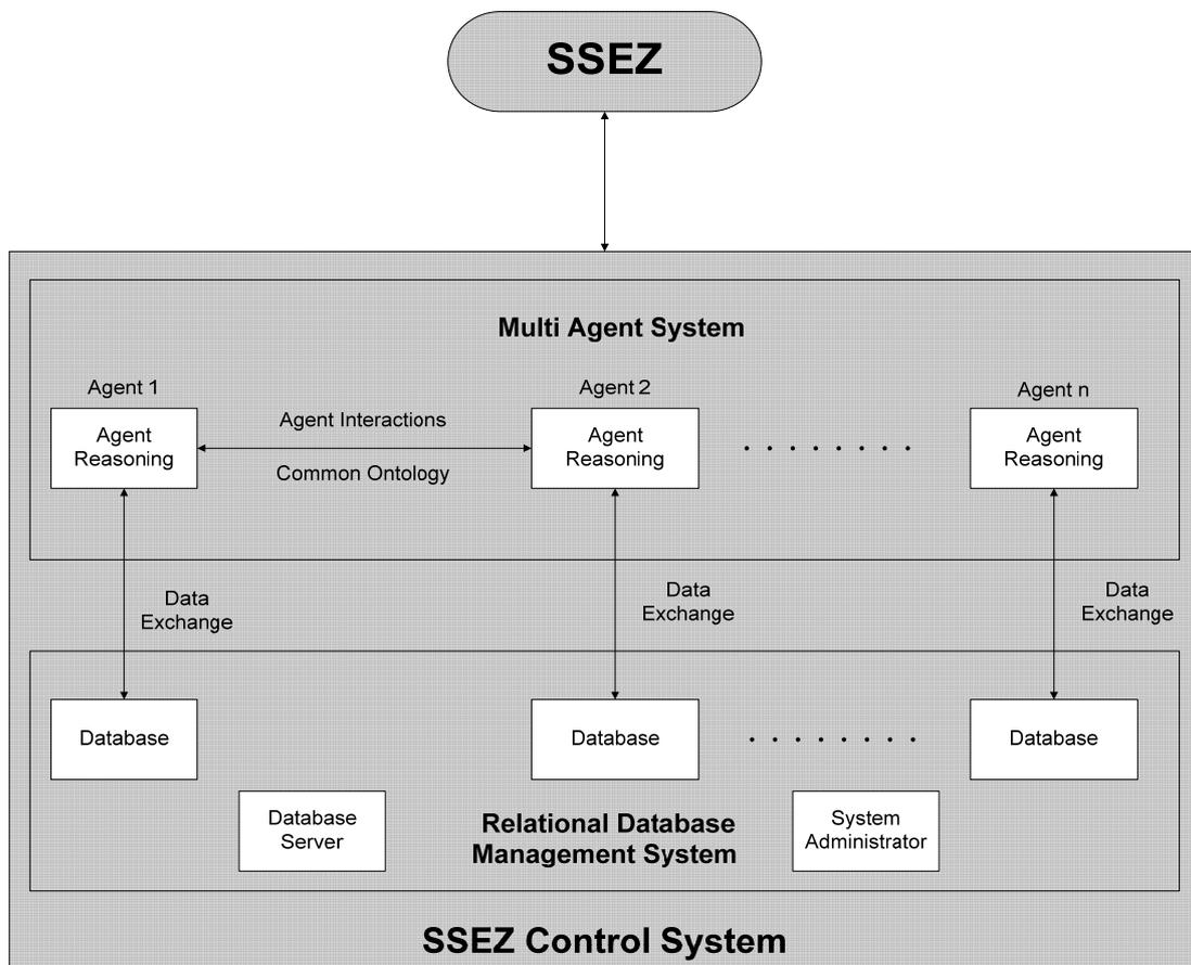
**Figure 6.1:** The design of the SSEZ control system.
