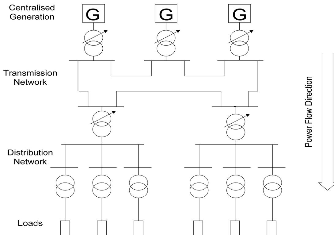
**Figure 1.1:** Conventional structure of electrical power systems.
