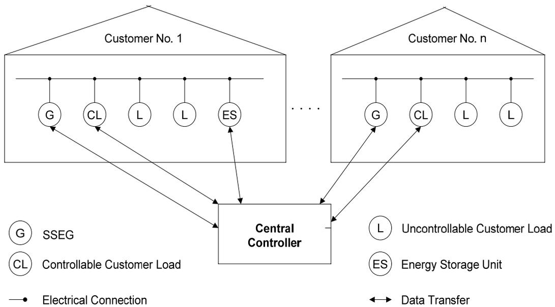
**Figure 5.1:** Centralised control operation for an SSEZ.
