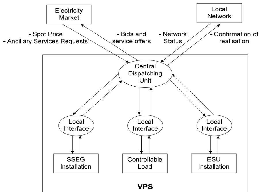
**Figure 1.7:** Architecture of a centralised Virtual Power Station [50].
