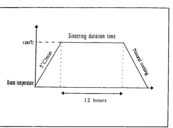
Figure (3.2) : Typical heating profile for the sintering cycle.
