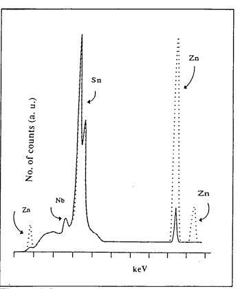
**Figure (6.6) :** EDAX spectrum for a  $Nb_2O_5$ -doped sample (2%  $Nb_2O_5$ ). Dotted line; normal sintering : solid line; sintering temperature > 1350°C.
