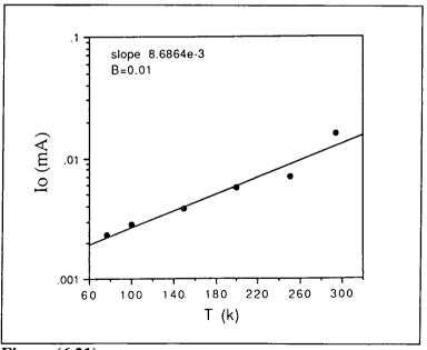
Figure (6.21) : A plot of Io with temperature for In-doped M.S diodes.
