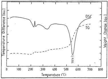
Figure (4.15) : Thermal gravimetery (TG) and differential scanning calorimetry (DSC) for reduced Zn<sub>2</sub>SnO<sub>4</sub>, heated in air.
