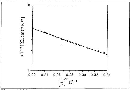
Figure (6.16) : Conductivity -Temperature characteristics for an In-doped sample.
