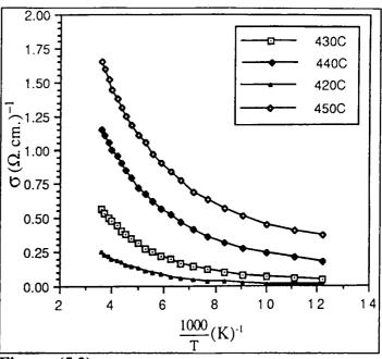
Figure (5.2) : Conductivity versus 1/T from 77K to room temperature, for samples annealed in the temperature range 420°C to 450°C.
