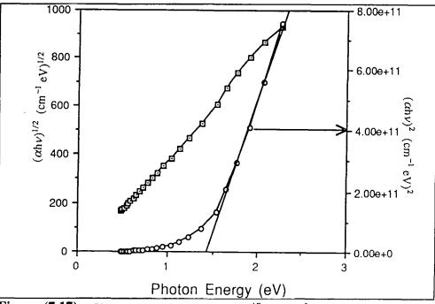
Figure (7.17) : Photon energy (hv) versus  $[(\alpha hv)^{1/2} & (\alpha hv)^2]$  for a film grown at room temperature.
