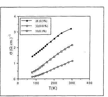
Figure (6.10): Conductivity-Temperature characteristics for Nb<sub>2</sub>O<sub>5</sub>-doped reduced samples.
