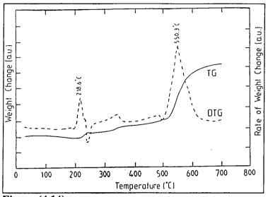
Figure (4.14) : Thermal gravimetery (TG) and differential thermal gravimetry (DTG) for reduced  $Zn_2SnO_4$ , heated in air.
