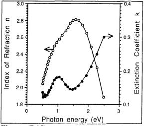
Figure (7.15) : Optical constants versus photon energy for a film grown at 200°C.
