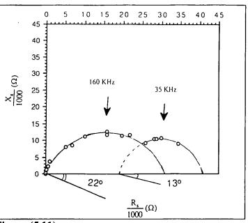
Figure (5.11) : A.c. impedance plot for a sample reoxidised in air (600°C for 12 hours), after reduction.
