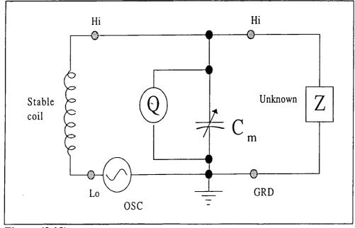
Figure (3.13) : Equivalent circuit for the Q-meter.
