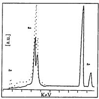
Figure (4.7) : EDAX spectra taken from a typical sintered sample : (a) (solid line) a typical pore, (b) (dotted line) general area scan. The sample was sintered at 1280°C for 12 hours.
