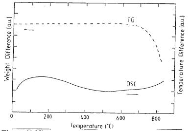
**Figure (4.13) :** Thermal gravimetery (TG) and differential scanning calorimetry (DSC) for as-fired  $Zn_2SnO_4$ , heated in 10%  $H_2$  / 90%  $N_2$ .
