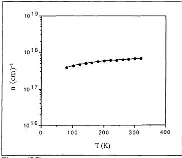
Figure (5.7) : Carrier concentration (n) versus temperature.
