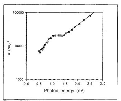
Figure (7.19) : Absorption coefficient versus photon energy for film grown at 200°C.
