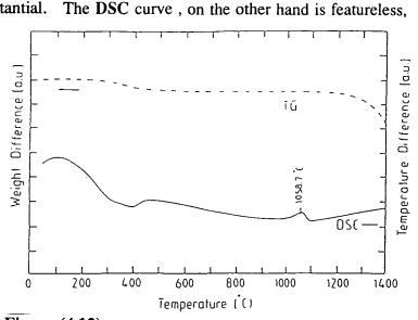
Figure (4.12) : Thermal gravimetry (TG) and differential scanning calorimetry (DSC) for a 2ZnO :  $SnO_2$  mixture, heated in air.
