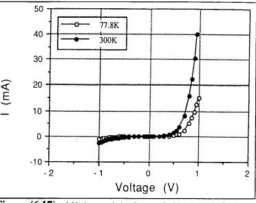
Figure (6.17) : I-V characteristics for a typical In-doped M.S. diodes.
