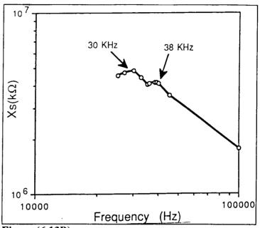
Figure (6.13B) : Reactance (Xs) versus frequency from impedance studies for 5% Nb<sub>2</sub>O<sub>5</sub>-doped sample.
