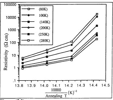
Figure (5.3) : Resistivity versus reciprocal annealing temperature.
