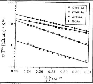
Figure (6.12) :  $log (\sigma T^{1/4})$  vs  $(1/T)^{1/4}$  characteristics for Nb<sub>2</sub>O<sub>5</sub>-
