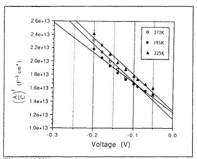
Figure (6.22) : The C<sup>-2</sup> versus V curves for a Au/In-Zn<sub>2</sub>SnO<sub>4</sub>/In,Ga diode at different temperatures.
