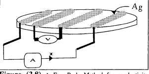
Figure (3.8) : Four-Probe-Method for conductivity measurements.
