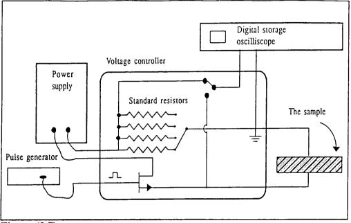
Figure (3.7) : Apparatus for Current-Voltage measurements.
