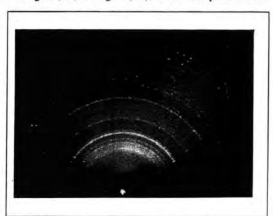
the Figure (7.3) : RHEED pattern from a film grown at 200°C.
