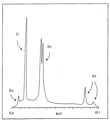
Figure (7.5) : EDAX spectrum of surface of a thin film of Zn<sub>2</sub>SnO<sub>4</sub>.
