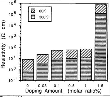
Figure (6.3) : Resistivity versus the doping level for  $V_2O_5$ -doped reduced samples.
