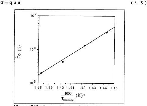
**Figure (5.9) :**  $T_{o}$  versus the reciprocal of the reducing temperature  $(1/T_{R})$ .
