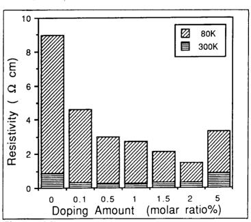
Figure (6.2) : Resistivity versus the doping level for  $Ta_2O_5$ -doped reduced samples.
