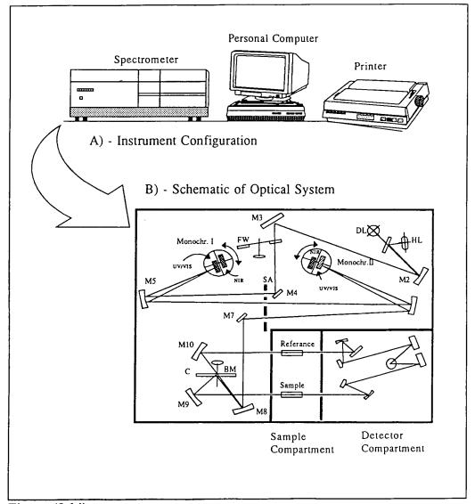
Figure (3.14) : Schematic of spectrophotometer system.
