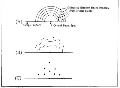
Figure (3.6) : RHEED patterns; a) randomly oriented polycrystalline sample, b) Ploycrystalline sample with preferred order, c) Single crystal sample.
