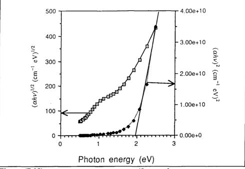
Figure (7.18) : Photon energy (hv) versus  $[(\alpha hv)^{1/2} \& (\alpha hv)^2]$  for a film grown at 200°C.
