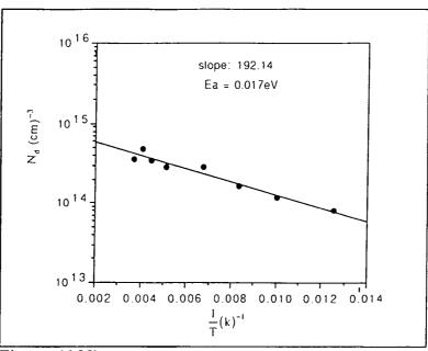
Figure (6.23) : Log  $N_d$  (from C-V study) versus 1/T for In-doped  $Zn_2SnO_4$  diodes.
