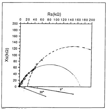
Figure (6.14) :A.c. impedance plot for 1% Nb<sub>2</sub>O<sub>5</sub>-doped sample.
