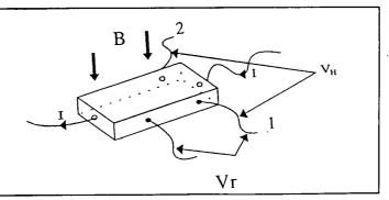
Figure (3.10) : Five-Probe-Method for Hall measurements.
