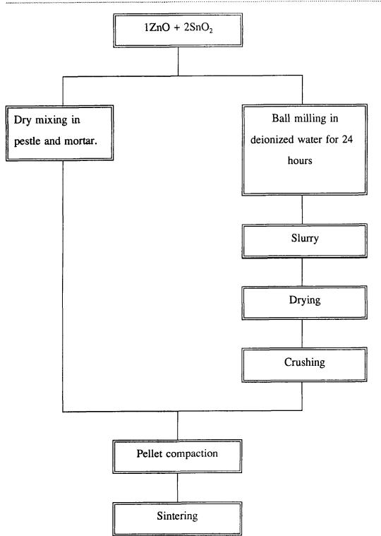
Figure (3.1) : Mixed oxide route for  $Zn_2SnO_4$  processing.
