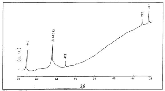
Figure (7.1) : X-ray diffractogram showing principal peaks of zinc stannate from a film grown at a substrate temperature of  $\sim 30^{\circ}$ C.
