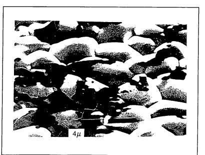
Figure (4.5): Photograph showing strange deposits on the surface of a sample fired at  $T > 1300^{\circ}C$  (for 12 hours).
