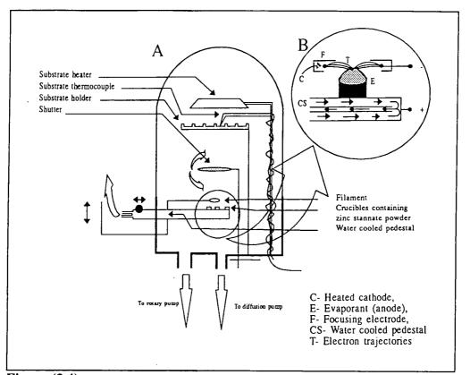
Figure (3.4) : a)-Schematic diagram of the Electron Beam Evaporator, b)- Schematic diagram of the Electron Beam Source.
