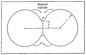
Figure (2.1) : Sintering by evaporisation condensation [ref. 2].
