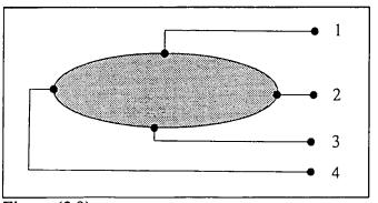
Figure (3.9): Four probe method, (Van der pauw method) for the resistivity measurements and Hall coefficient.
