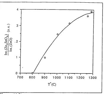
Figure (4.2): The variation of  $Zn_2SnO_4/ZnO X$ -ray peak intensity ratio versus the firing temperature.
