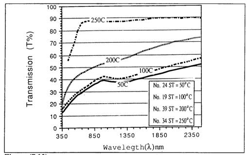
Figure (7.12) : Transmission (T%) versus wavelength ( $\lambda$ ) for thin films of Zn<sub>2</sub>SnO<sub>4</sub> grown at substrate temperatures between 50°C to 250°C.
