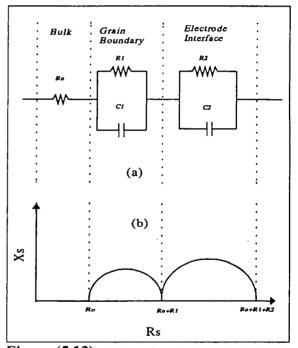
Figure (5.13) : Schematic equivalent circuit (a) and corresponding impedance plot (b) for electrical transport through a ploycrystalline solid.
