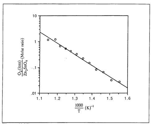
Figure (4.11): The amount of  $O_2$  loss during reduction of  $Zn_2SnO_4$  versus the heating temperature.
