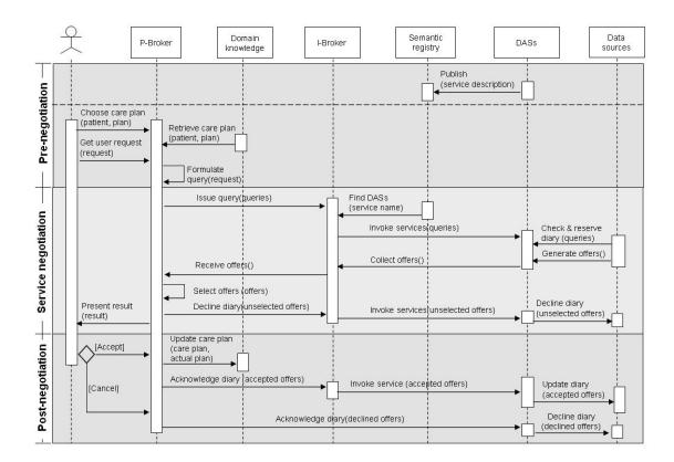
Figure 6.8: The sequence diagram of CAPTAIN
