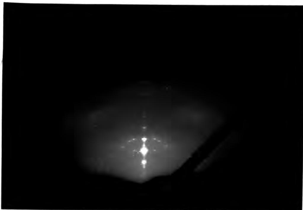
Figure 5.36 RHEED pattern for 6 layers of perylene:TA 1:12.
