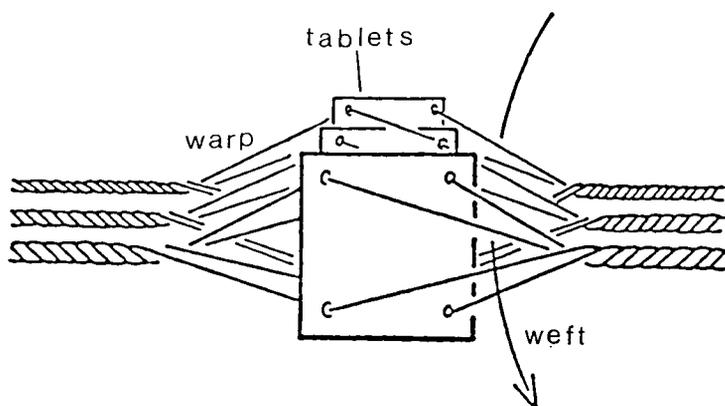
Fig. 4.9. Tablet-weaving using 3 4-hole square tablets and 12 warp-threads.
