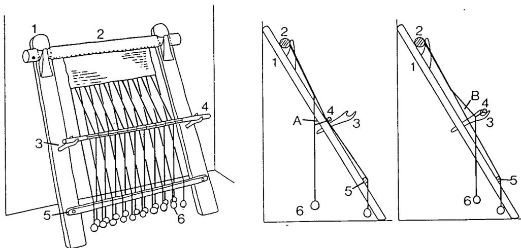
Fig. 4.12. Warp-weighted loom:
