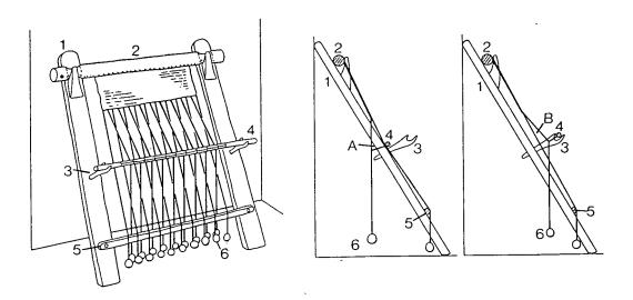
Fig. 4.12. Warp-weighted loom: <u>1.</u> uprights; <u>2.</u> cloth-beam; <u>3.</u> heddle-rod bracket; <u>4.</u> heddle-rod; <u>5.</u> fixed shed-rod; <u>6.</u> loom-weights. <u>A.</u> natural shed; <u>B.</u> countershed.
