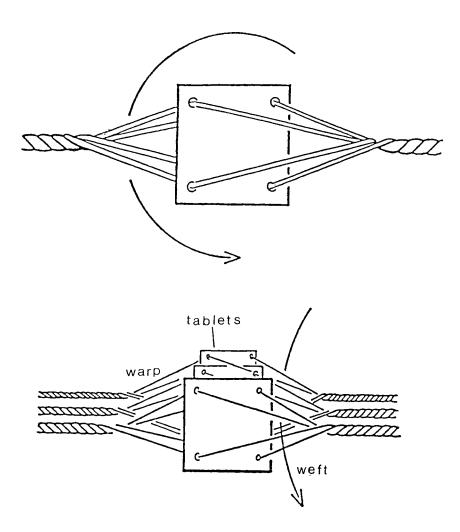
Fig. 4.9. Tablet-weaving using 3 4-hole square tablets and 12 warp-threads.
