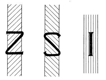
Fig. 4.7. Spin direction: clockwise - Z-spun. anti-clockwise - S-spun. twistless - I-twistless
