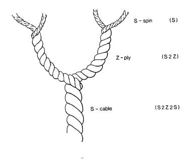
Fig. 4.8. Plying and cabling yarn.
