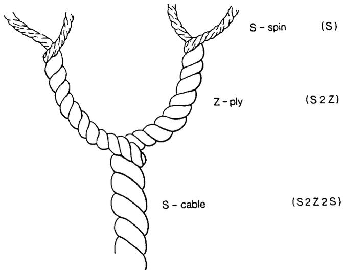
Fig. 4.8. Plying and cabling yarn.
