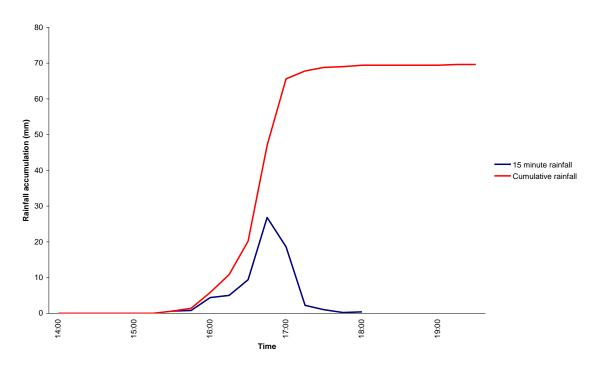
Figure 1.3: Rainfall recorded at Hawnby (number two) rain gauge on the 19th June 2005, showing 15 minute rainfall accumulations (blue line) and cumulative storm rainfall (red line). Rainfall data provided by the Environment Agency.
