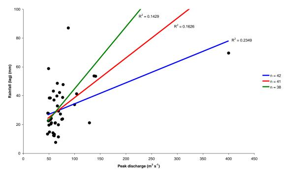
Figure 5.15: Relationships between peak discharge and rainfall for the largest flow events recorded at Broadway Foot, 1978-2009. Rainfall data formed from data contained in the Met Office MIDAS database, discharge data provided by the Environment Agency except 19th June 2005 peak discharge (estimate by Wass et al., 2008).
