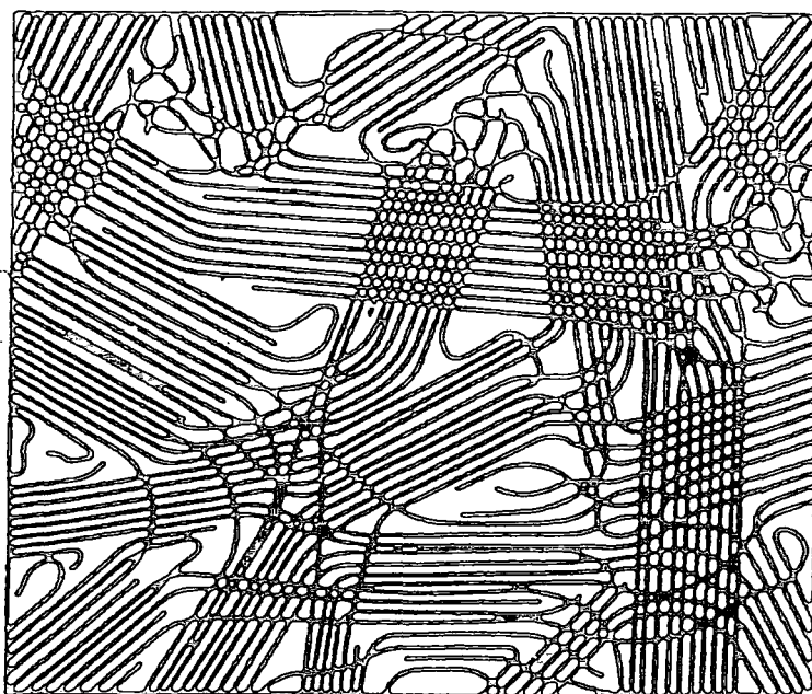
Figure 6.2 The 'fringed micelle' or two-phase model for polymers representing ordered regions, or domains, in a less well ordered matrix.
