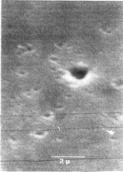
Figure 6.5. Crater formation on copper electrodes. Magnetically driven with an arc velocity 4 \text{ ms}^{-1} .
