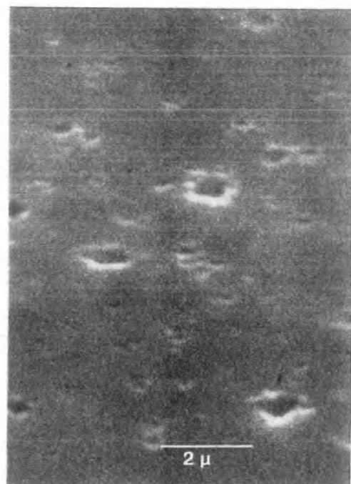
Figure 6.18. Crater formation on copper electrodes. Aerodynamically driven with an arc velocity 16 ms -1 .
