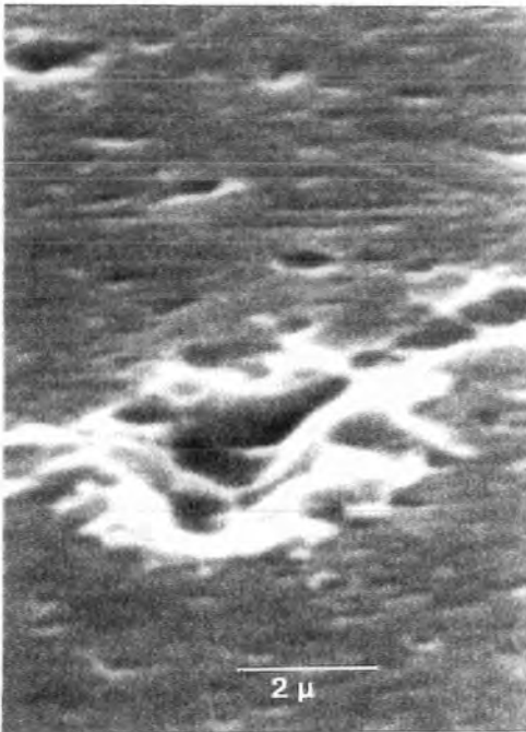
Figure 6.7. Crater formation on copper electrodes. Magnetically driven with an arc velocity 10 \text{ ms}^{-1} .
