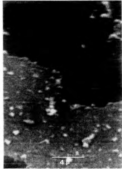
Figure 7.3. Crater formation on copper electrodes, with a 100 nm oxide layer.
