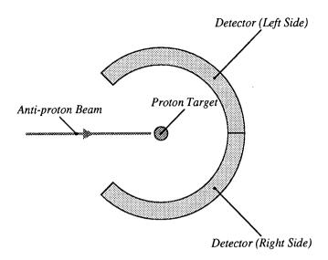
Figure 2.5: An idealised  $\overline{p}p \to \pi\pi$  experimental setup. The proton target is polarisable in the up and down directions (i.e. in or out of the plane of the figure).
