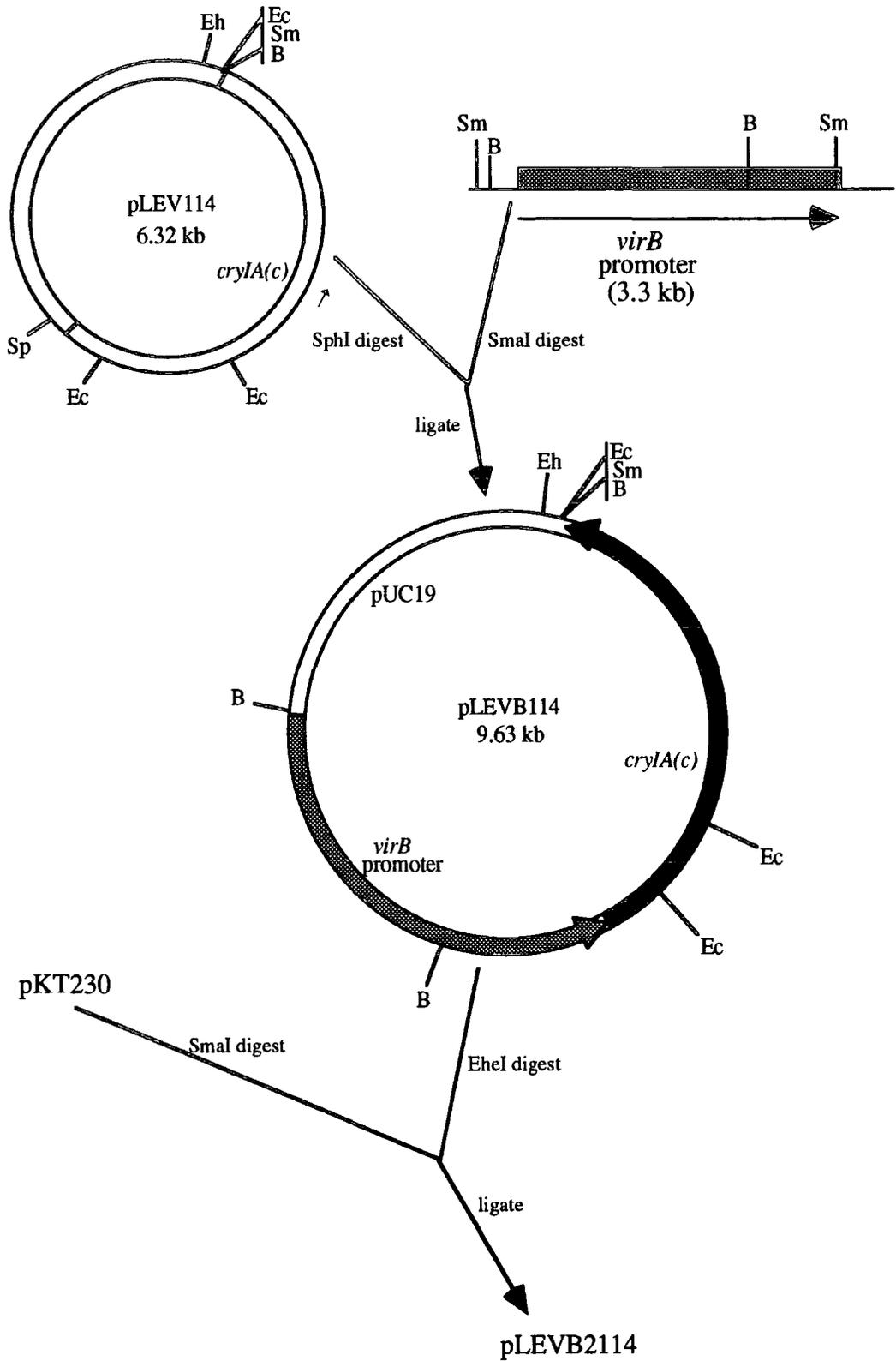
**Figure 5.3.2.a** - showing construction of the broad host range plasmid, pLEVB2114, containing *vir*-inducible *cryIA(c)*. Restriction sites shown - B = BamHI, Ec = EcoRI, Eh = EheI, Sm = SmaI, Sp = SphI.
