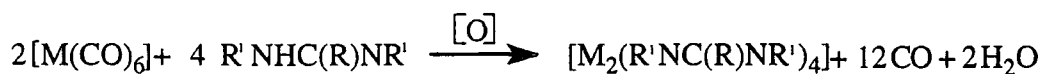
Figure 1.15 Reaction pathway of [M(CO)_6] with amidines ( R = H, CH_3, Ph ; R' = Ph, p tolyl)
