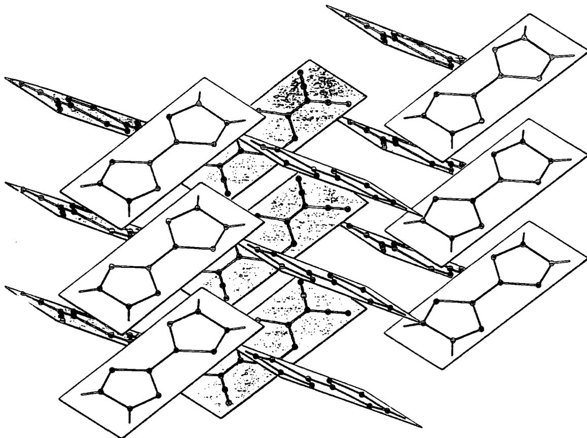
*Figure 1.2. - 'Herringbone' stacking in crystals of TTF-TCNQ.*
