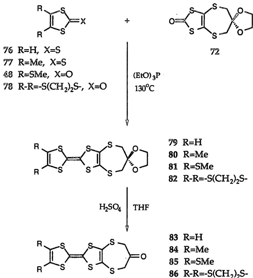
**Scheme 2.12.** - Synthesis of unsymmetrical TTF derivatives containing exocyclic ketone functionality.
