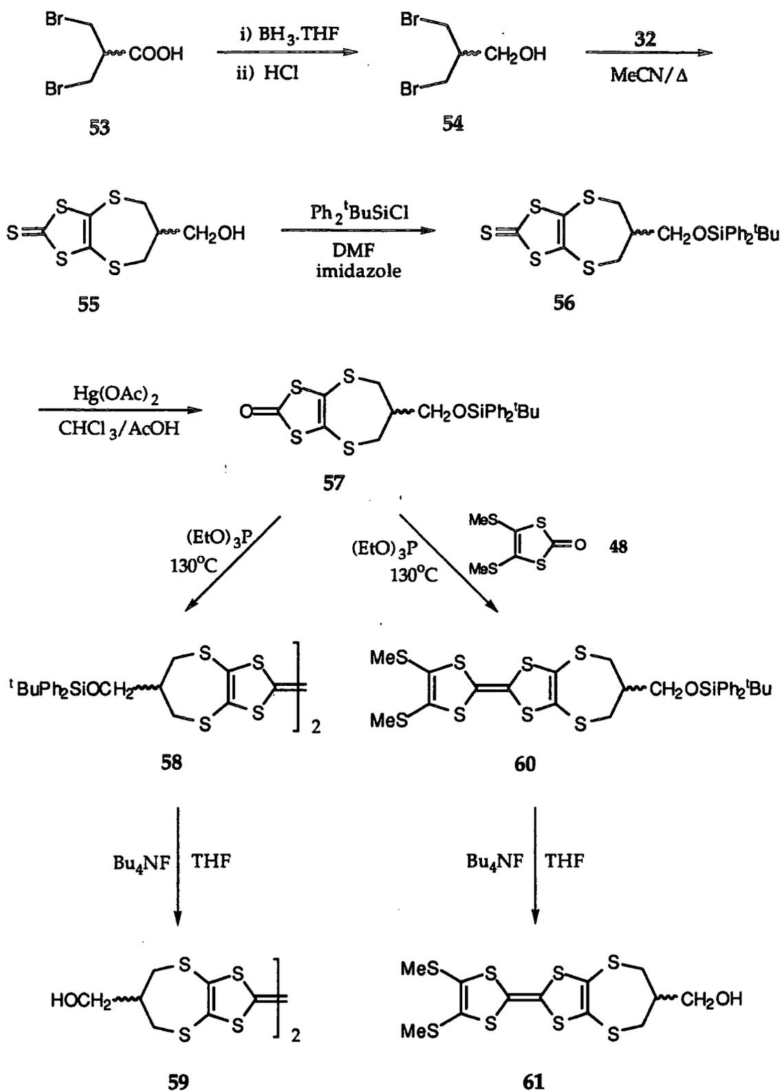
Scheme 2.6. - Synthesis of symmetrical and unsymmetrical TTF derivatives containing the 4,5-[2-(hydroxymethyl)propylene-1,3-dithio] unit.
