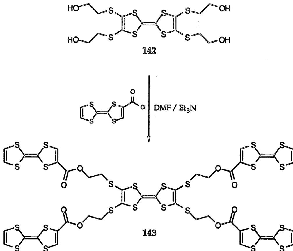
*Scheme 3.13. - Assembly of a penta-TTF macromolecule.*
