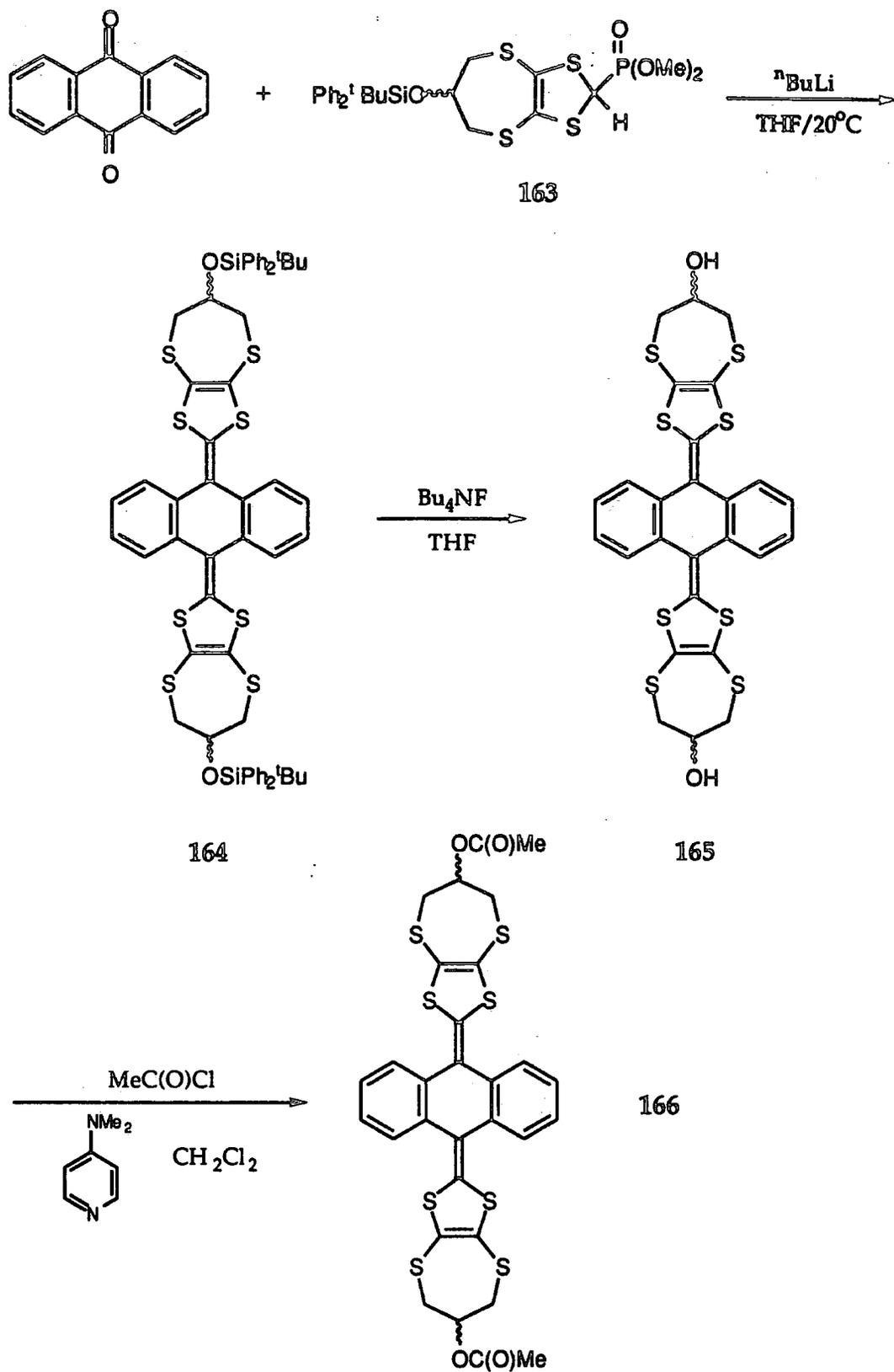
**Scheme 4.5.** - Synthesis of extended-TTF derivatives with functionalised 1,3-dithiole units.
