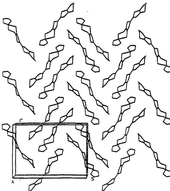
*Figure 2.3. - X-Ray crystal structure of compound 82 projected along the a axis.*
