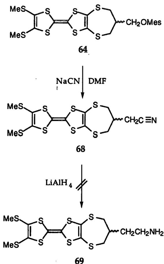
*Scheme 2.9. - Attempted amine synthesis via hydride reduction of a nitrile functionality.*
