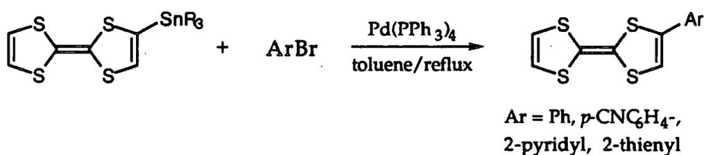
Scheme 1.6. - Cross-coupling reactions of trialkylstannyl-TTFs.
