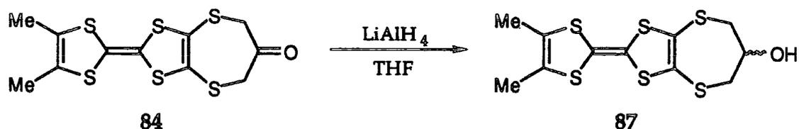
*Scheme 2.13.* - Synthesis of a mono-alcohol TTF system via hydride reduction of a ketone group.
