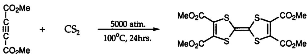
*Scheme 1.11.* - Reaction of an electrophilic acetylene with CS<sub>2</sub> under high pressure.
