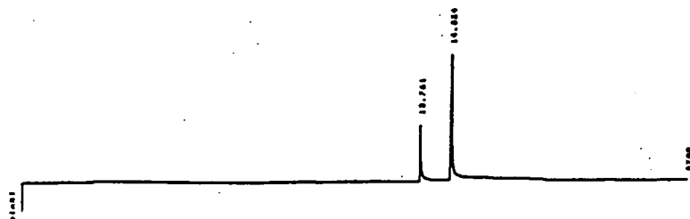
Appendix 1.10 GC trace of the product of the attempted reduction of dimethyl methyl-(3'-propionaldehydro)-malonate
