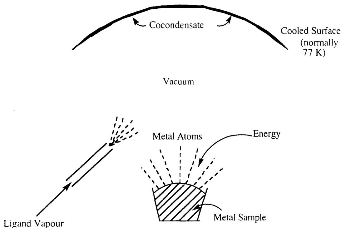
**Figure 7.** Basics of the MVS Technique
