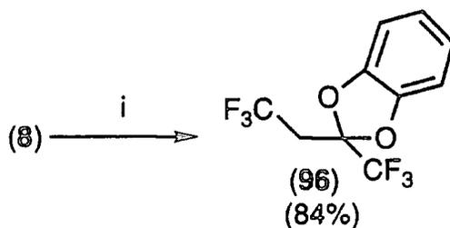
$i$  = Catechol,  $\text{Cs}_2\text{CO}_3$ , Acetonitrile, Room temperature
