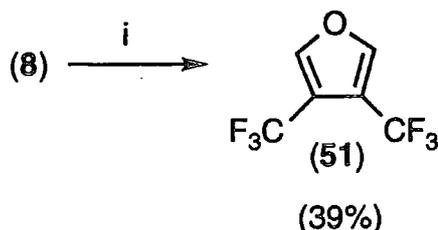
$i$  = 2-Furoic Acid,  $300^\circ\text{C}$ , Sealed metal tube
