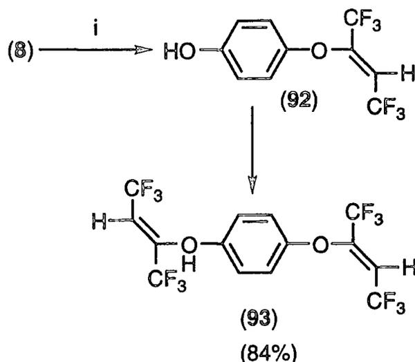
$i =$  Hydroquinone,  $\text{Cs}_2\text{CO}_3$ , Acetonitrile, Room temperature
