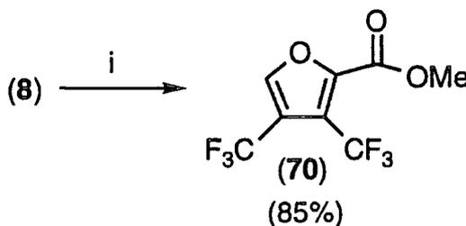
$i$  = Methyl 2-furanoate,  $250^\circ\text{C}$ , quartz tube
