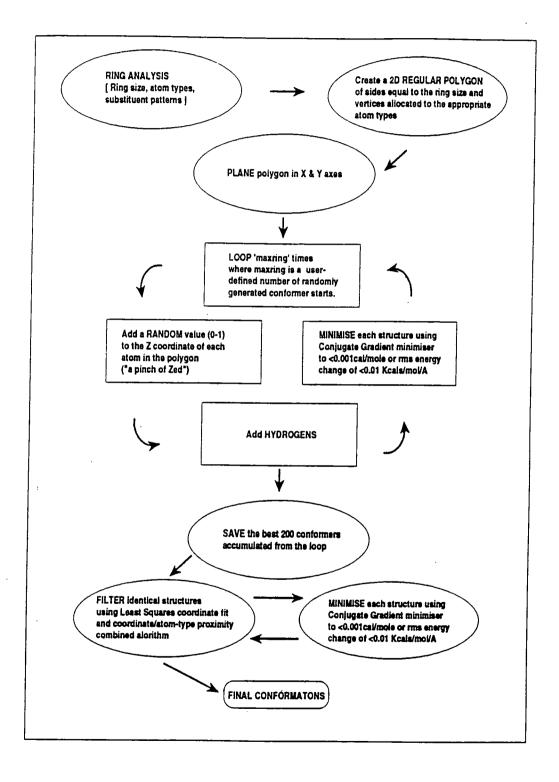
Figure 2.12 Flowchart detailing the operations involved in a COSMIC energy calculation
