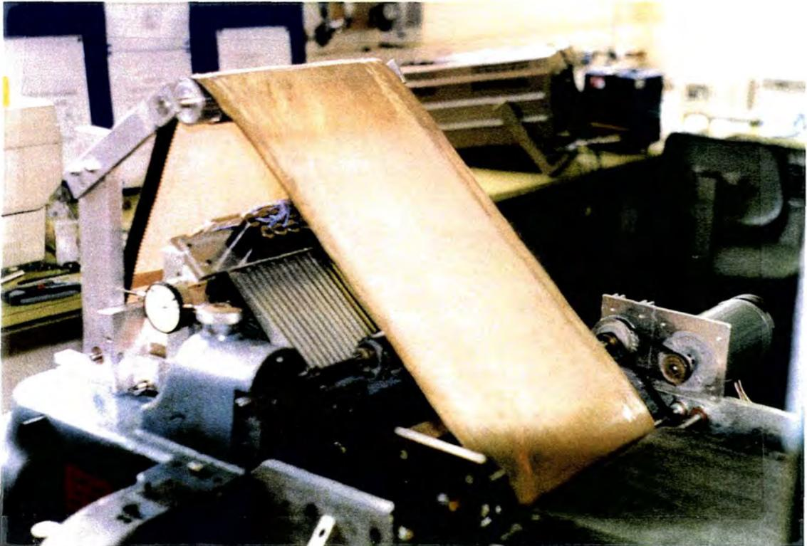
*FIG 1.7 Shows the appearance of the skiving system.*
