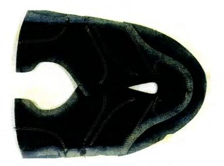
Fig 1.5 The assembly of a shoe upper, comprising a number of skived components (by permission BUSM Ltd).
