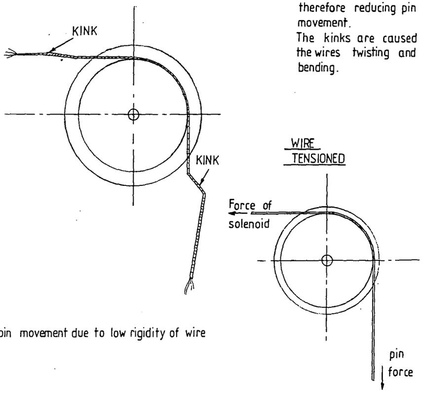
NOTE; As force is applied the kinks are stretched therefore reducing pin movement. The kinks are caused by the wires twisting and bending.
