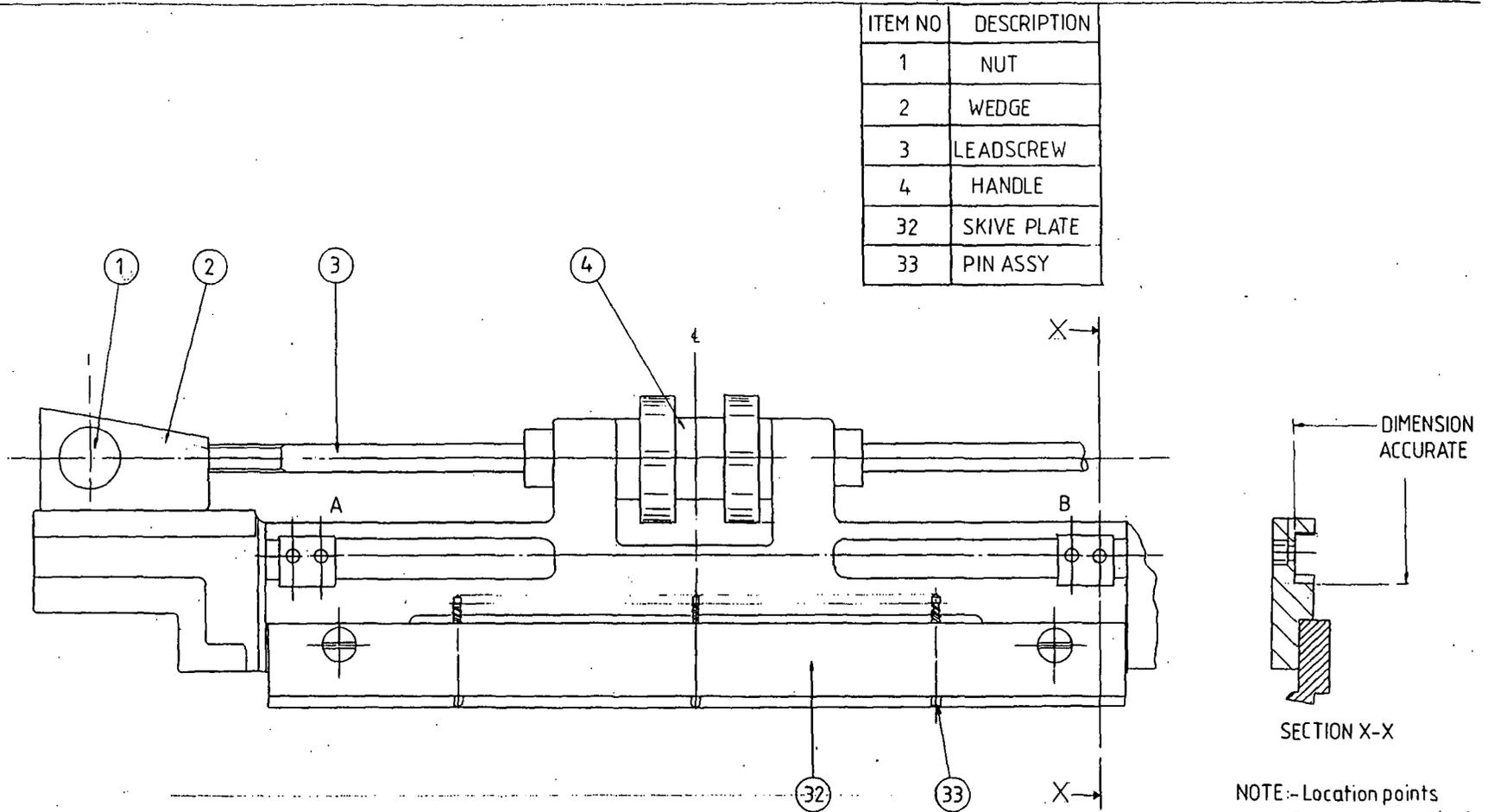
NOTE:- Location points A and B are premachined, therefore (during manufacture) accurate with respect to each other.
