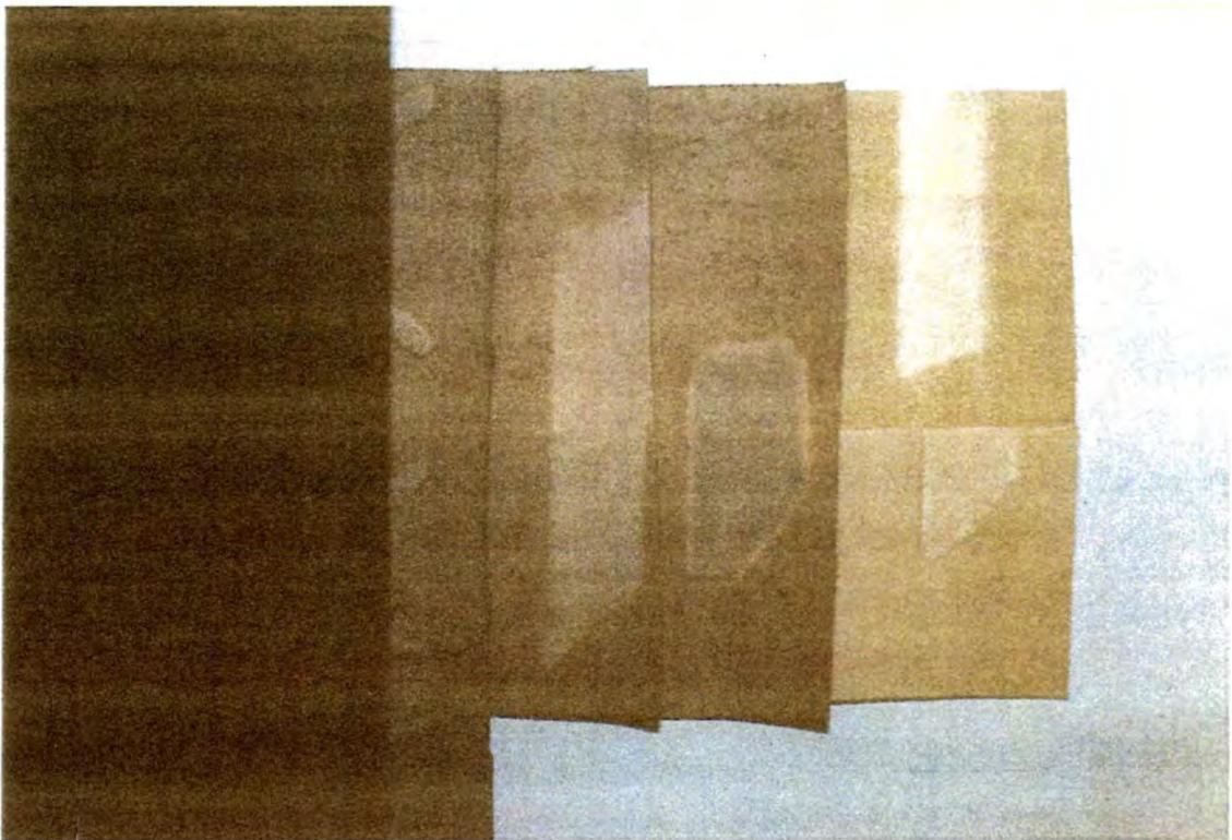
**FIG 3.0** Shows the Skiving tests done to prove that the required resolution pitch was 2mm and the skived leather with no stepping effect.
