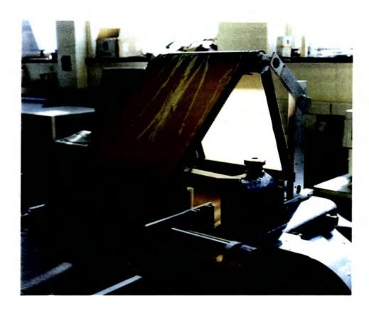
Fig. 3.3 Shows the old splitting machine and conveyor
