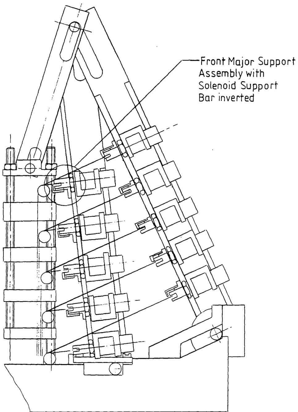
FIG 6-1 Shows inverted Solenoid Support Bar
