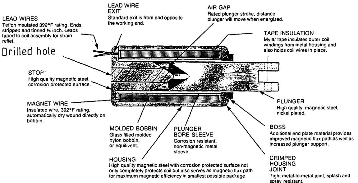
FIG 4-2 Shows hole drilled in solenoid
