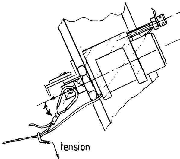
FIG 7-2(b) Shows wire pushing 'u'tube away from bar.
