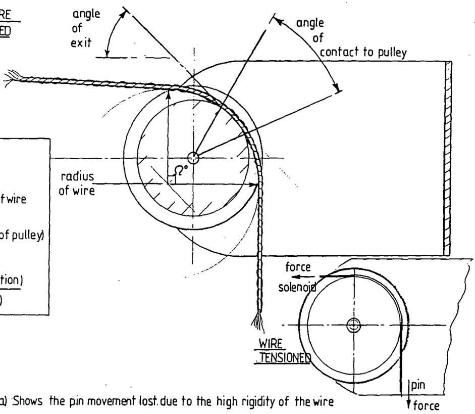
Movement lost at solenoid due to rigidity of wire is  $[\frac{\Omega^\circ}{360^\circ} \times 2\pi \times \text{radius of wire}] - (\frac{\Omega^\circ}{360^\circ} \times 2\pi \times \text{radius of pulley})$
