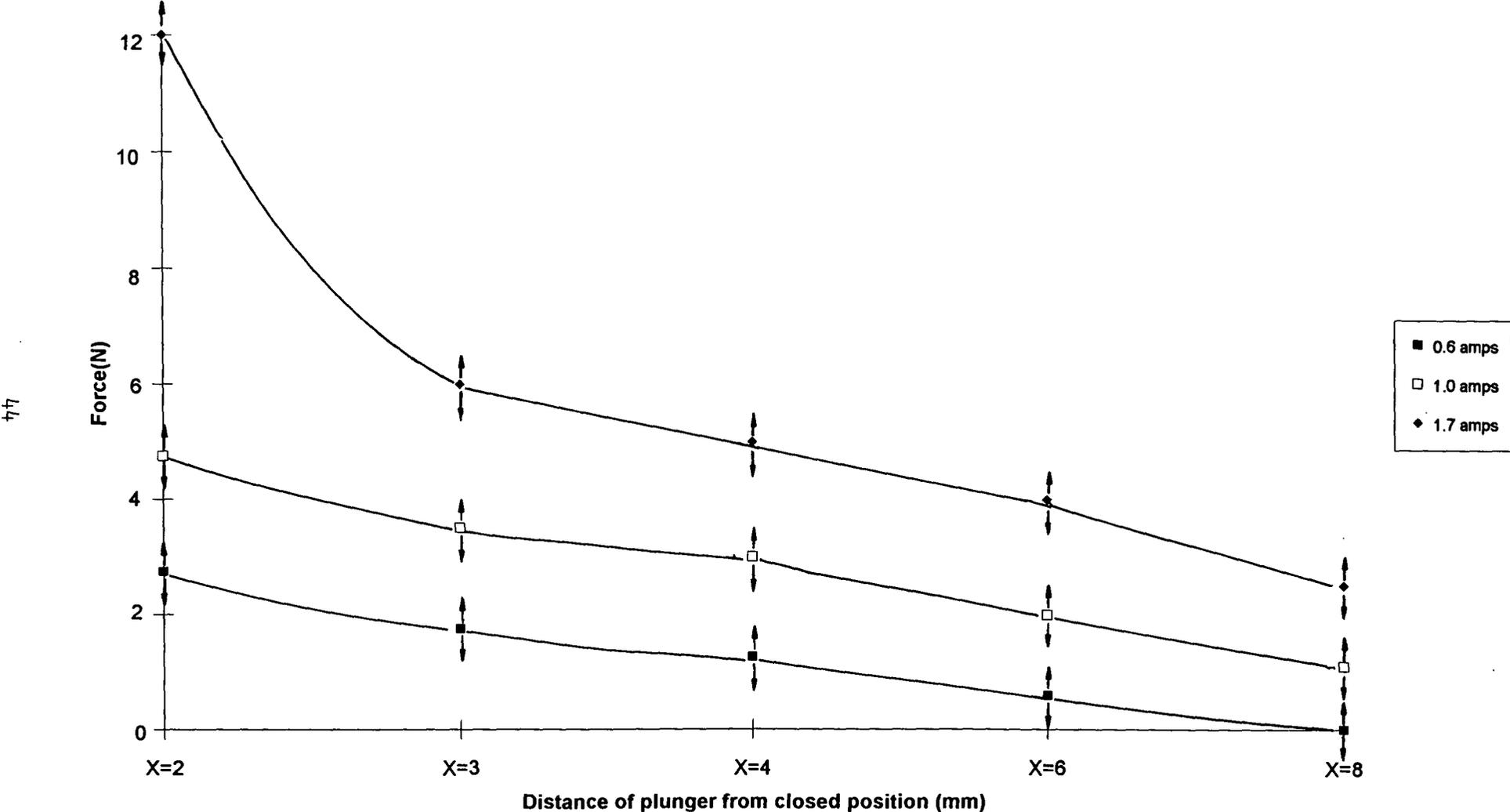
FIG 4.1 Shows force characteristics of new solenoids
