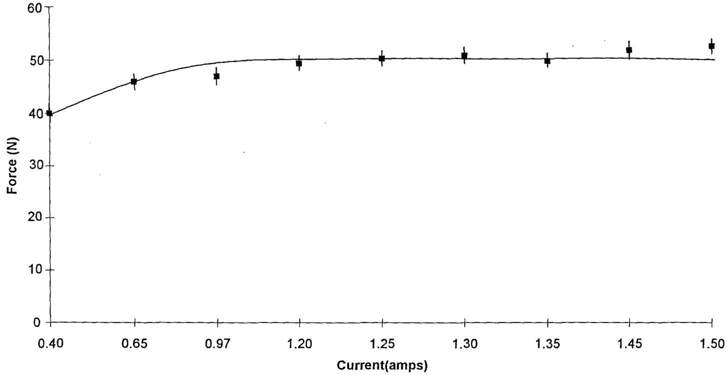
FIG 4.0 Shows the variaton in force with new solenoids
