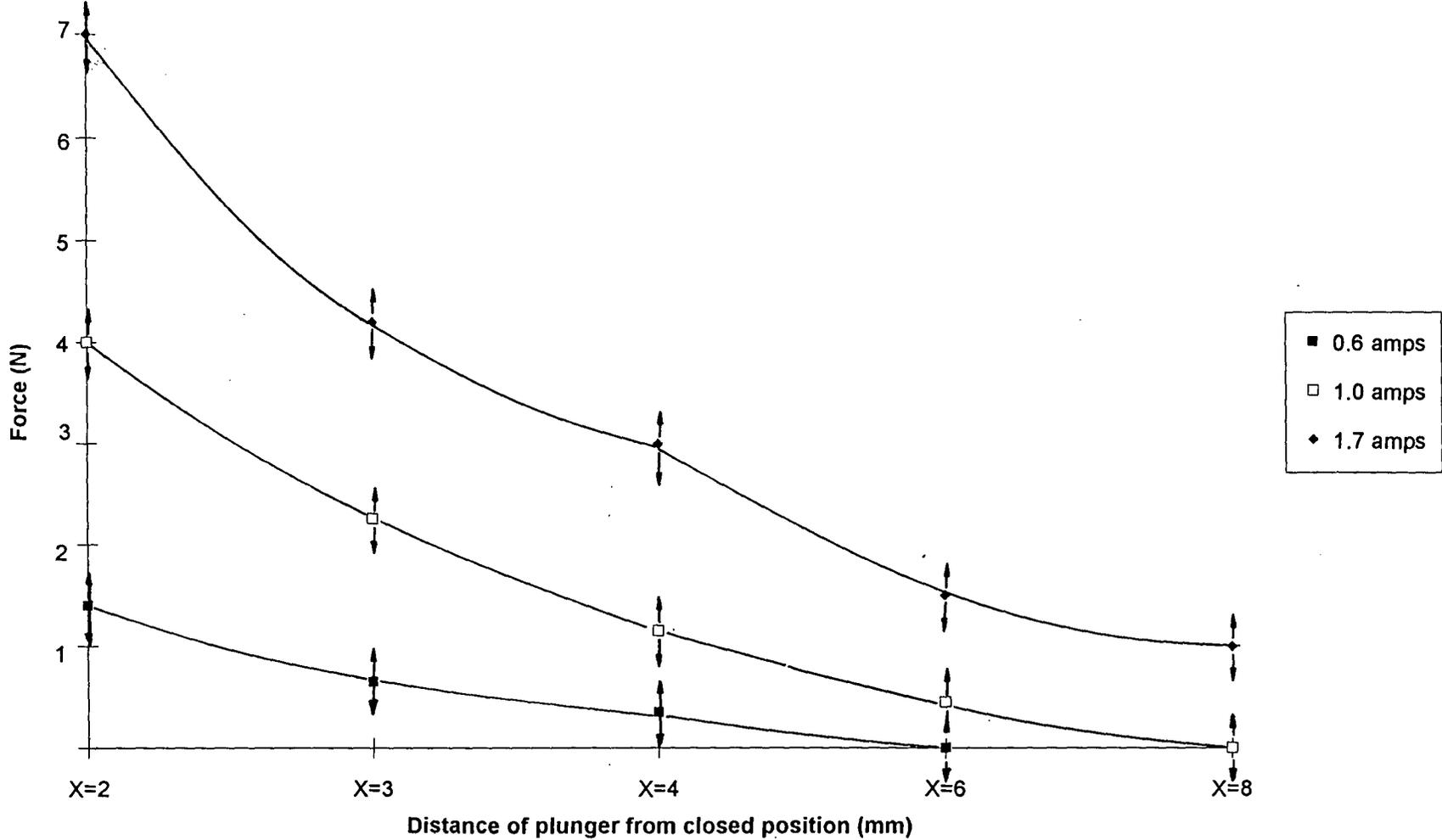
FIG 4.3 Shows force characteristics of modified solenoid
