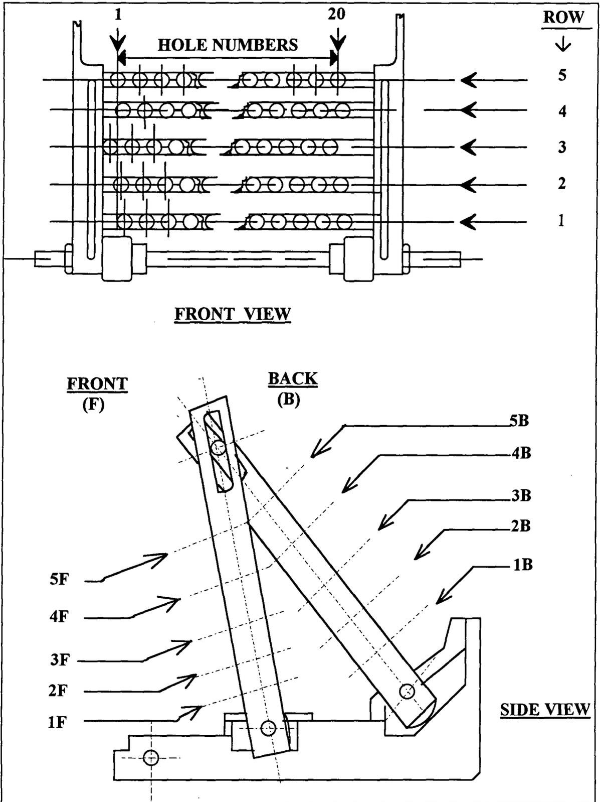
FIG A.8 Shows the identification of the backs of solenoids.
