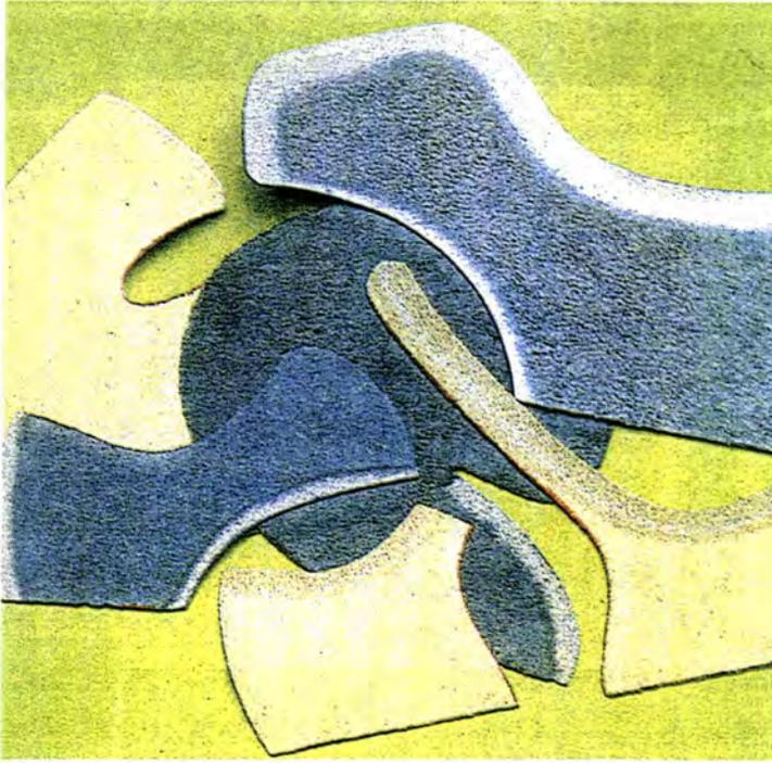
Fig 1.4 A typical example of skived components ( by permission BUSM Ltd ).
