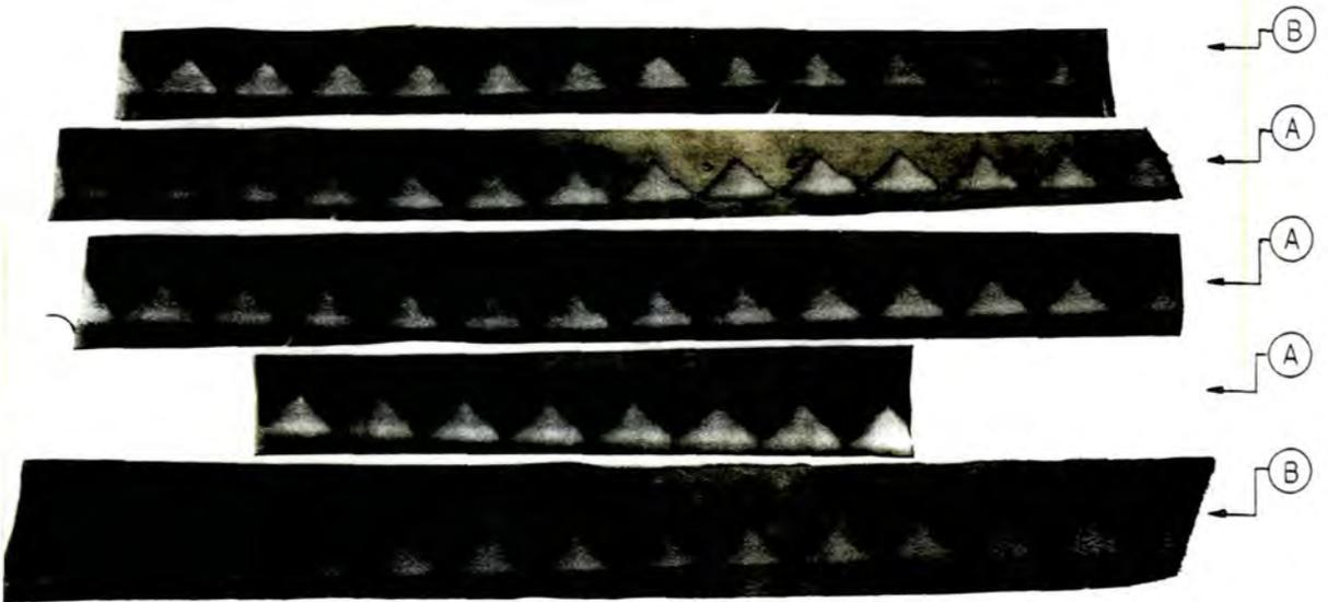
Figure 8.11 Shows the comparison of the skived strips of leather with the input voltages of 12v and 24v. The top photograph is a closer view and shows that the skives labelled A have been skived at 24v, whilst the skives labelled B have been skived at 12v.
