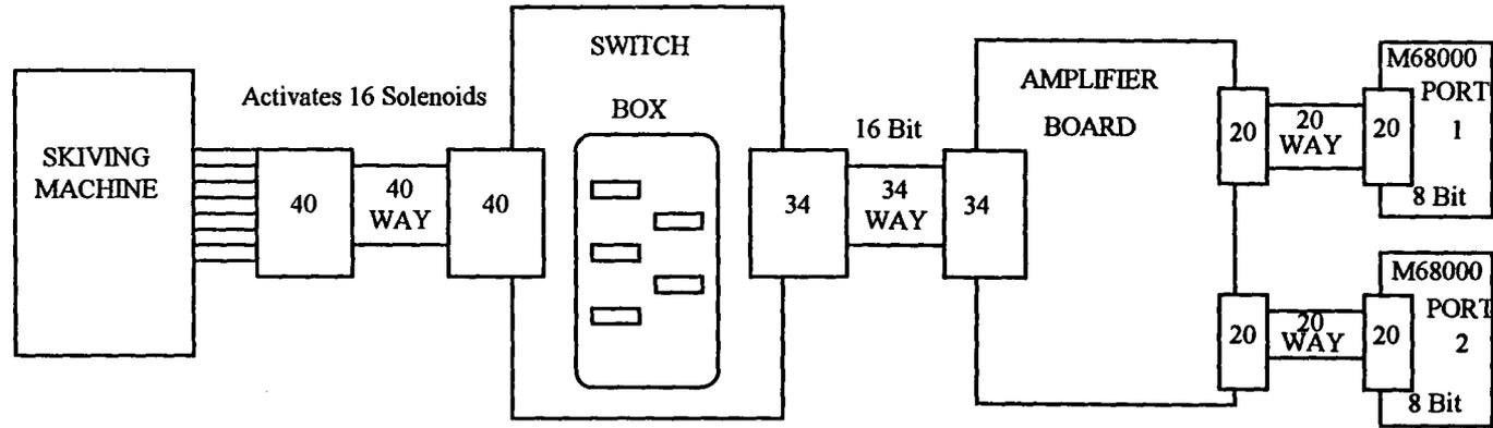
FIG 7.1 Shows the communication between the Motorola M68000 microprocessor and the new Skiving Machine.
