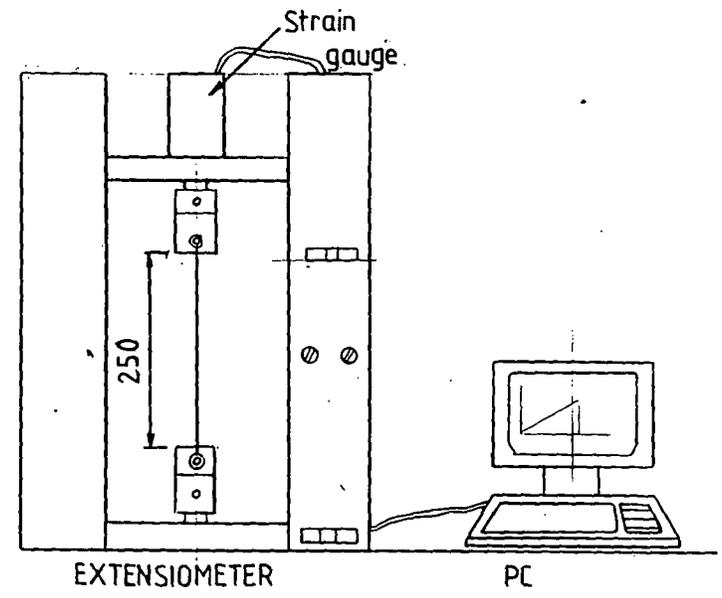
FIG 4.5 Shows method of connecting wire to extensometer
