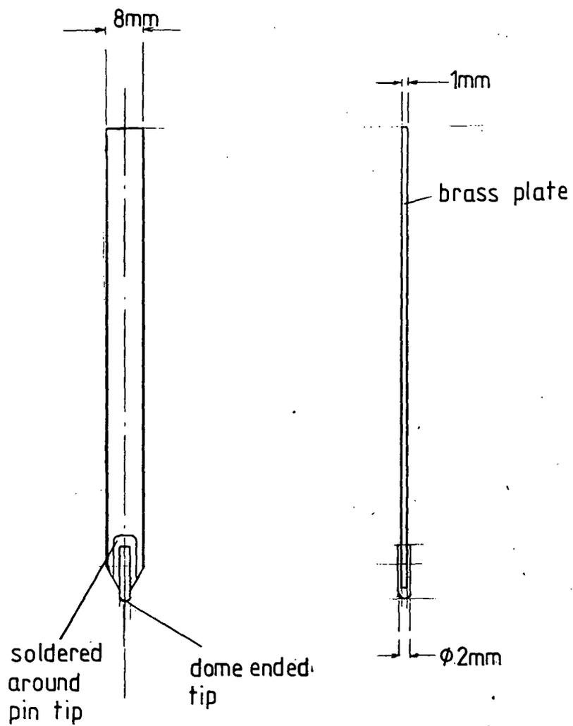
FIG 3.1 Shows experimental pin.
