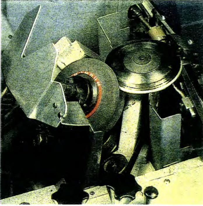
Fig. 1.2 The basic disk knife based mechanism, in all existing skiving machines
