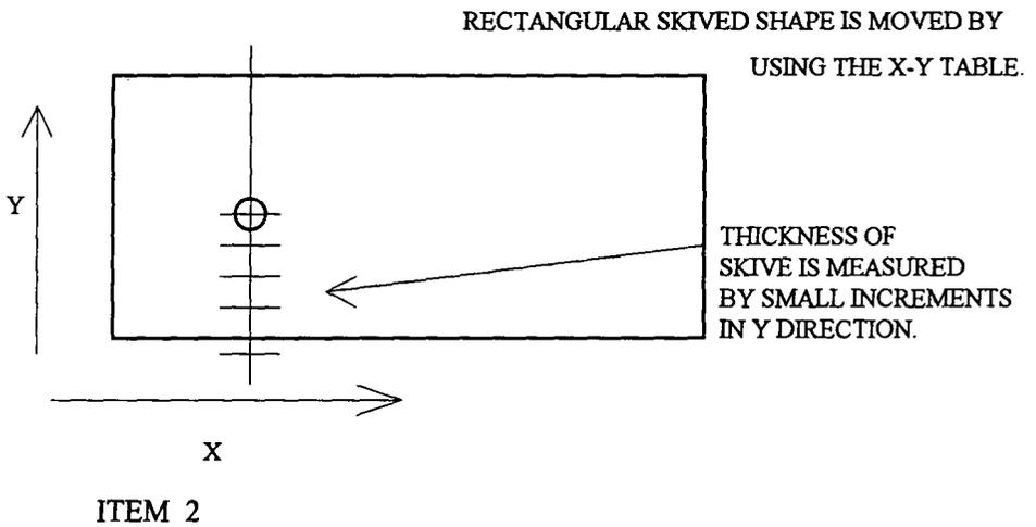
Figure 8.6 shows the equipment and method used to determine the depth of cut.
