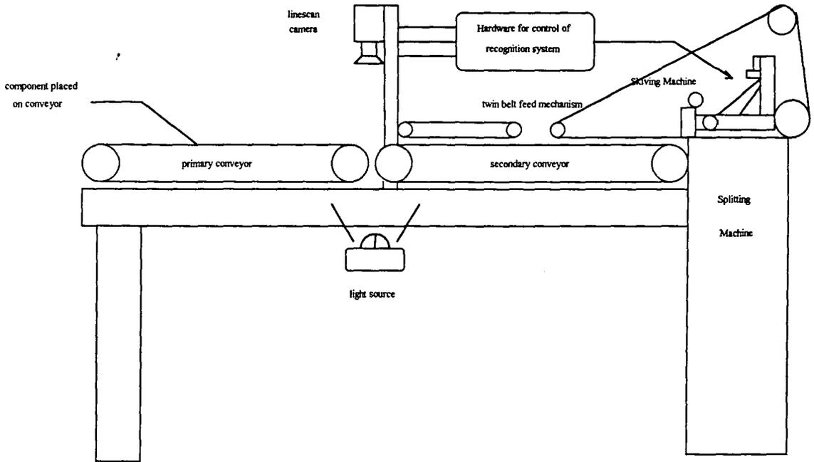
**Fig 1.6 Shows a schematic diagram of the automated skiving system.**
