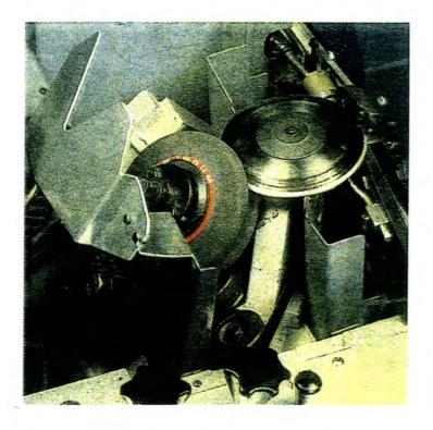
Fig. 1.2 The basic disk knife based mechanism, in all existing skiving machines (by permission BUSM Ltd).
