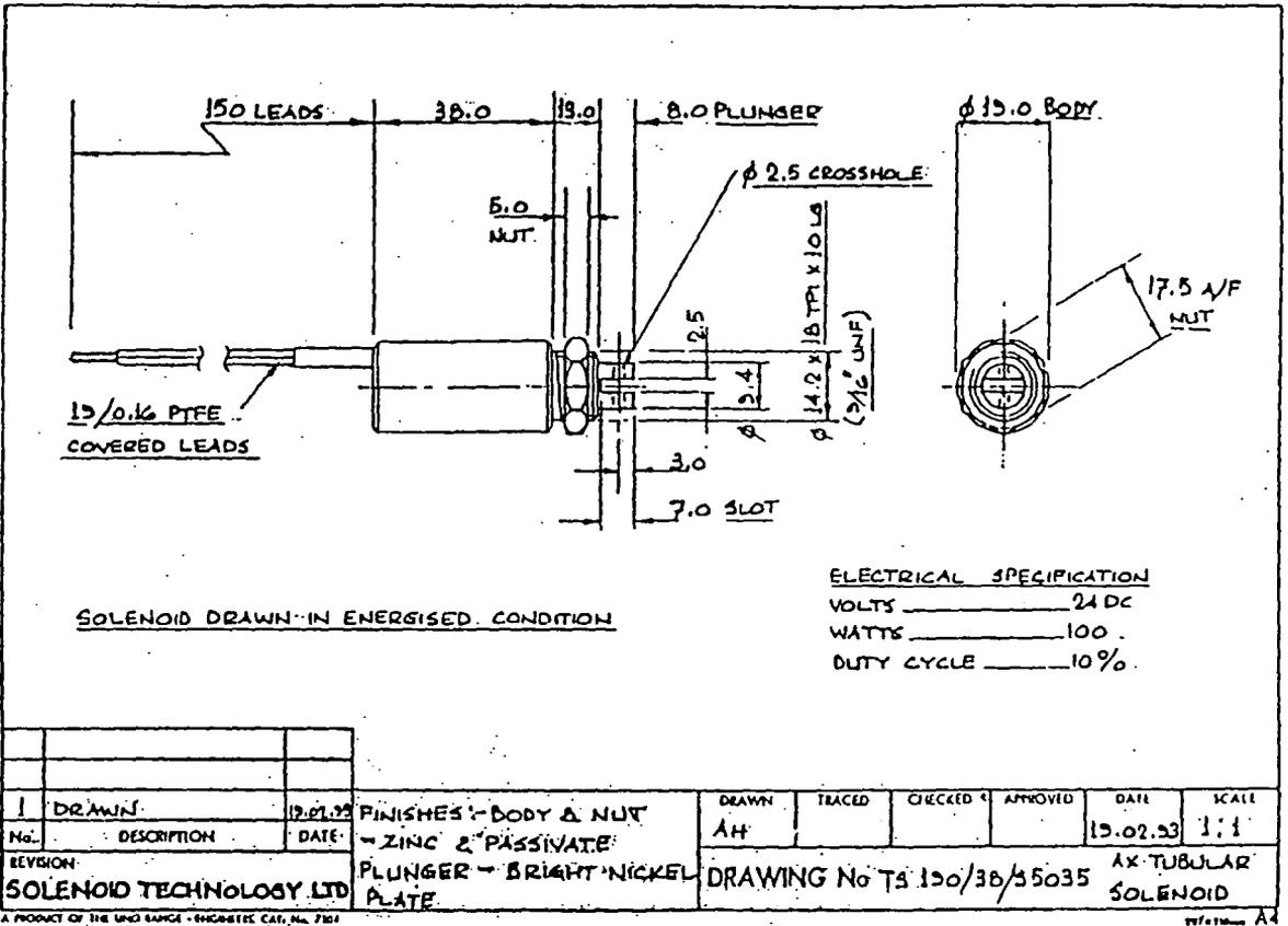
Fig. 3.5 Shows the details and dimension of the new solenoid
