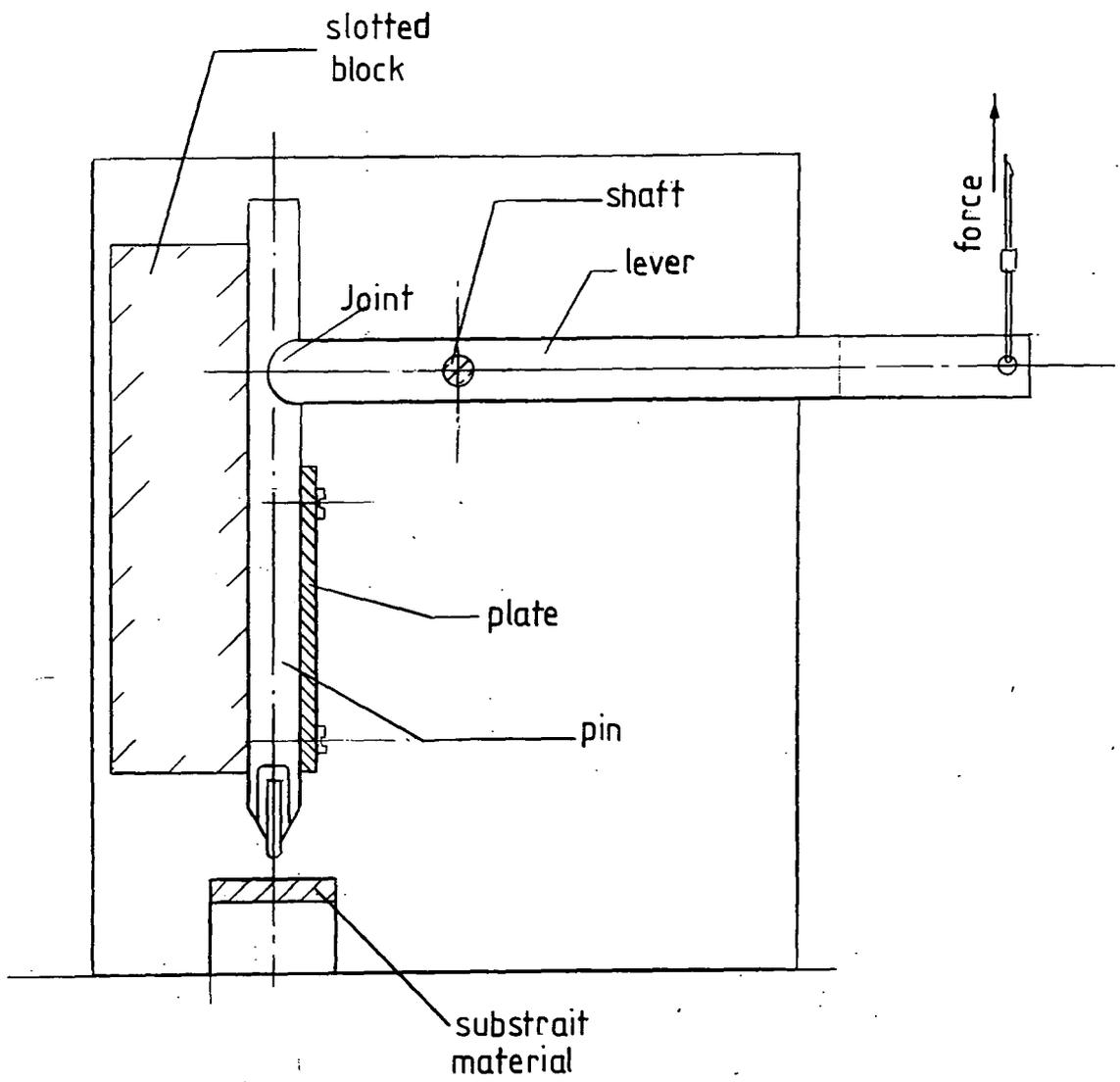
FIG3.2 Shows the lever and pin joint mechanism
