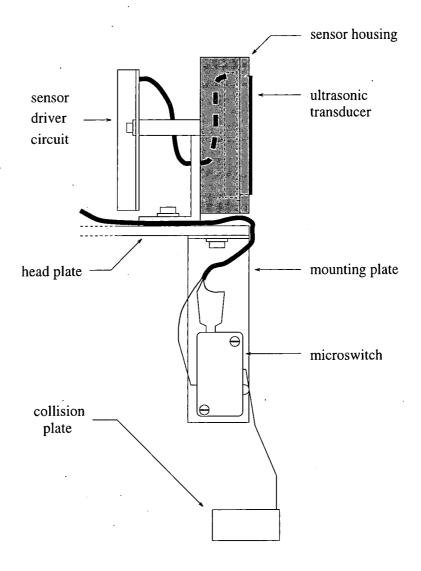
Figure 6.10: The ultrasonic sensor housing and collision detector
