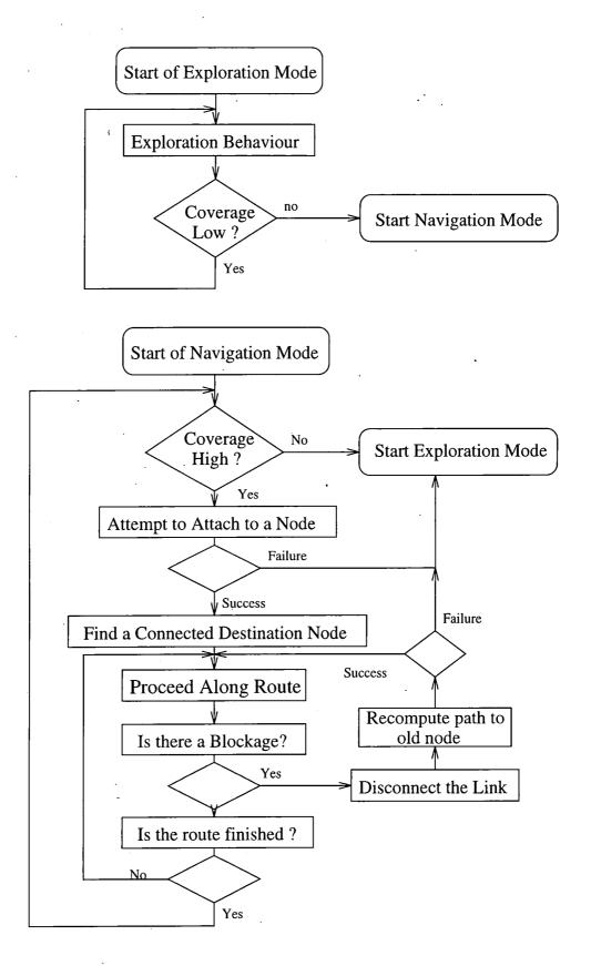
Figure 5.4: Flow diagrams for coverage control strategy
