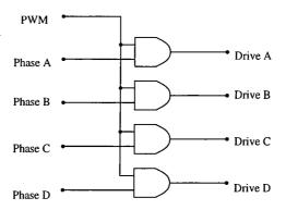
Figure 6.21: The logic interface
