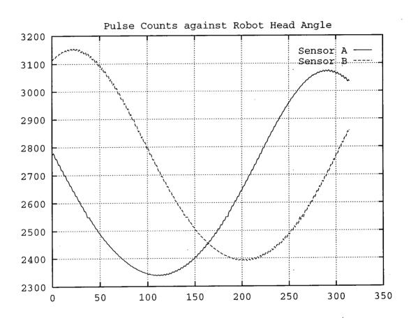
Figure 7.9: The output values from the two sensors A and B
