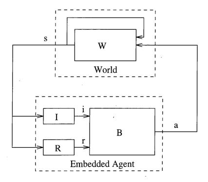
Figure 2.6: The reinforcement learning framework
