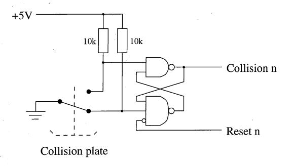
Figure 6.35: The collision detector diagram
