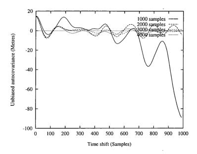
Figure 4.11: Variation of autocovariance for different path lengths
