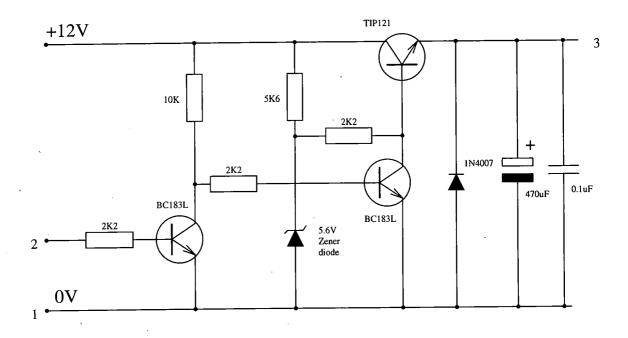
Figure C.7: The connectors for the ultrasonic sensor power supply
