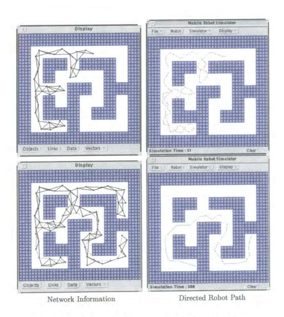
Figure 5.8: Path planning and corresponding robot motion in a maze
