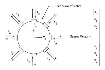
Figure 3.8: The robot's sensor vector
