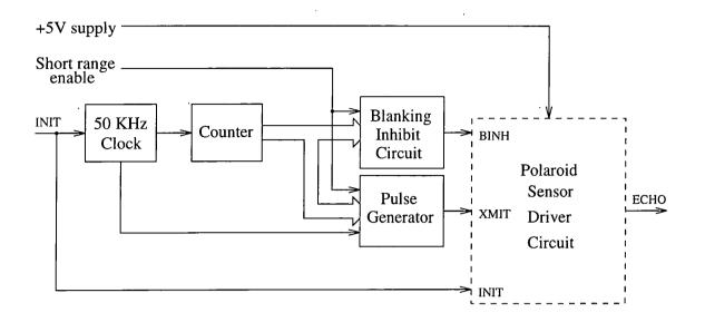
Figure 6.31: The sensor circuit
