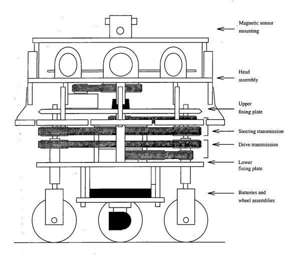
Figure 6.3: The robot chassis
