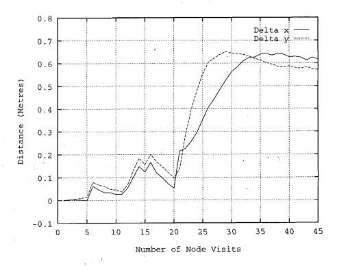
Figure 8.8: The positional correction required for both a translational and a positional disturbance
