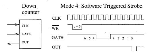
Figure 6.27: The down counter's operation in mode 4
