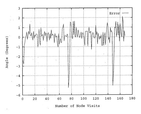
Figure 8.31: Estimated angular error during navigation with correction
