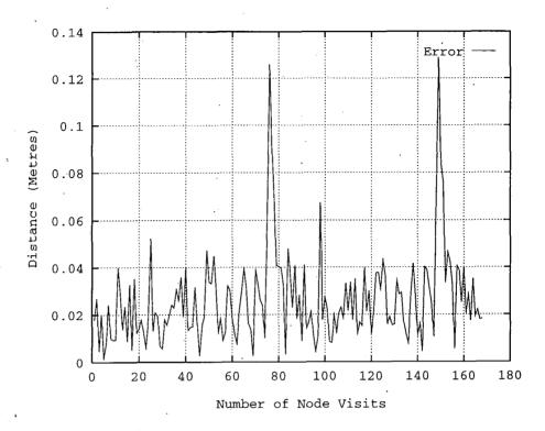
Figure 8.30: Estimated positional error during navigation with correction
