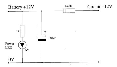
Figure C.8: The connector for the battery supply and fuse protection circuit
