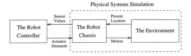
Figure 3.7: The main simulation elements
