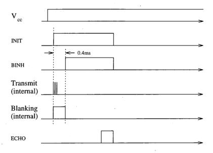
Figure 6.30: The Polaroid short range operating cycle
