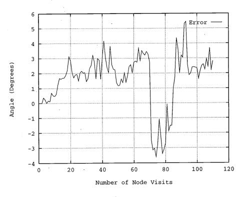
Figure 8.29: Estimated angular error during navigation without correction
