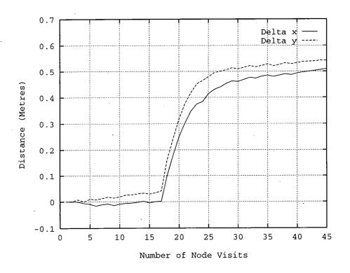
Figure 8.4: The position correction required with a translational disturbance
