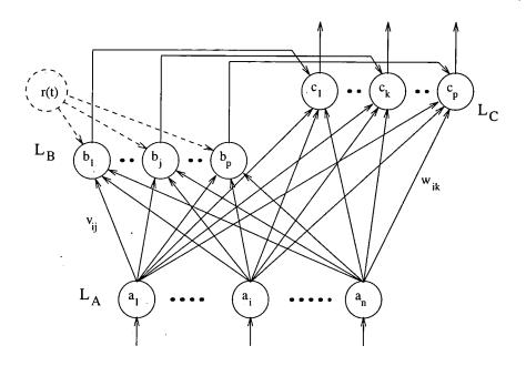
Figure 2.7: The adaptive heuristic critic
