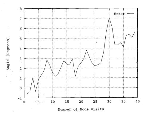
Figure 8.16: Estimated angular error during navigation without correction
