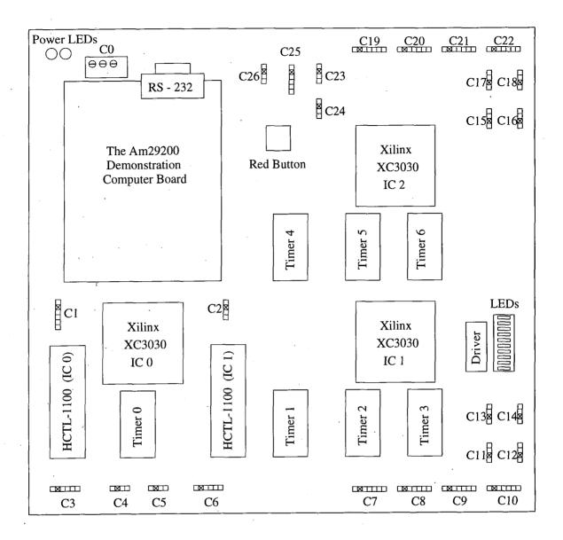
Figure C.1: The control circuit board layout
