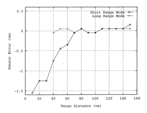
Figure 7.6: The sensor error recorded as a function of distance measured
