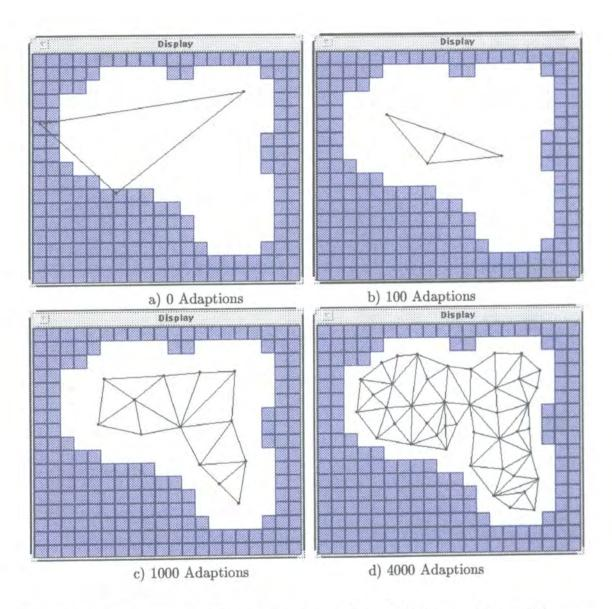
Figure 4.4: Development of a 2D growing cell network to a 2D data set. The model parameters were  $\lambda=100, \epsilon_b=0.06, \epsilon_n=0.002, \alpha=0.05$
