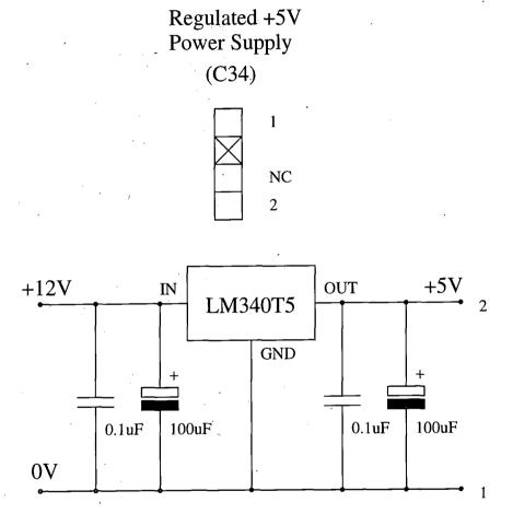
Figure C.6: The connectors for the regulated power supply
