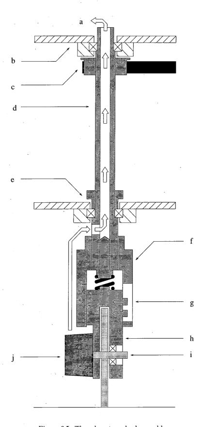
Figure 6.5: The odometry wheel assembly
