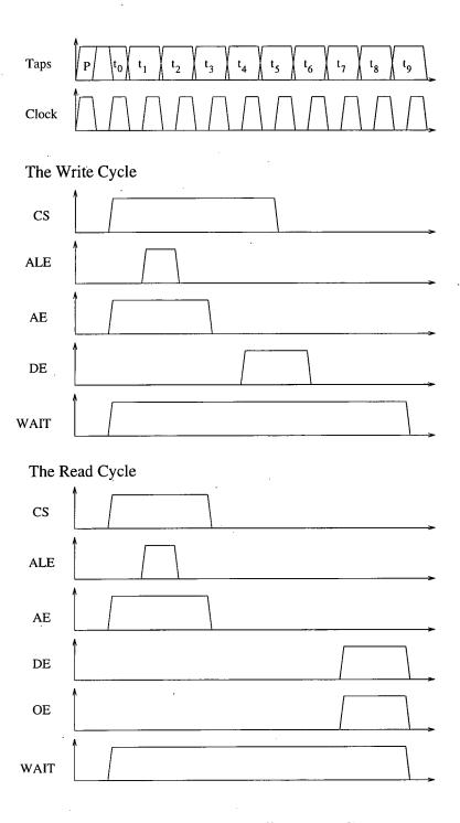
Figure 6.16: The motor controller timing diagram
