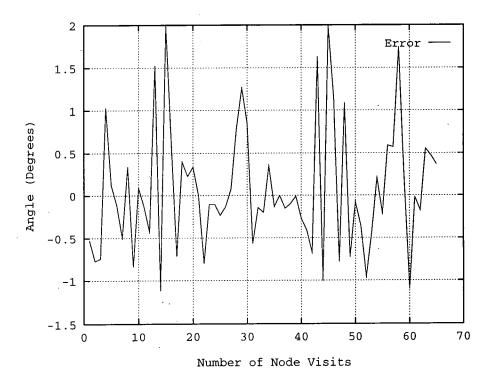
Figure 8.25: Estimated angular error during navigation with correction
