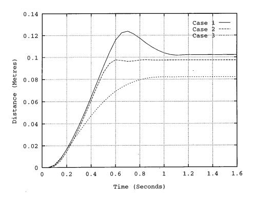
Figure 7.2: The robot's step response at different gain values
