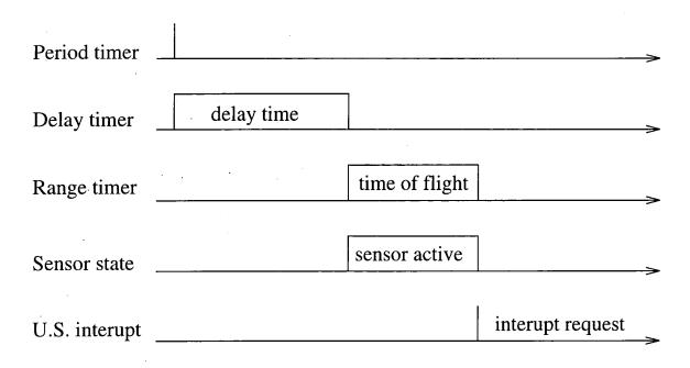
Figure 6.25: The ultrasonic sensor timing diagram
