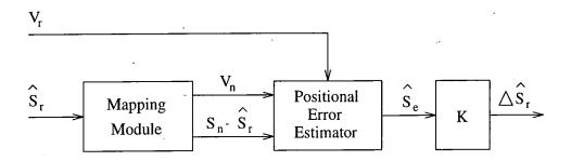
Figure 8.1: The correction mechanism for odometric drift
