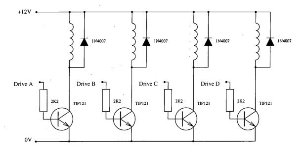
Figure 6.22: The stepper motor circuit diagram
