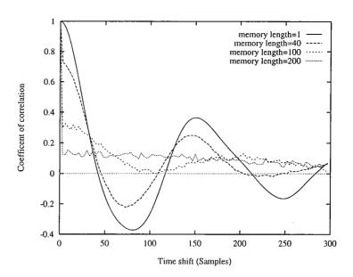
Figure 4.17: Output correlations for different sized memory banks
