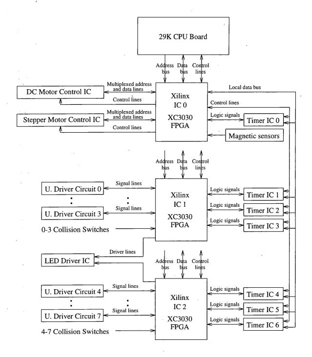
Figure 6.12: The system's logic layout
