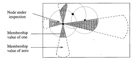
Figure 5.2: Calculation of coverage from sensor range measures
