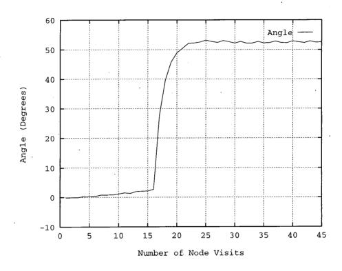
Figure 8.5: The angular correction required with a rotational disturbance
