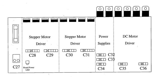
Figure C.3: The power and drive circuit board
