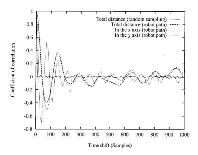
Figure 4.12: Comparison of correlation of x,y and total distance measures
