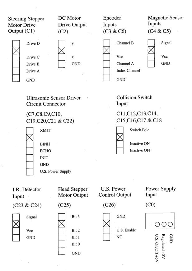
Figure C.2: The control circuit connectors diagram
