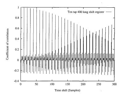
Figure 4.15: Output correlation from a ten tap shift register
