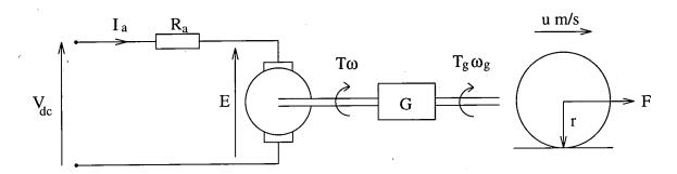
Figure A.1: The circuit diagram for the motor and load
