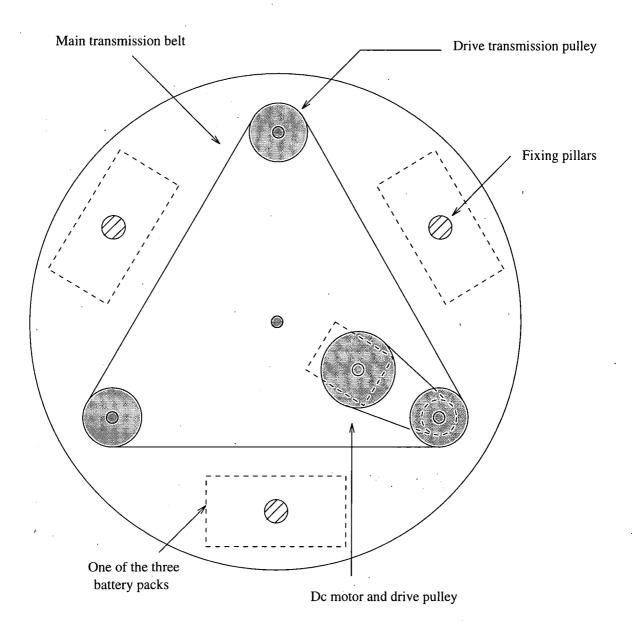
Figure 6.6: The drive transmission
