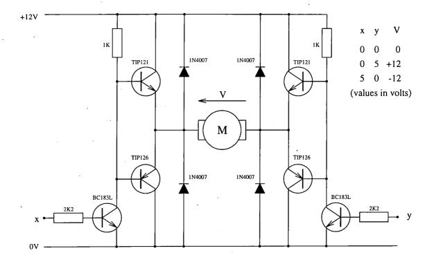
Figure 6.19: The 'H' bridge power amplifier
