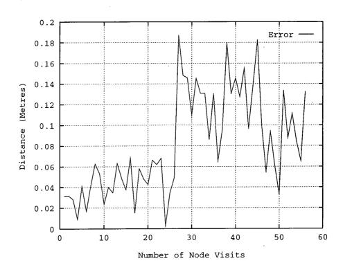
Figure 8.22: Estimated positional error during navigation without correction
