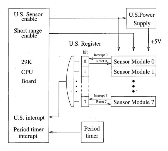
Figure 6.26: The schematic diagram of the sensor system
