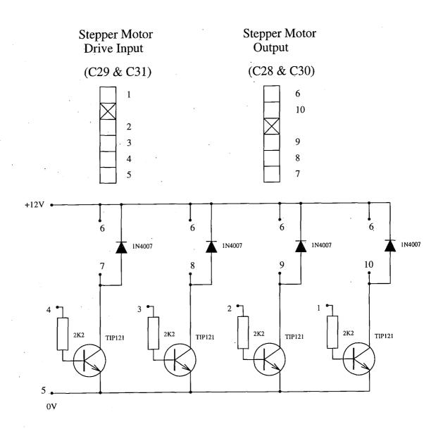
Figure C.5: The connectors for the stepper motor driver circuit
