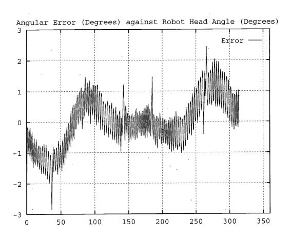
Figure 7.11: The error in the magnetic field sensor system
