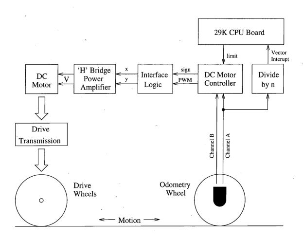
Figure 6.17: The motor controller feedback loop
