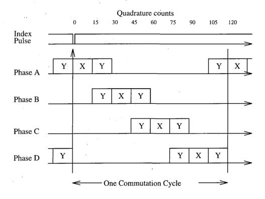
Figure 6.20: The stepper motor commutation cycle
