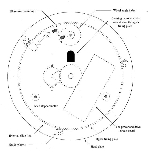
Figure 6.8: The mounting for the head assembly
