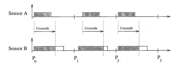
Figure 6.23: The error eliminating rapid ultrasonic firing scheme
