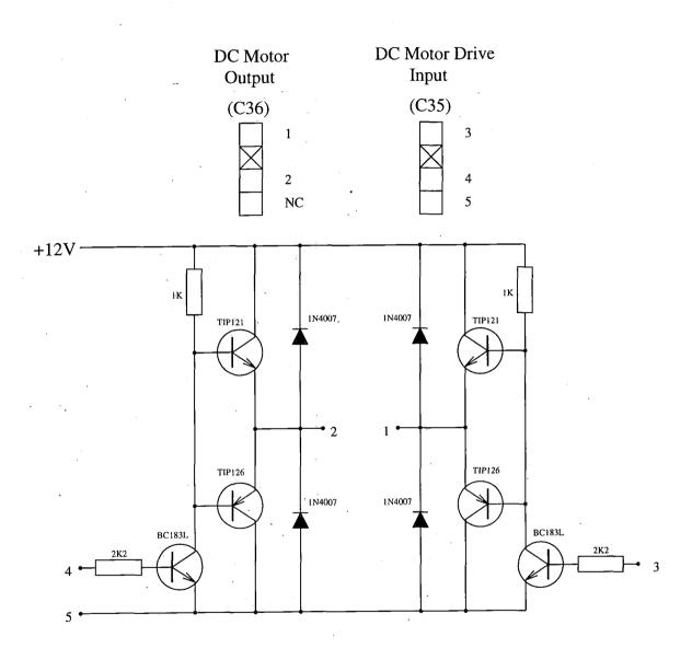
Figure C.4: The connectors for the DC motor driver circuit
