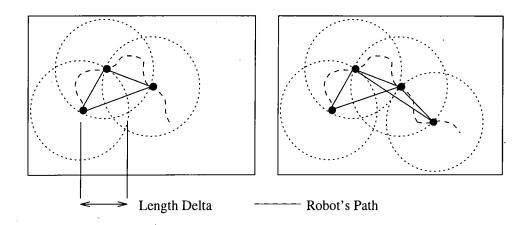
Figure 5.1: The creation of a new node in the network
