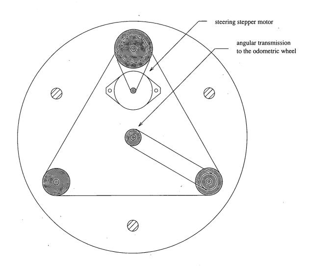
Figure 6.7: The steering transmission
