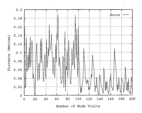
Figure 8.10: Estimated positional error during navigation of a rectangular environment
