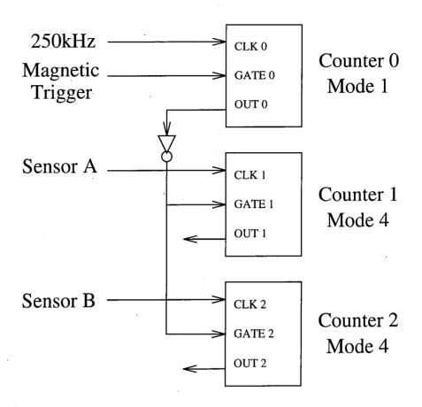
Figure 6.33: The magnetic sensor schematic
