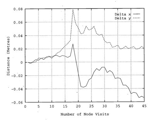
Figure 8.6: The positional correction required with a rotational disturbance
