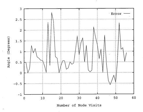
Figure 8.23: Estimated angular error during navigation without correction
