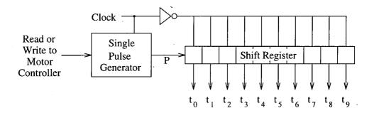
Figure 6.15: The motor controller pulse generator
