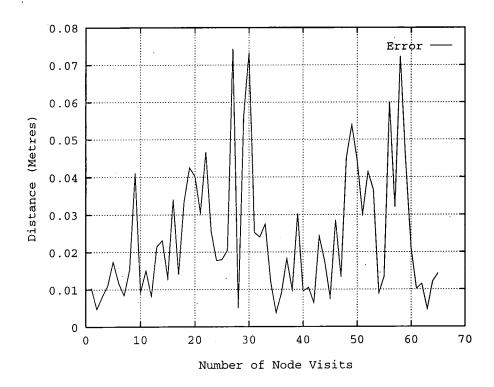
Figure 8.24: Estimated positional error during navigation with correction
