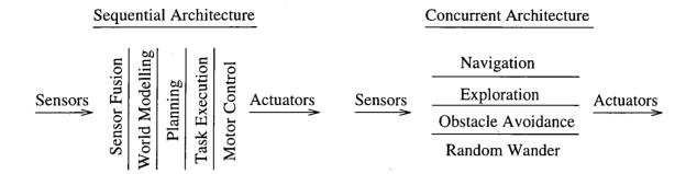
Figure 3.9: Sequential and concurrent architectures
