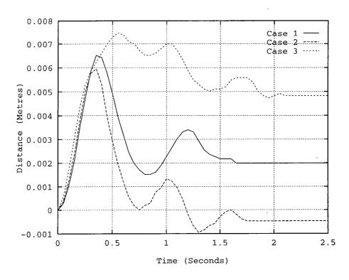
Figure 7.3: Displacement of the drive system for different controllers
