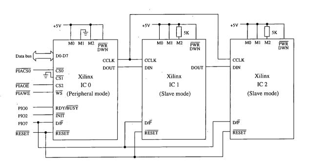
Figure D.1: Programming the FPGAs
