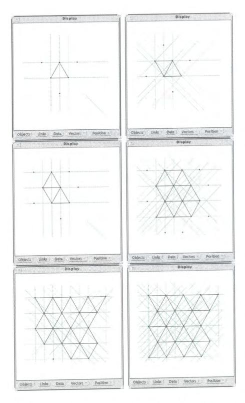
Figure 8.21: Robot mapping using the exhaustive mesh search algorithm
