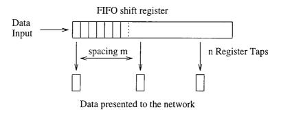
Figure 4.13: Shift register used for de-correlating incoming data
