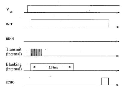
Figure 6.29: The Polariod sensor operating cycle
