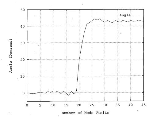
Figure 8.7: The angular correction required for both a translational and a rotational disturbance
