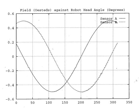
Figure 7.10: The calibrated field values from the two sensors A and B
