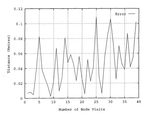
Figure 8.15: Estimated positional error during navigation without correction
