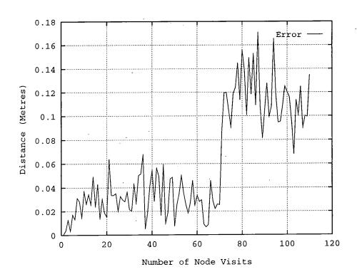
Figure 8.28: Estimated positional error during navigation without correction
