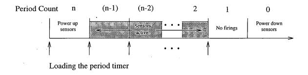
Figure 6.24: The sensor firing period timing diagram
