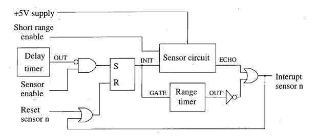
Figure 6.28: The schematic diagram of the sensor module
