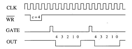
Figure 6.32: The down counter's operational mode 1
