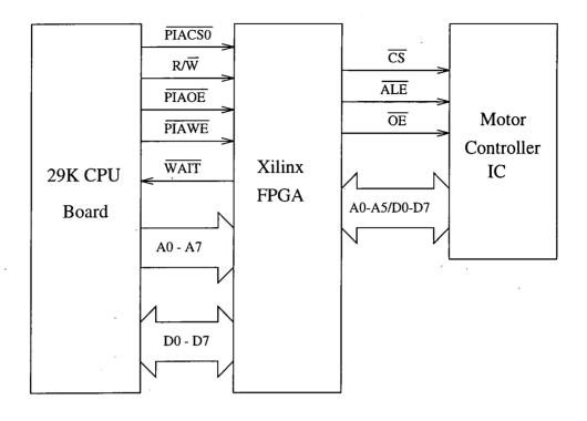
Figure 6.14: The motor controller interface
