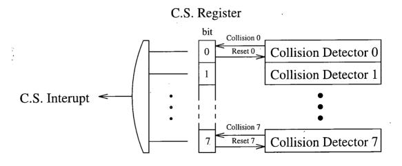
Figure 6.34: The schematic diagram of the collision system
