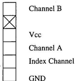
**Magnetic Sensor Inputs (C4 & C5)**
