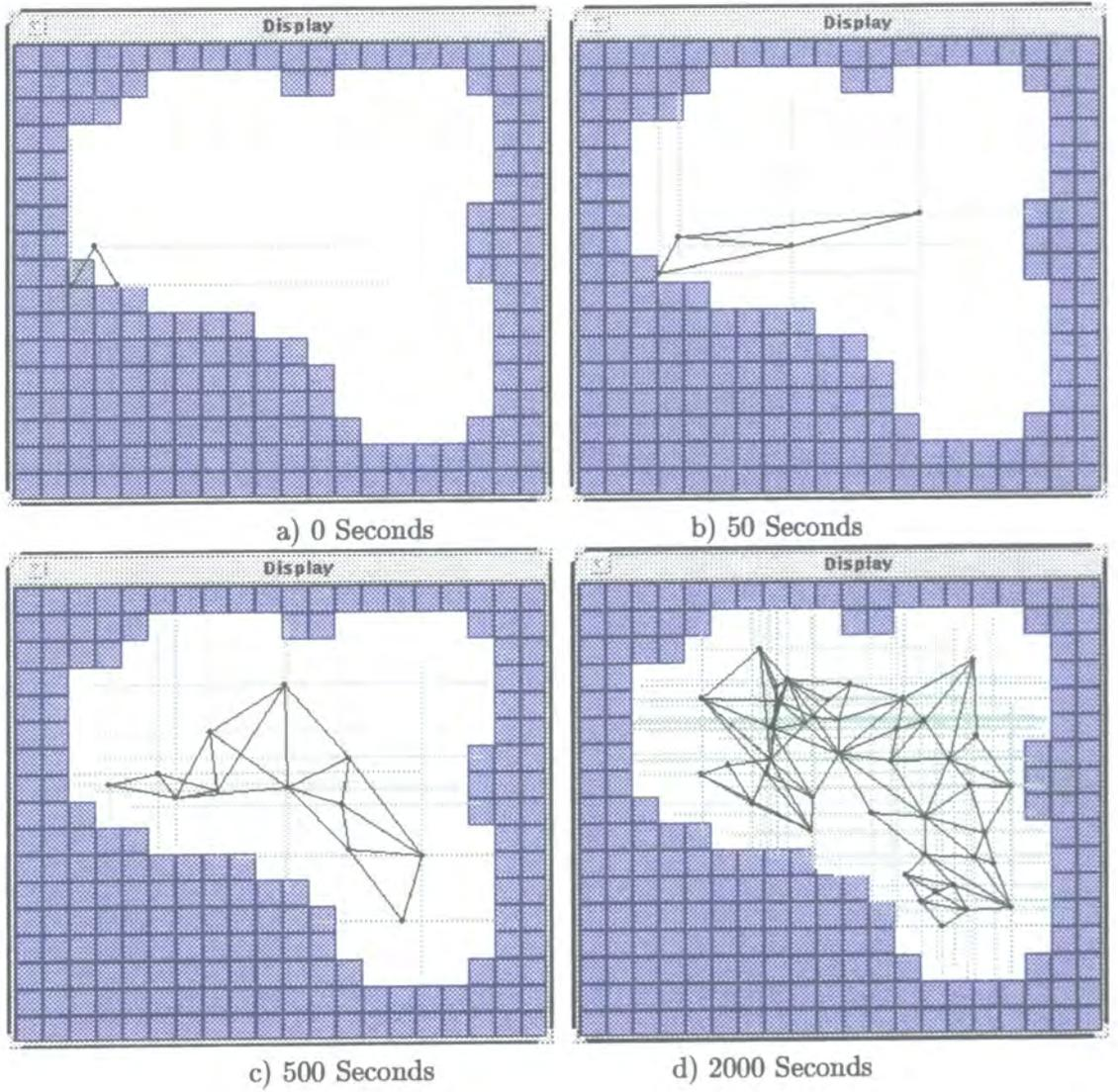
Figure 4.6: Development of the GCS during exploration of the environment. The model parameters were  $\lambda = 100$ ,  $\epsilon_b = 0.06$ ,  $\epsilon_n = 0.002$ ,  $\alpha = 0.05$
