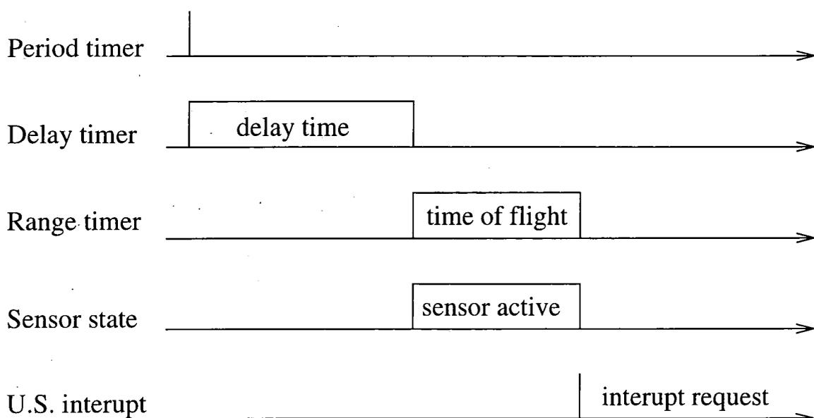
Figure 6.25: The ultrasonic sensor timing diagram
