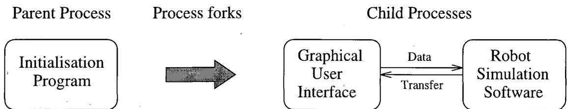
Figure 3.1: Initial set-up of the main simulation software
