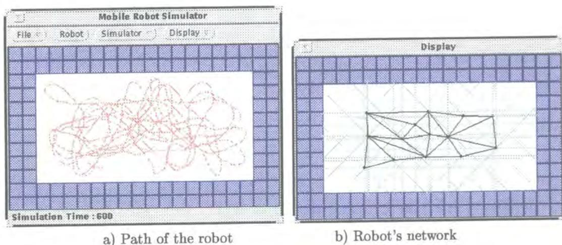
Figure 4.5: Network growth of a mobile robot using simple GCS
