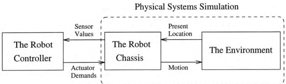
Figure 3.7: The main simulation elements
