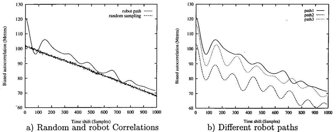
Figure 4.9: Comparison of unbiased autocorrelation function for data sequences
