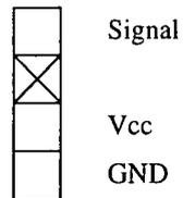
**Ultrasonic Sensor Driver Circuit Connector**
