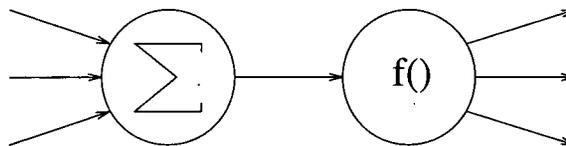
Figure 2.1: A single processing element
