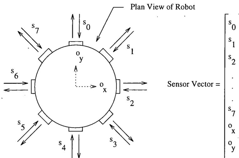
Figure 3.8: The robot's sensor vector
