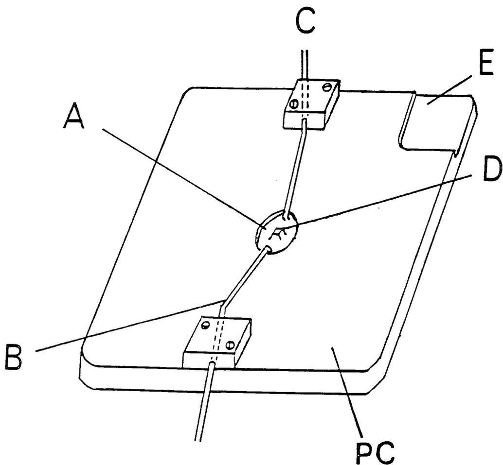
**Fig. 2.6. Superfusion bottle used to supply saline to the experimental chamber**
