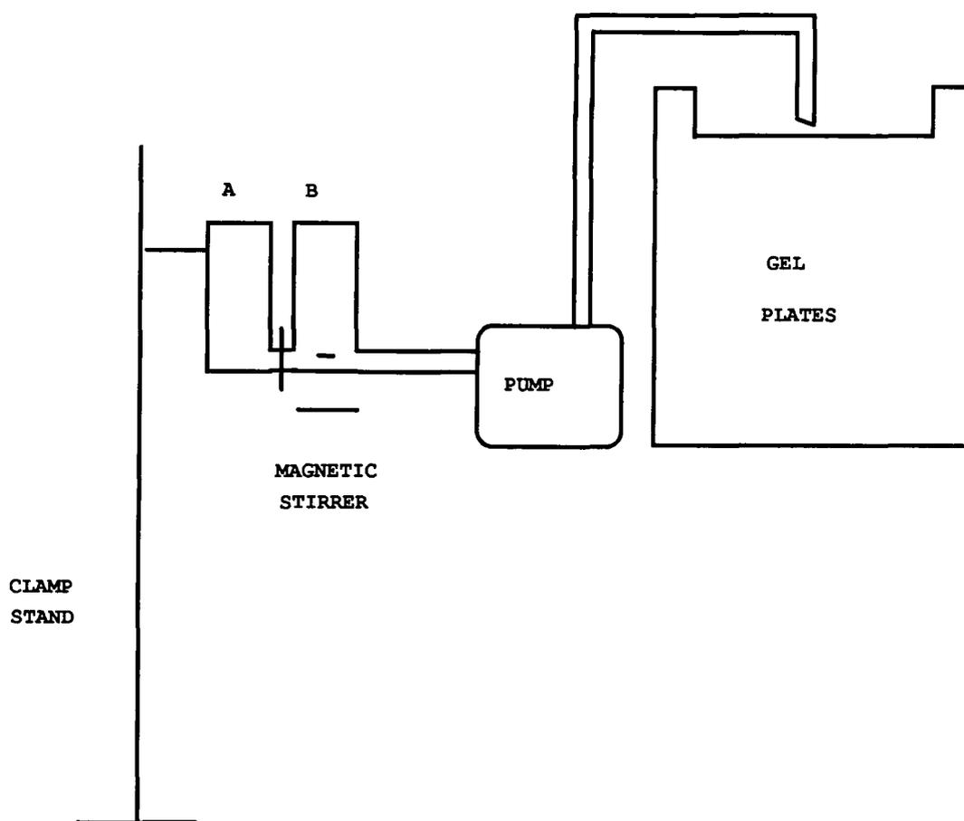
A was the reservoir of the gradient maker and B was the mixing chamber which contained a magnetic flea. B was suspended above a magnetic stirrer by a clamp. A clip isolated the two chambers (A and B). Tubing which connected the gradient maker to the peristaltic pump and glass gel plates was silicon tubing (1.6mm, inner diameter). The end of this tubing was cut at a  $45^\circ$  angle and held at the centre of the rear gel plate with the cut edge facing this plate.
