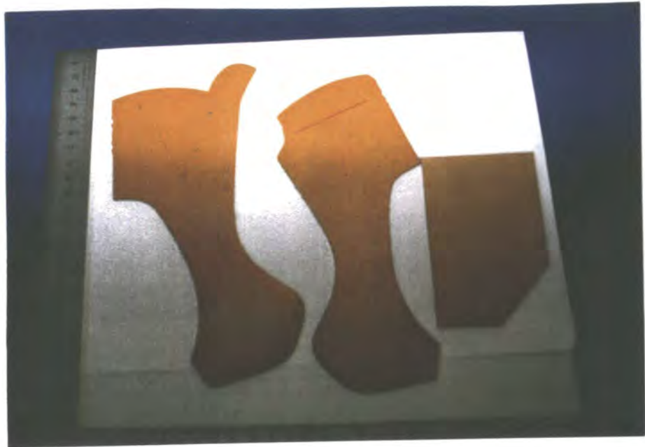
Figure 5.11 Typical components used to manufacture shoes
