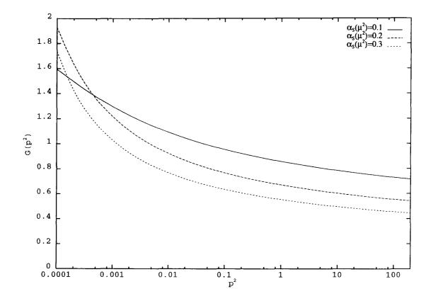
Figure 5.4: The gluon renormalisation function  $G(p^2)$  as a function of  $p^2$  with the infrared cutoff  $\lambda^2 = 10^{-4} \text{ GeV}^2$ .
