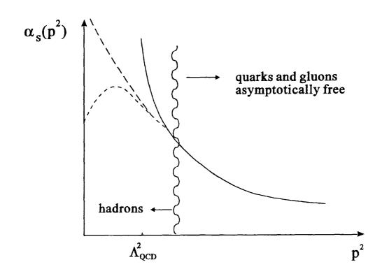
Figure 2.4: The running coupling  $\alpha_s$ . Here the solid line represents the perturbative result, and the dashed lines indicate that we do not know for certain what the behaviour of the coupling is at low momenta where perturbation theory is inapplicable.
