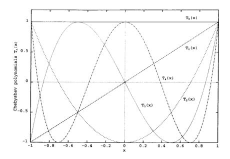
Figure 5.3: Chebyshev polynomial  $T_0(x)$  through  $T_4(x)$
