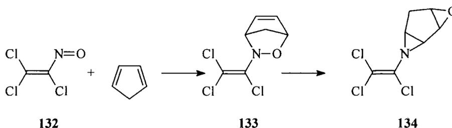
**Scheme 1.42:** [4+2] Cycloaddition of a Nitroso-Alkene with a Cyclic Diene
