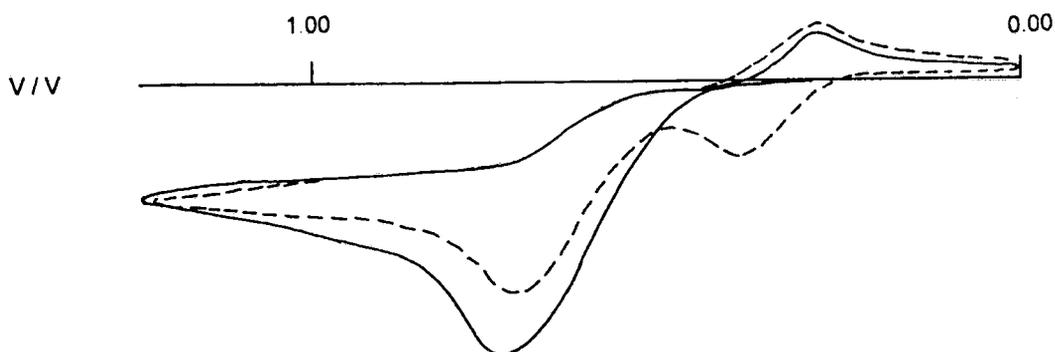
**Figure 2.9:** Cyclic Voltammogram for compound **188a** in Acetonitrile at 20°C with Tetrabutylammonium Hexafluorophosphate as Electrolyte.
