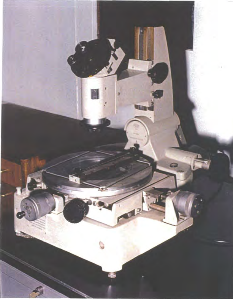
Figure 5.3 Carlzeiss Jena 10907 microscope used for measuring the flank wear
