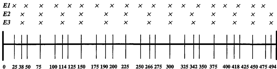
Figure 9.10 Machine stoppages for edge changing and the accumulated number of parts.
