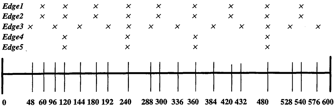
Figure 9.4 Machine stoppages for edge changing and the accumulated number of parts when the second strategy is employed.
