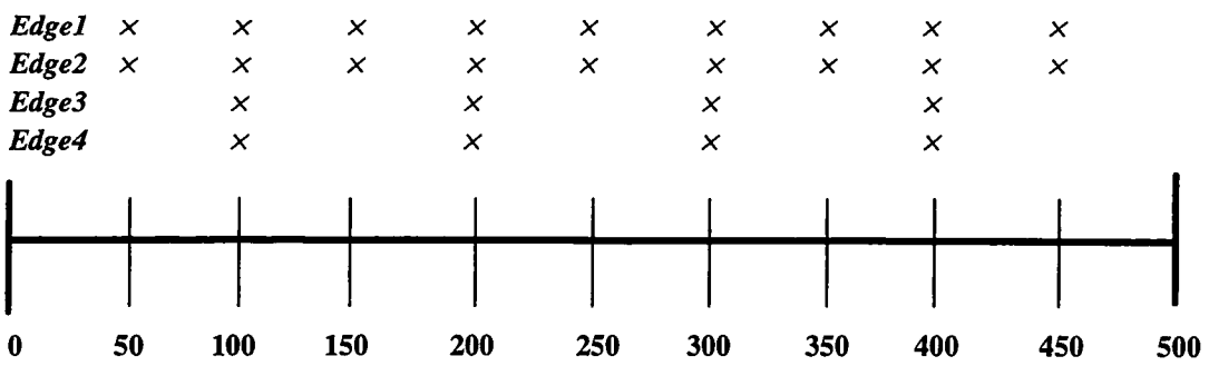
Figure 9.7 Machine stoppages for edge changing and the accumulated number of parts.
