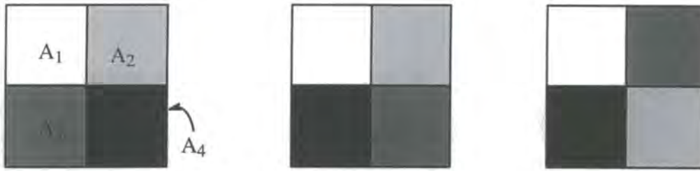
Figure 4.2: The three canonical positions for the brightness level of the quadrants of a square sub-image [21]
