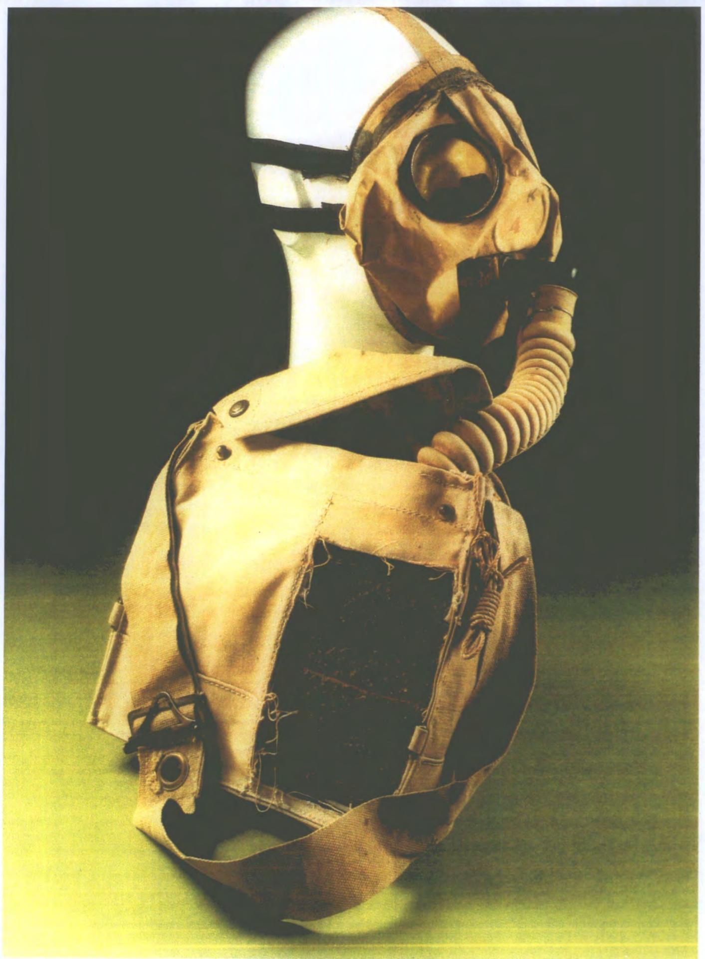
Figure 1.2.2. Muslin mask with a carbon box filter.
