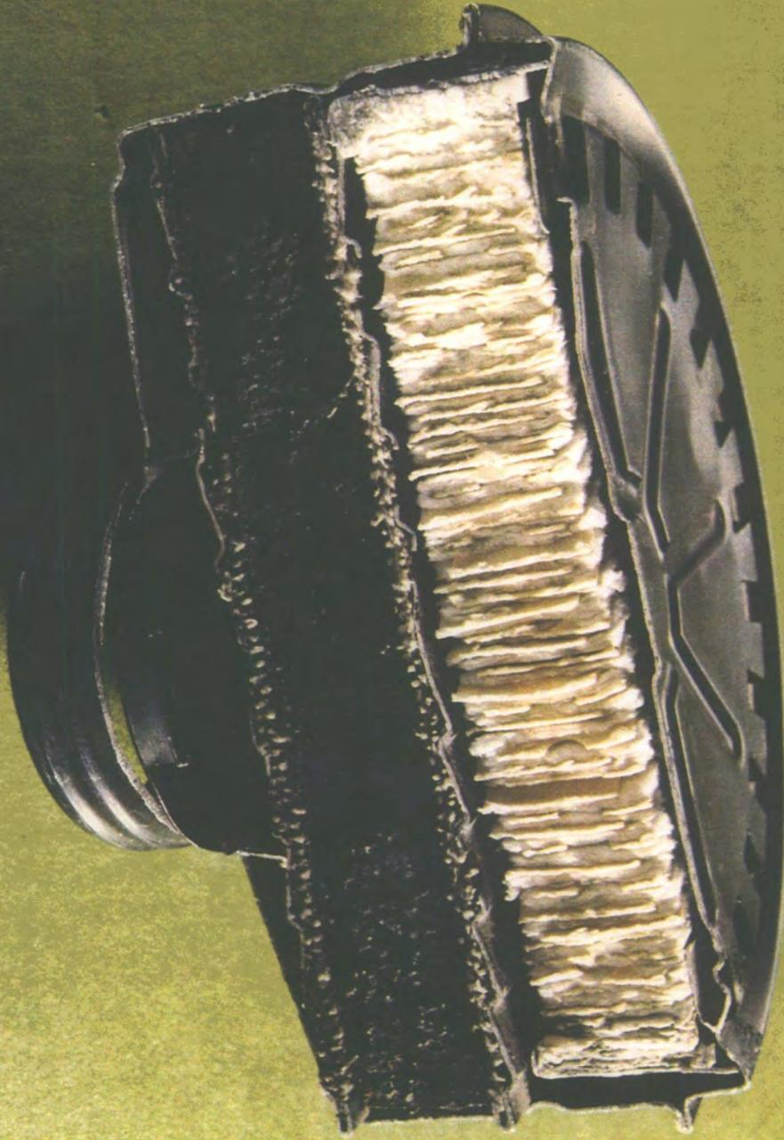
Figure 1.2.6. A section through a filter canister.
